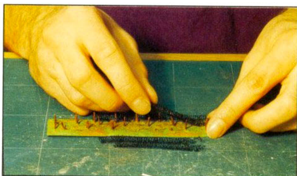
Attaching the coiled mesh to the support
