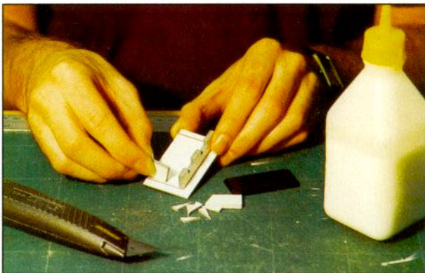
Gluing the walls to the base
