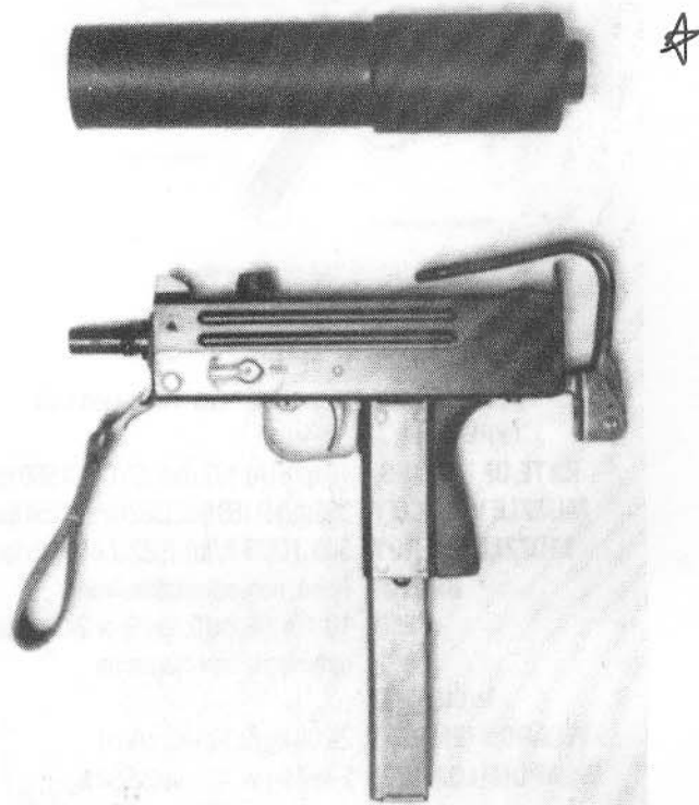
Ingram M11 with MAC suppressor separate and 32 rd magazine
