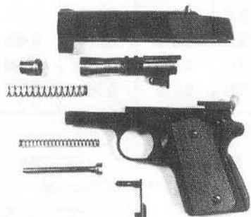
A field stripped Detonics Combat Master
