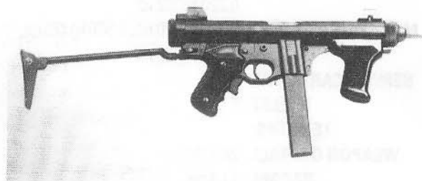
PM-12S with stock extended and bolt forward
