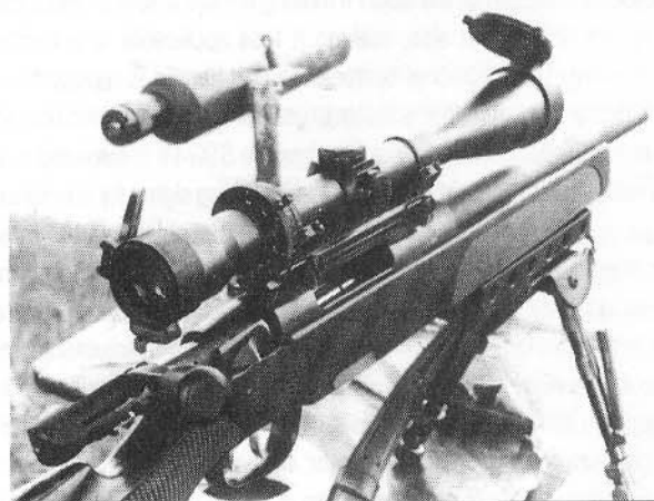
Steyr SSG PII showing the ART IV telescopic sight and its controls
