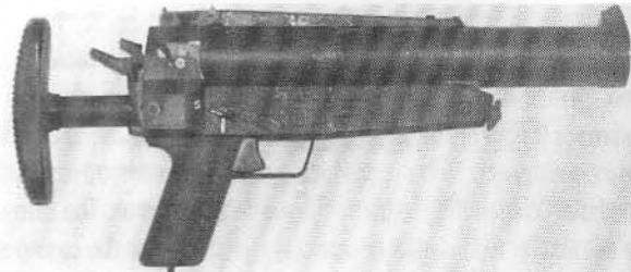
Granatepistole with stock collapsed and sight folded
