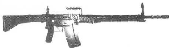
Stg 57, Swiss military issue version of the 510-4 except for being chambered for 7.5 Swiss and having a 24 round magazine, the Stg 57 is identical to the 510-4
