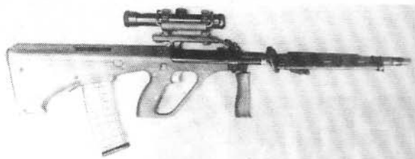
AUG LSW (HBAR-T) with bipod folded and 42 rd magazine
