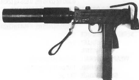
Ingram M11 with MAC suppressor mounted and 32 rd magazine, selector set to full automatic and bolt in forward position
