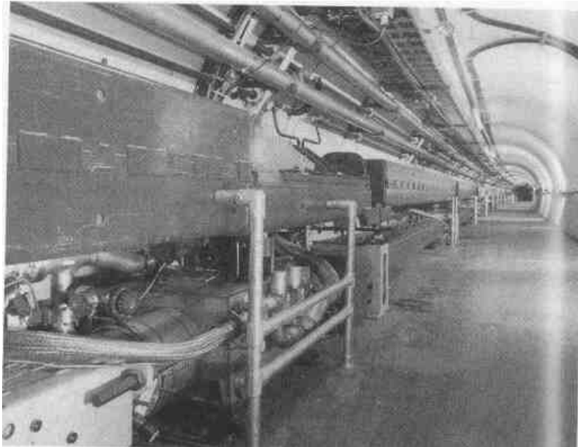
John Peoples, director of Fermilab, shown with the antiproton source which he designed. The antiprotons produced by collisions of protons on a lithium target are stored in a circular beam using the array of magnets shown in the photograph. ( Fermilab Photo )
