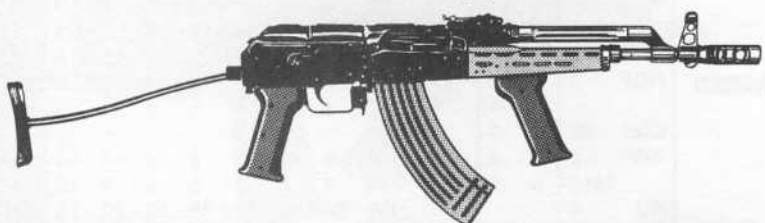
Hungarian modified AKM 63 with folding stock and foregrip.
