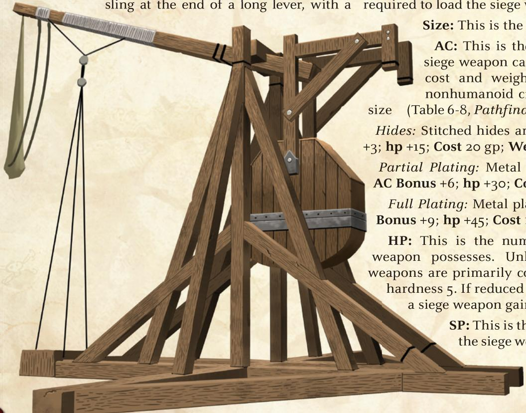
counterweight (often with crew or animals pulling attached ropes) close to the fulcrum. The leverage imparted by a trebuchet allows it to hurl massive missiles. Trebuchets are too bulky to move and must be assembled on the battlefield. Trebuchets have a minimum range of 150 feet. Trebuchets are indirect fire weapons.
