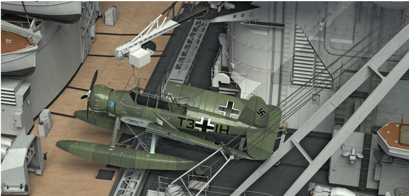
An alternative way to transfer the floatplane from the hangar to the catapult – by means of an overhead crane.
