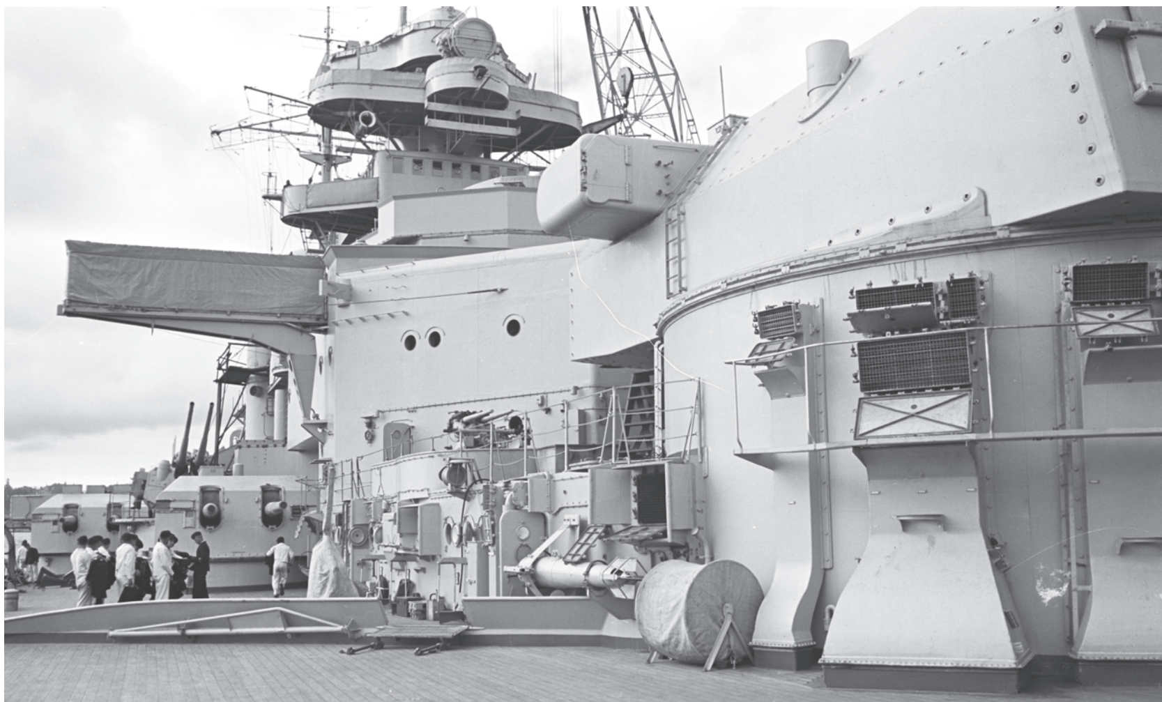
Blohm & Voss shipyard, Hamburg, summer 1940. Photo taken from the upper deck to the right side of main artillery turret 'Bruno', looking aft. The vents at the barbette in the foreground would later be modified so that they wouldn't get flooded with seawater and spray. The rear breakwater to the left has a hinged passage. A small crane arm, part of the paravane gear, is fitted against the breakwater's fore surface. (Bundesarchiv, Bild 193-05-3-39)
