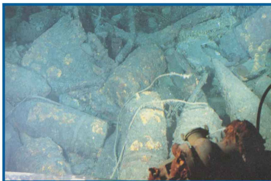
46cm AP shells in the broken lower part of gun turret
