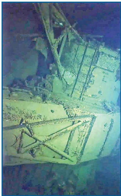
The 'Hoiban' tower with the small rear mast and the aft wall of the 15.5m rangefinder with strengthening framework
