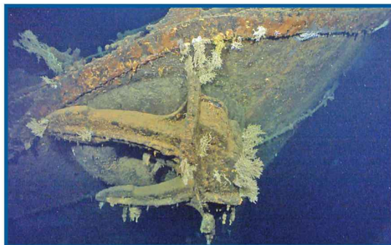
Starboard 15-ton anchor, the port anchor was dropped into the sea about two hours before her sinking, to attempt to reduce the list.
