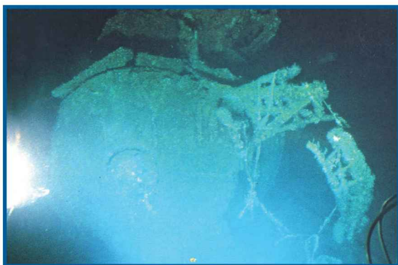
View of the 'Hoiban' roof without the lost periscope turret and broken small mast
