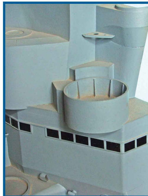
View of the compass bridge with the base of the MG control tower and the base of the 1.5m navigation rangefinder
