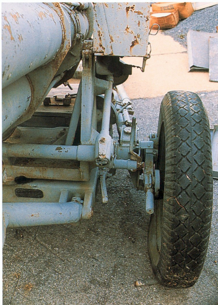
Fig.10 & 11 Details of the launcher tubes elevation and traversing mechanism as well as the complicated wheel suspension. Photos show several different thread patterns occurred on the tires throughout the war. Tires, too, may have varied in size. Note the upright launch assembly support is strengthened on the inside with a welded steel plate wedge.
