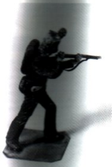
Fig. 14-5. In years past, lead disease, the white powdery build-up seen here, used to wipe out whole armies of model soldiers, but it's rare in modern figures because of their higher tin content.
