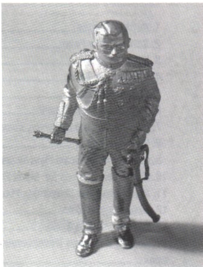
Fig. 1-2. Distortion occurs when the rubber mold is compressed, flattening the cavity into which the metal is poured. It affects 54mm and 90mm figures. Again, no amount of skill in painting can rescue a figure suffering from this malady. The simplest cure is just not to paint it in the first place.
