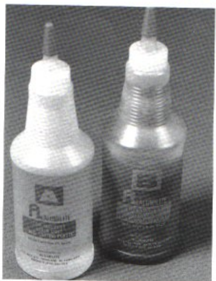
(Top) Fig. 13-17. Casting parts in rubber molds allows you to duplicate your work and saves a lot of time and effort. (Above) Fig. 13-18. Alumilite is a convenient resin-like casting material available in many hobby shops. It is relatively odorless and has a fast setting time (5 minutes or less), which can be extended by storing the bottles in the refrigerator.
