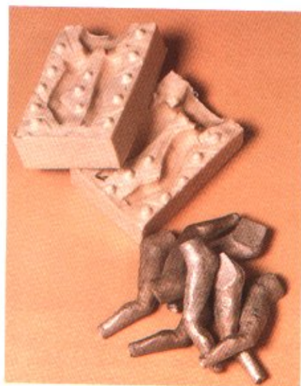
Fig. 13-19. Making a one-piece mold
