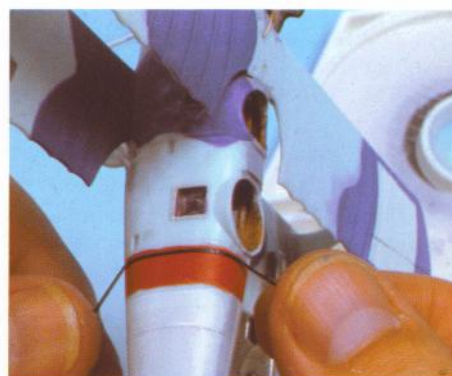
The red band is subsequently masked with flexible tape.
