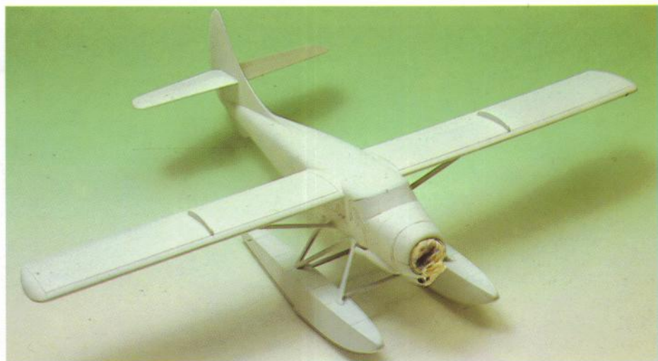
The airframe is coated in acrylic white before applying the colours.
