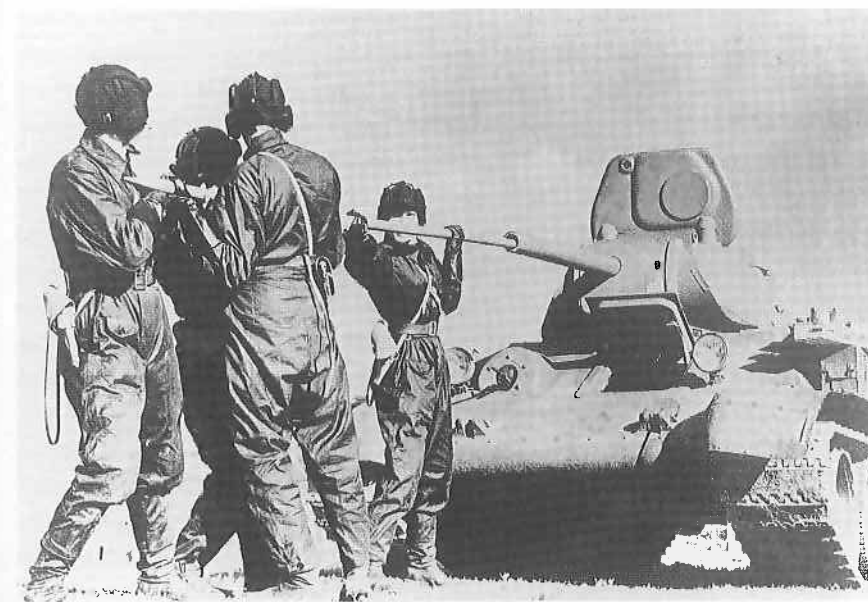
A T-34 crew "punches the gun tube" in order to clean the T-34's gun barrel of carbon residue after firing a significant number of rounds. [Tank Museum, Bovington]
