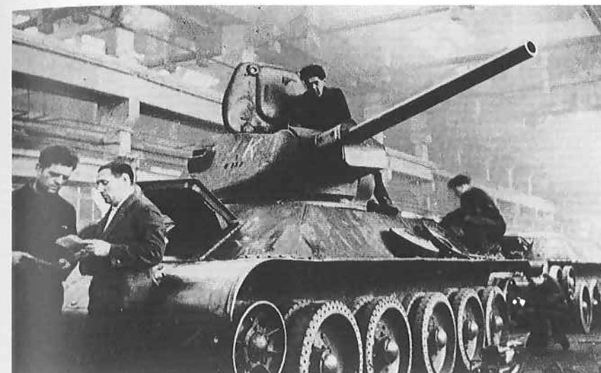
Building a T-34/76 in the Urals. A T-34/76 in 1943 cost 135,000 rubles [$25,470] and required about 3,000 man-hours to complete. A Panther cost about 129,000 Reichsmarks [$51,600] and 55,000 man-hours to complete. (Tank Museum, Bovington)
