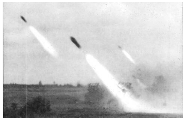
Below: Nebelwerfer rockets are launched in a salvo from several launchers towards Soviet lines. The rockets were particularly useful in suppressing large area targets, as it was impossible to aim them accurately.
