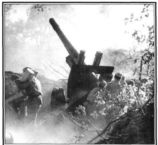
Below: The Soviet barrage caught the Germans by surprise and disrupted their preparations for the offensive. The gun shown below is a Soviet M1937 (ML-20) howitzer firing massive 152mm (6in) shells.
