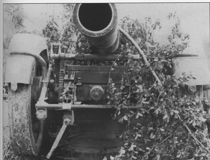
Two additional photographs of a 21cm Mörser 18. It would appear that this gun has been emplaced and subsequently concealed with foliage as the traverse platform is lowered and the wheels raised off the ground. Note the unusual barrel or keg emblem on the right mudguard from an unidentified unit.
