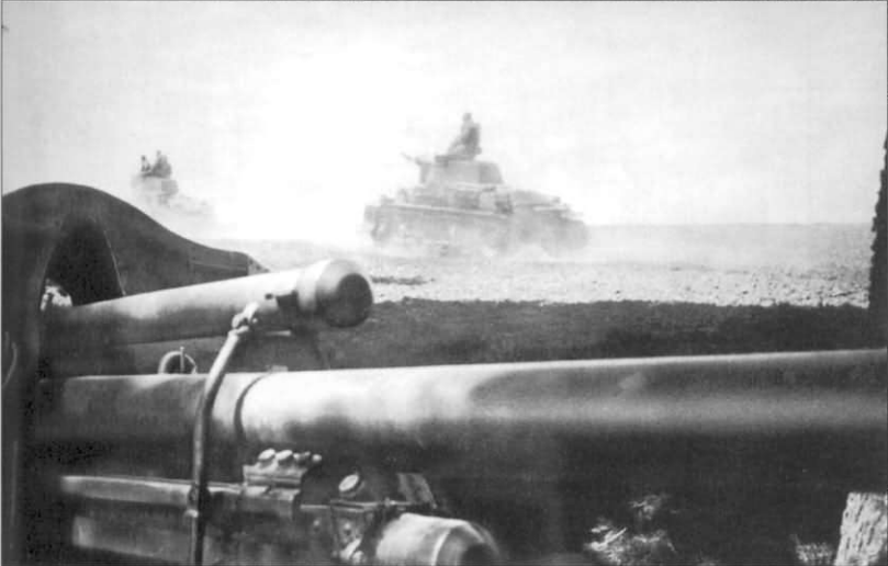
Two Pz.Kpfw.35(t) from 6.Panzer-Division cross a dusty field in front of a 10.5cm leichte Feldhaubitze 18 or leFH 18, which was the standard field gun in the Artillerie-Regiments of both the panzer and infanterie divisions. The Panzer 35(t)s carry the standard load of jerry cans for this campaign, two mounted on edge on the rear of the fender and three laying flat on the engine deck.
