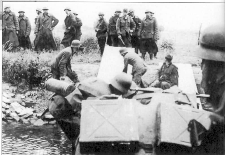
A 3.7cm Pak 35/36 antitank gun is manhandled into position by its crew. This was the only dedicated towed antitank gun in service with the Wehrmacht at this time and it proved to be very ineffective against most French tanks, except at extremely close range. Ammunition boxes have been hung from the front shield for easy access and transportation. The bicycle-mounted Gefreiter to the right appears to be looking at a dead or wounded comrade lying on the ground.
