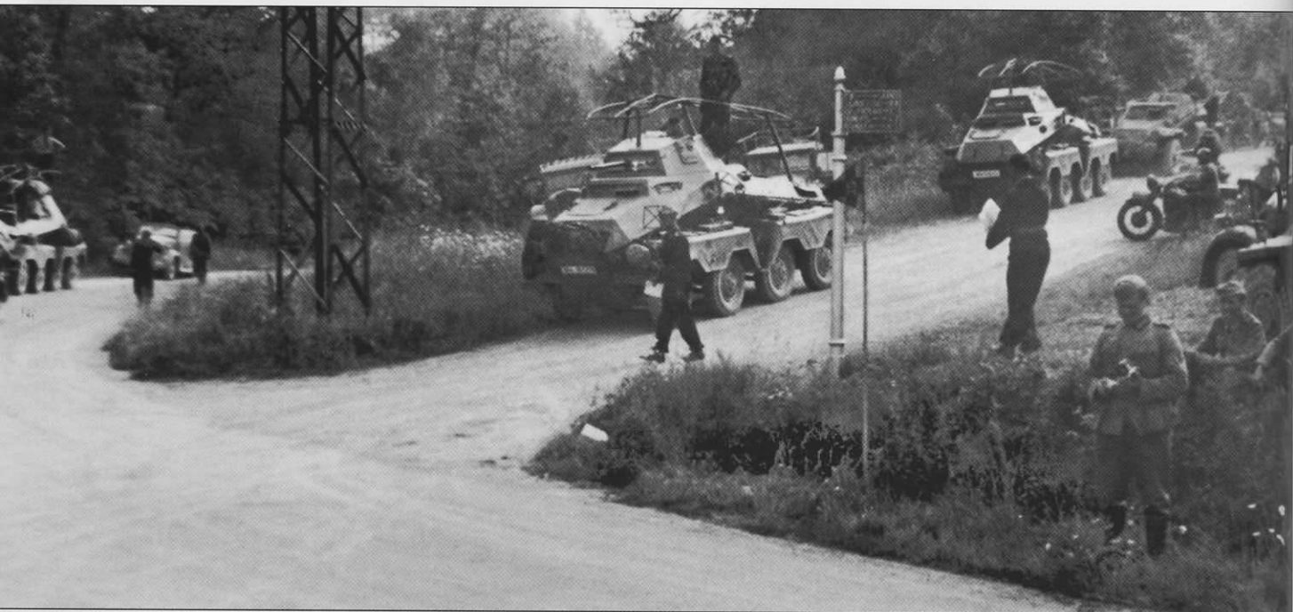
Reconnaissance elements of Rommel's 7. Panzer-Division, presumably from Aufklärungs Abteilung 37, in the vicinity of Cherbourg on June 18, 1940. An Sd.Kfz. 223 with its frame antenna folded down follows two Sd.Kfz. 232 (8 Rad) and a Sd.Kfz. 263 is to the left. Notice the command pennant frame on the tender of the nearest armored car.
