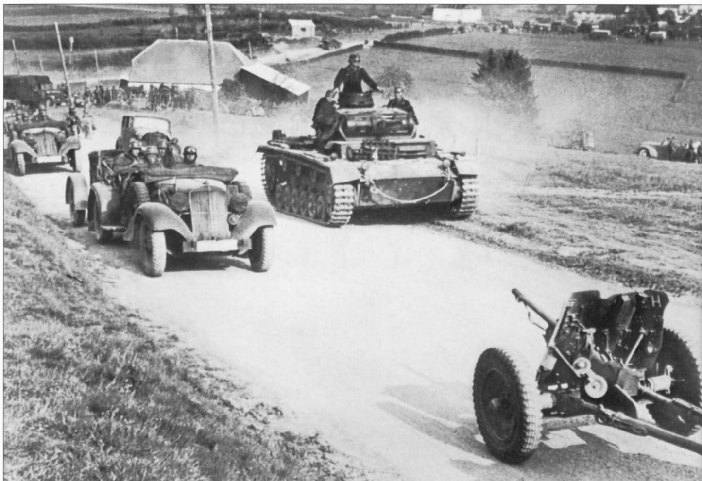
A column of Kfz. 12 (Horch 830 R) towing 3.7cm Pak 35/36 anti-tank guns and trailers passes a Pz.Kpfw. III Ausf. E on a dusty road in Belgium on May 17. The speed of the advance over the previous week left many of the infantry and supporting units far behind. In the background can be seen numerous cars and trucks as they attempt to catch up with the panzer regiments. The letter "H" on the inside of the gun shield probably indicates the individual gun within the company, as the standard anti-tank company at this time was equipped with 9 guns.
