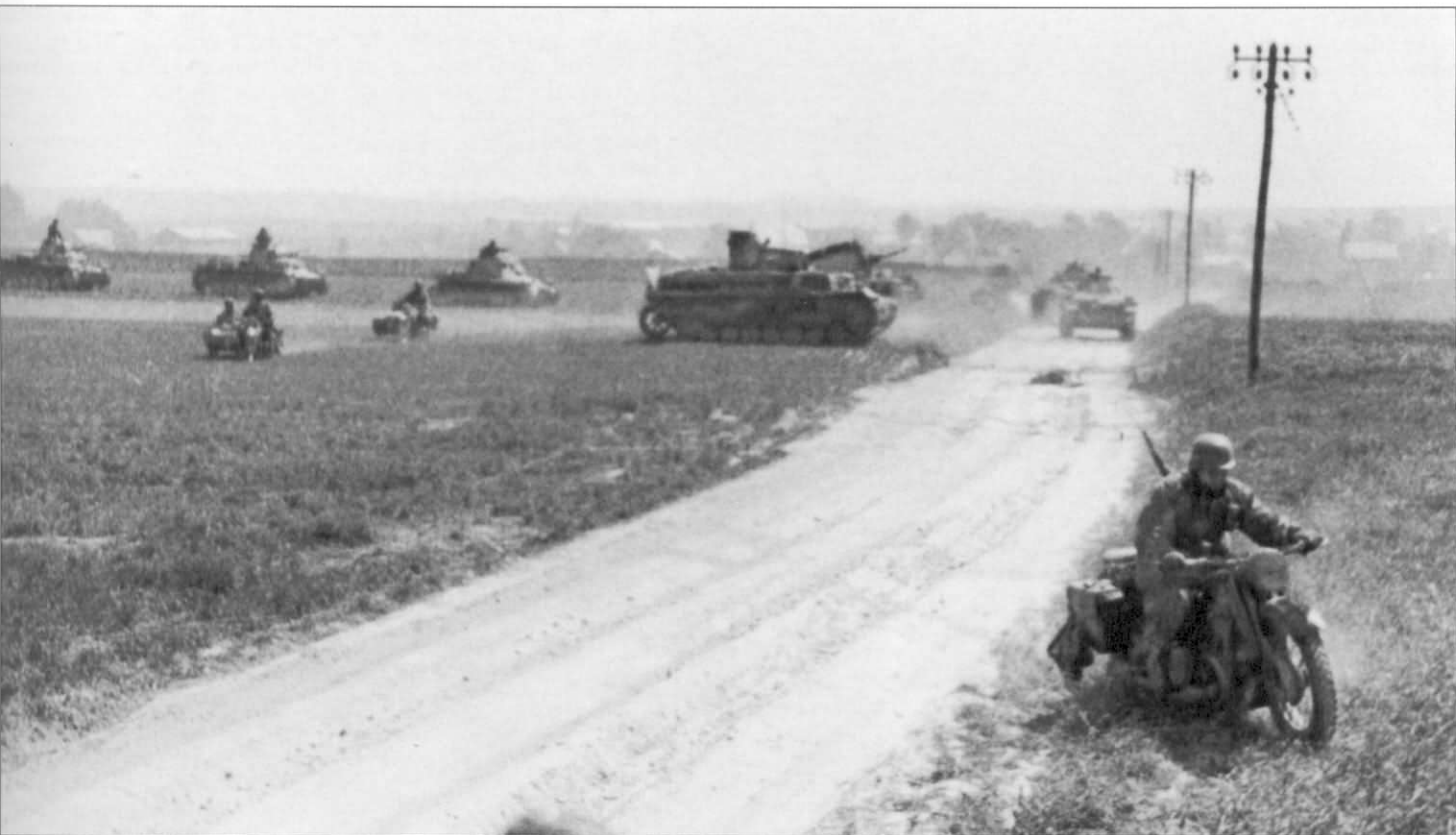
Several types of panzers and motorcycles from 7.Panzer-Division advance across a French field towards a road and village. Nearest to the camera is a Pz.Kpfw.IV, followed by a kl.Pz.Bef.Wg.I Ausf.B and two Pz.Kpfw.II. Immediately behind the Panzer IV is what appears to be Pz.Kpfw.38(t). As seen here, motorcycle mounted infantry was a primary component of the German blitzkrieg and although vulnerable to small arms fire, it allowed the infantry to keep pace with the panzer units during their advances.
