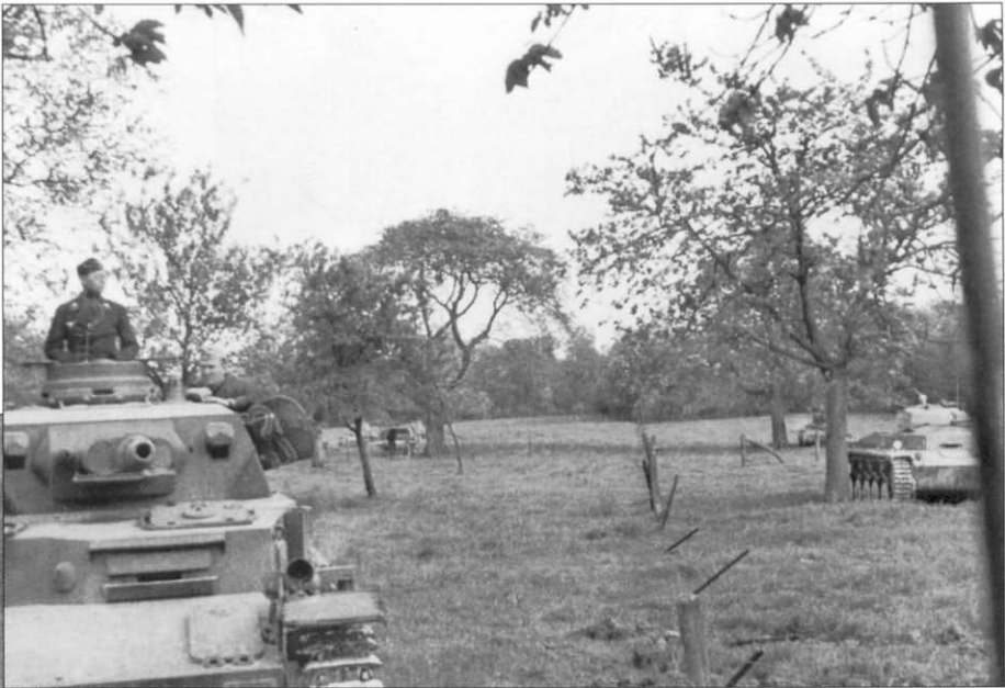
A unique set of four photographs taken roughly in sequence of a Pz.Kpfw.IV Ausf.D from 7.Panzer-Division. The familiar red with thin white outline tactical numbers are apparent from the open turret doors, of which a "3" is visible. In the background can be seen additional Pz.Kpfw.IV, as well as Panzer IIs and 38(t)s. Notice that the turret crewman wears a field gray version of the Feldmutze (sidecap), while the commander's is black.
