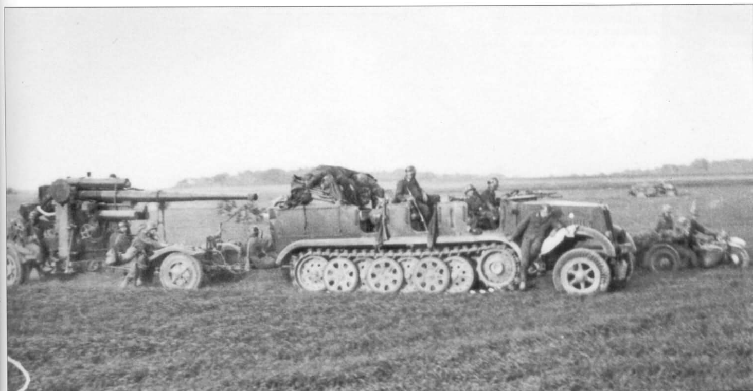
An Sd.Kfz.7 8-ton halftrack towing an 8.8cm Flak 18 on an Sd.Ah.201 sits in a field in France while its crew takes a much needed break. This gun invariably belongs to a Luftwaffe Flak unit as the few Panzer-Jäger-Abteilung equipped with 88s in the Battle of France used the modified guns with large shields. Although the Flakartillerie was employed against French tanks in some instances, this was not a common occurrence and many more enemy aircraft were destroyed than tanks.
