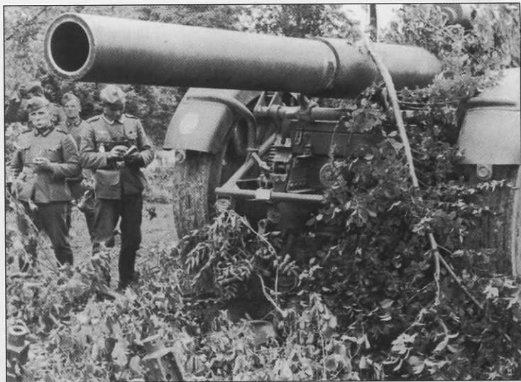
Two additional photographs of a 21cm Mörser 18. It would appear that this gun has been emplaced and subsequently concealed with foliage as the traverse platform is lowered and the wheels raised off the ground. Note the unusual barrel or keg emblem on the right mudguard from an unidentified unit.
