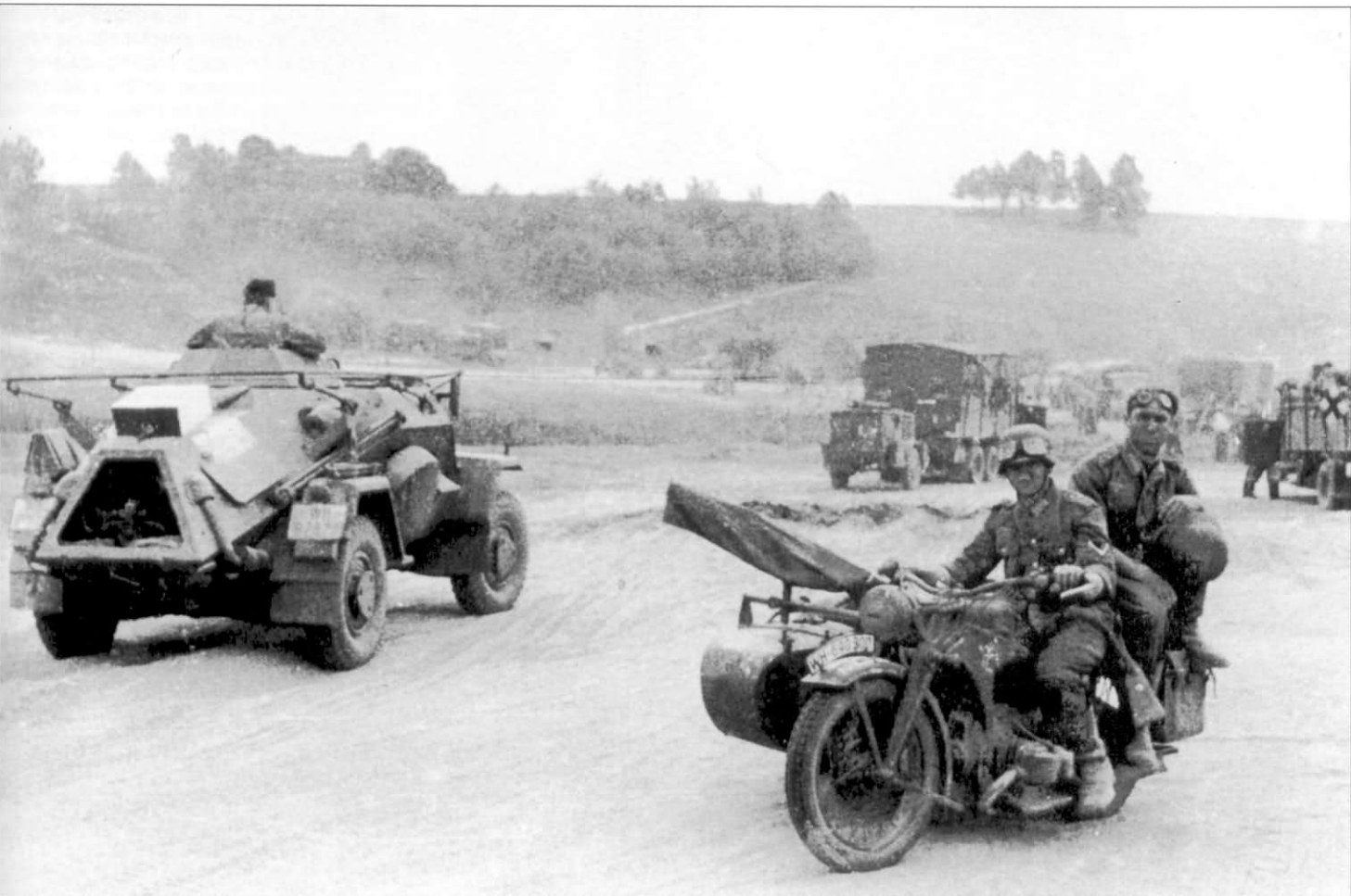
An array of vehicles move through a shallow valley, with a Zündapp KS600 motorcycle combination in the foreground, equipped with an MG34 mounted on the sidecar. The Sd.Kfz.223 (WH82875) has its frame aerial folded down and the white aerial recognition rectangle can be seen painted across the top of the stowage box and down either side onto the hull. It is missing the rear ventilation grille, most likely removed due to irreparable damage. Further up the road is a Henschel Type 33 D1 6x4 truck towing a compressor or generator.
