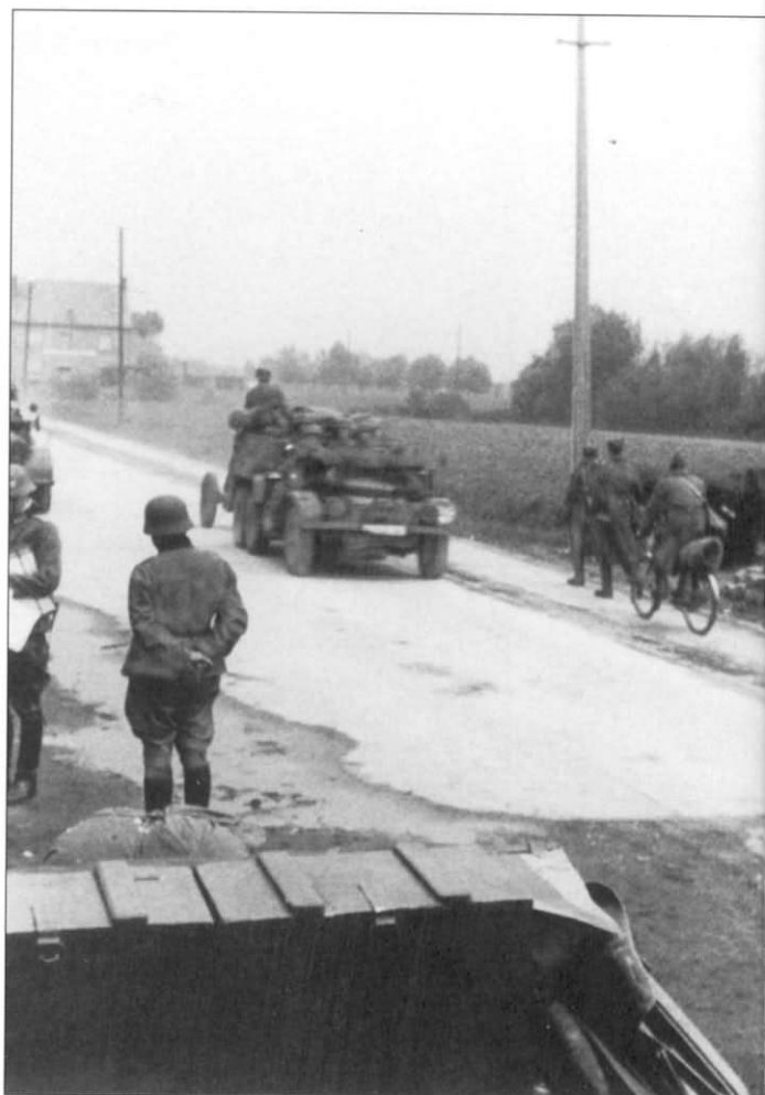
A Krupp Protze Kfz.69 truck pulling a 3.7cm gun on a road in France. This light truck was very common throughout the early battles of WWII and served a variety of roles, particularly as a prime mover for the 2cm Flak 38 and Pak 35/36 seen here.
