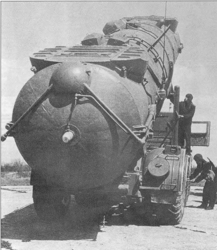
The Soviet Navy acquired an anti-ship version of the FKR-2 system called the Redut (SSC-1b Shaddock). It was similar to the Air Force FKR-2 system, but the cab designs were significantly different. The coastal defense version of the launcher was called the SPU-35V. These served with the Soviet Navy's BRAV coastal defense units starting in the 1960s.
