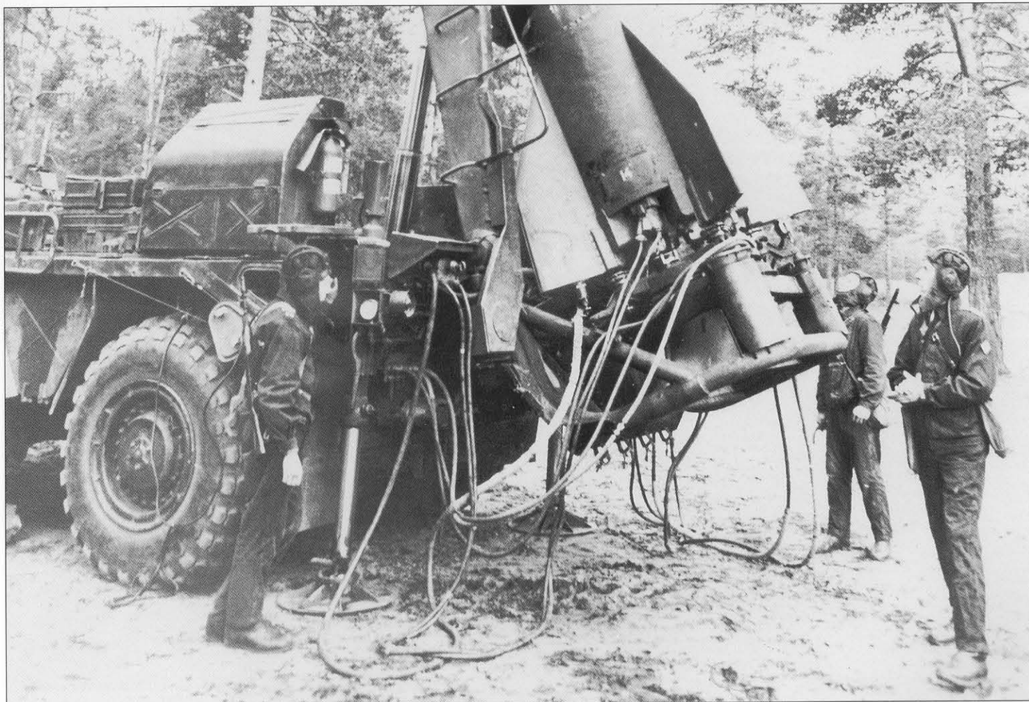
An R-17 missile being prepared for firing. A large amount of cabling is required, some of which is used to pass ignition signals to engine components, other of which provides data back to the launch control station to monitor the status of the missile prior to launch.
