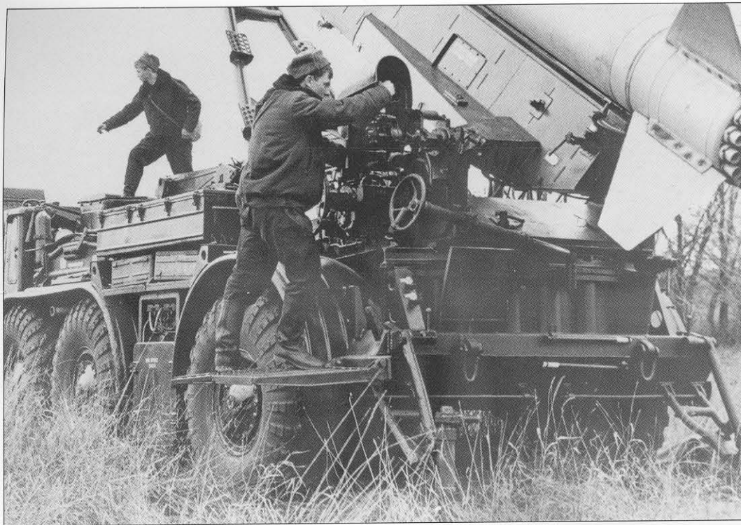
When the 9M21 rocket is being prepared for launch, a pair of platforms on either side are lowered to allow the crew easier access to the sighting and aligning equipment at the rear of the launch station.
