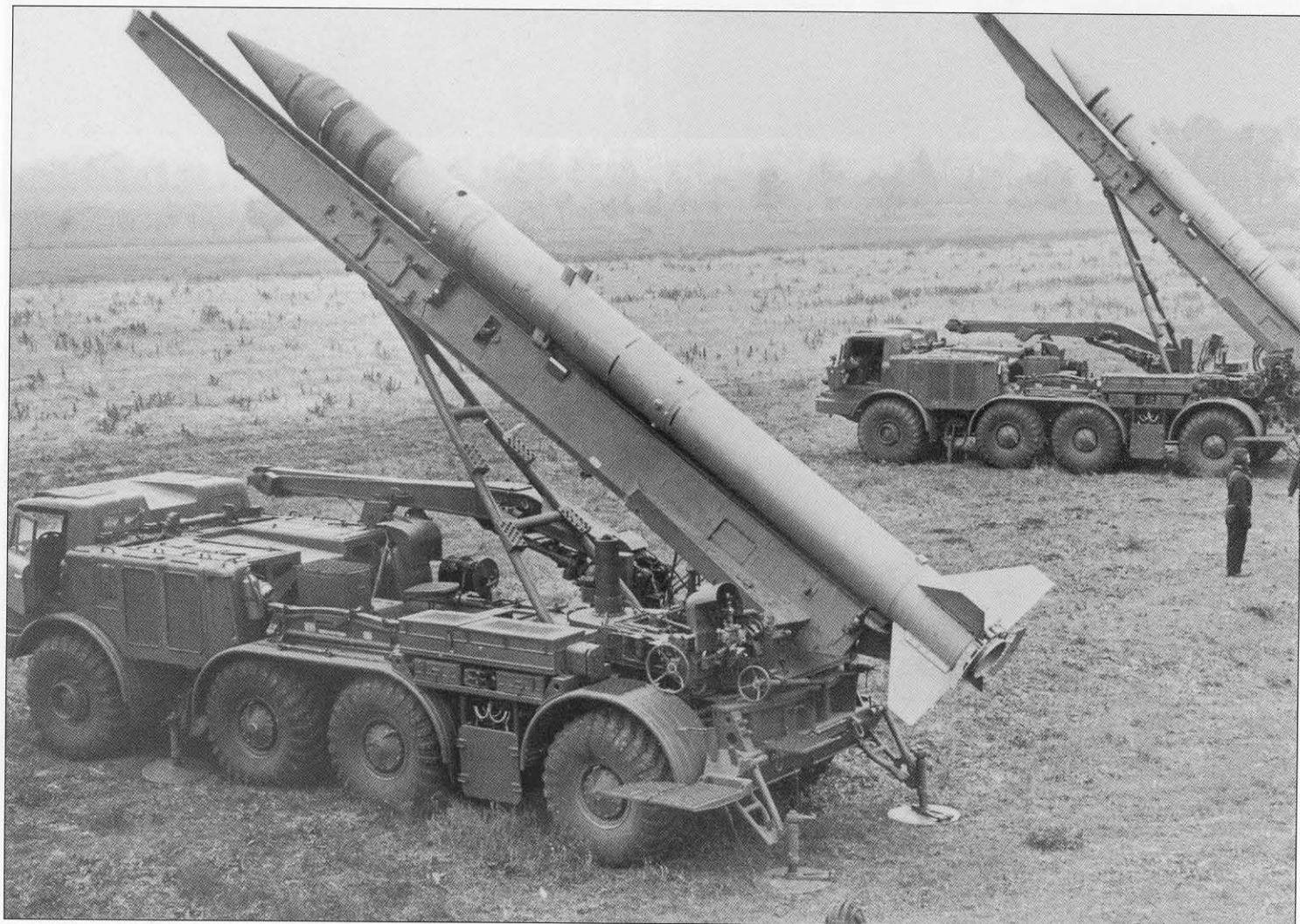
A Luna-M launch battery ready to fire. Note that there are four stabilizing jacks on the 9P113 TEL, a pair behind the front axle and another pair at the rear. (Sovfoto)
