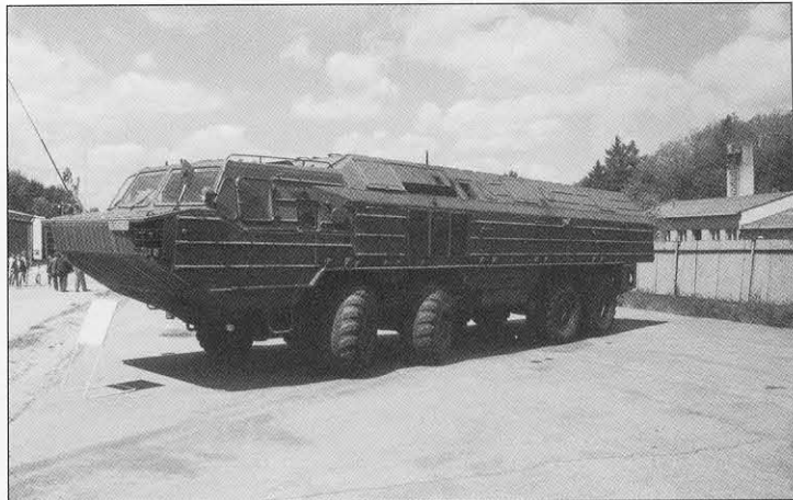
This is the 9P71 TEL with the missile stowed inside. Although similar in appearance to the 9P129 Tochka, it is in fact considerably larger. This is a retired Czechoslovak example. (Andrzej Kinski)
