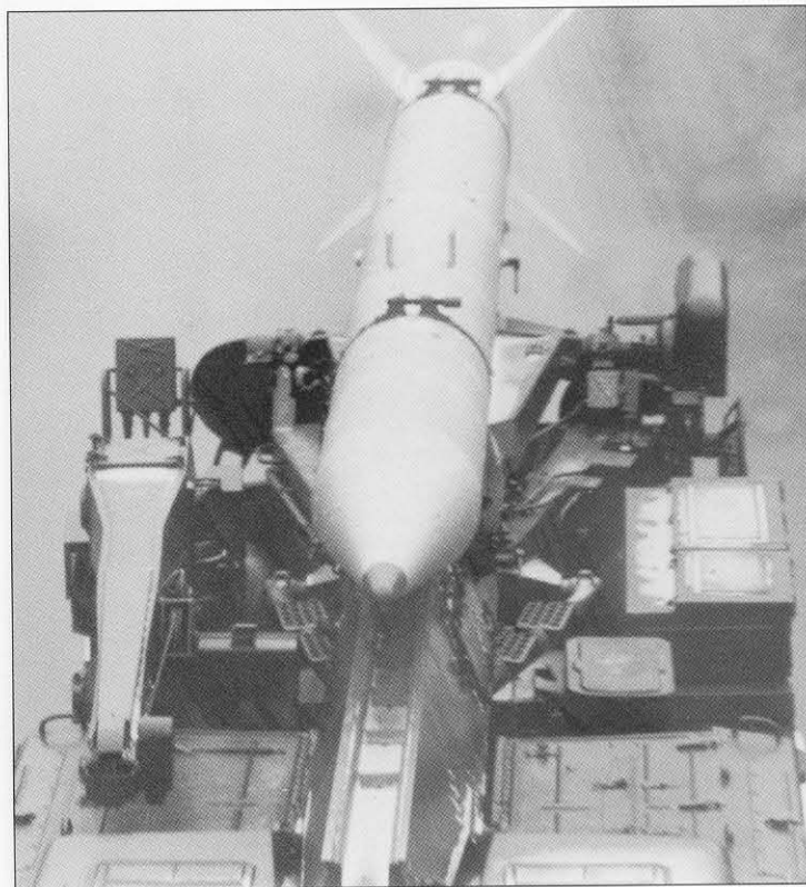
An overhead view of a 9P113 launcher vehicle. The 9P113 designation for the BAZ-135LTM vehicle has the following meaning: 9= tactical missile; P= puskovaya ustanovka (launch system) and 113 is the numerical sequence of this particular launch vehicle. The two vertical fins evident midway down the rocket fuselage are intended to keep the rocket firmly on track when fired from the launch rail.
