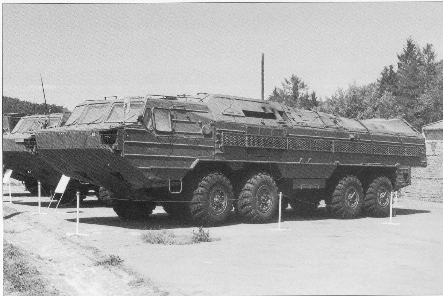
This could be mistaken for an 9P71 launcher vehicle but it is in fact the 9T230 transloader vehicle, based on the same BAZ 6944 chassis. Close inspection will reveal that the after compartment is covered by a canvas tarpaulin and lacks several of the access panels of the launcher vehicle. This is a retired Czechoslovak vehicle. (Andrzej Kinski)
