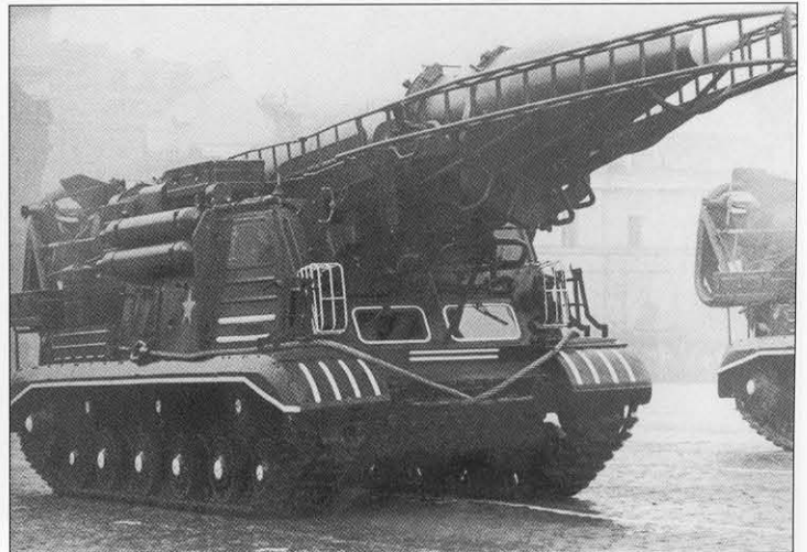
The 8U218 TEL was succeeded by the very similar 2P19. The 2P19 used the new R-17 missile, known to NATO as the SS-1c Scud B. The R-17 missile was longer than the R-11, requiring a reconfigured launcher. The modified 2P19 launcher can be most easily distinguished by the two high pressure air bottles on either side of the vehicle superstructure, as well as by the more elaborate reinforcing frame on the front of the hull.
