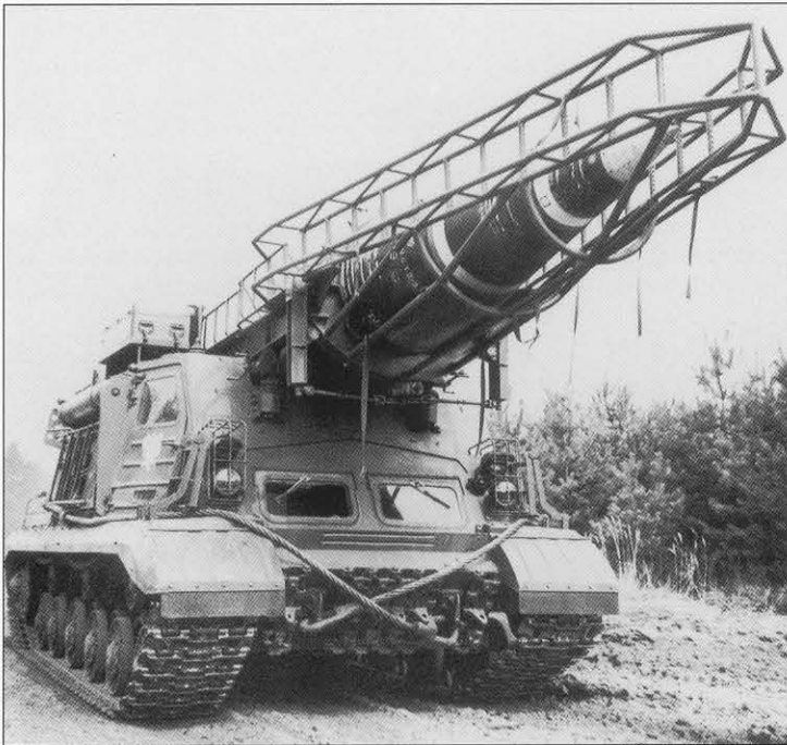
A Polish 8K11 launcher vehicle in the field in the 1960s. The elaborate bracing around the missile was designed in part to protect it against damage, but also permit launch crews to climb up alongside the missile to check various features prior to launch.
