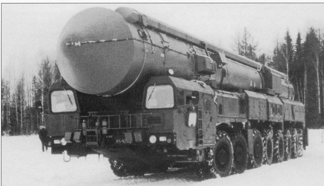
The latest Russian missile system is the Topol-M, known in the West as SS-27. It is a further evolution of the Topol, but larger. A mobile version has been planned, and the prototype was built on the MAZ-79221 truck chassis as seen here. This superficially resembles the earlier Topol TEL on the MAZ-7917, but it has eight axles rather than seven.
