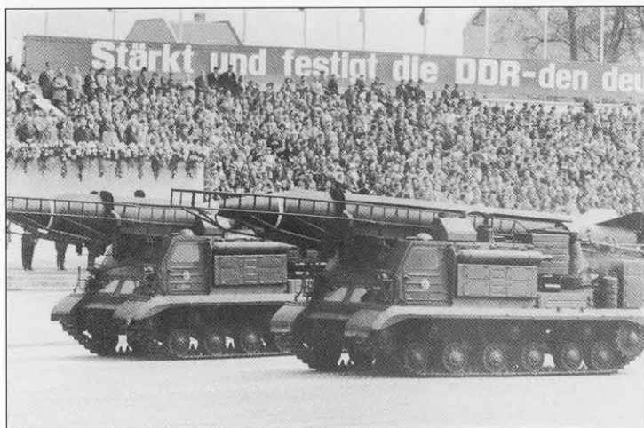
The earliest model of the Scud, the R-11 missile, was mounted on a modified ISU-152 heavy assault gun chassis called the 8U218 TEL. It was reminiscent of the similar Fillin/FROG-1 launcher seen earlier in this book. The 8U218 launcher vehicle can be distinguished from the later 2P19 version by the presence of one high pressure air bottle on the hull superstructure- the later 2P19 version had two bottles on either side. This is a Polish LWP 8U218 launcher vehicle. There is a thermal blanket over the warhead to maintain temperature.
