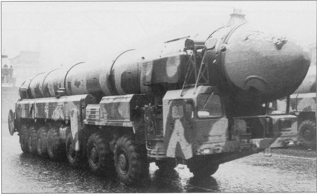
A side view of the RT-20P's Obiekt 821 TEL. Although based on IS heavy tank components, the TEL is considerably larger than tactical TELs of the period such as the 2P19 Scud TEL.
