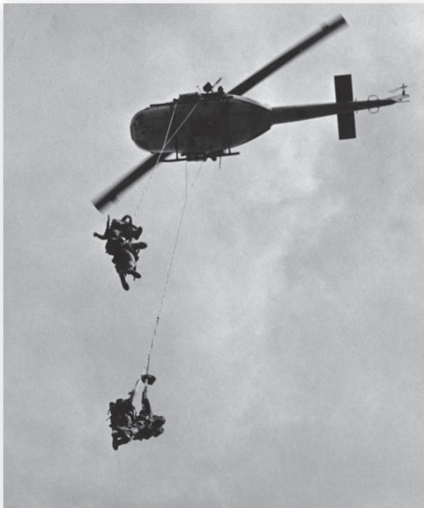
A UH-1H Huey extracts an RT during training using STABO rigs. This was a harness arrangement incorporated into the recon man's web gear in lieu of load-bearing equipment suspenders. A Special Forces NCO and two officers developed the system in 1969 at the MACV Recondo School. (Dale Boswell via John Plaster)
