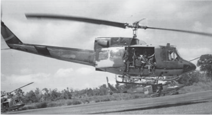
The Air Force's 20th Special Operations Squadron used Bell UH-1F, P, and N Huey helicopters to insert and extract SOG reconnaissance teams in Laos and Cambodia from 1965–72. Known as “Green Hornets,” they were armed with two M60 machine guns. Some helicopters carried a pair of seven-tube 2.75in. rocket pods. The Green Hornets could be identified by their four-color camouflage pattern (olive green, forest green, black, and sand) and their light-gray underbelly. Army Hueys were painted in solid olive green. Green Hornets bore no national markings. (Alfonso Rivera via John Plaster)
