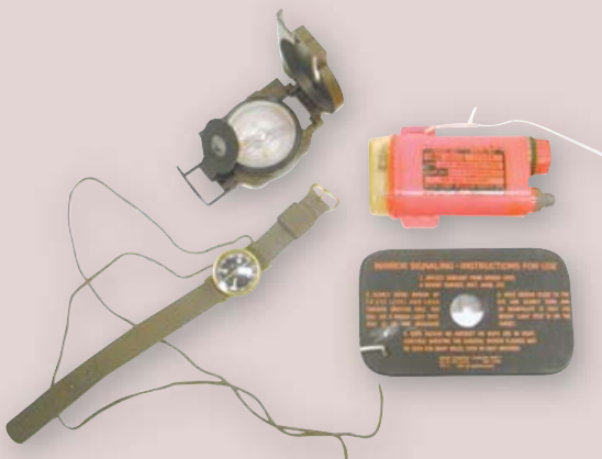
Typical items carried by a LRP, (left to right): Lensatic compass attached to the person by a dummy cord; wrist compass on an olive drab web band carried as a backup; SDU-5E strobe light; Mk 3 signal mirror (backside). (Trey Moore collection)
