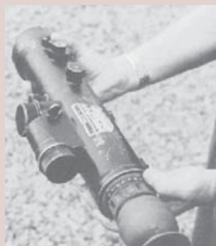
An AN/PVS-1 "starlight scope" that could be mounted on an M14 or M16A1 rifle. These first-generation night vision weapons sights were heavy and of marginal effectiveness. (US Army)
