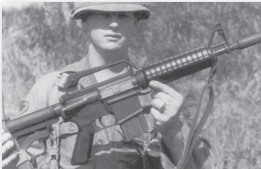
The 5.56mm XM177E2 submachine gun was issued to many recon teams. Its compact design was ideal for use by LRPs. This is a 20-round magazine. Curved 30-round magazines were extremely rare. (US Army)
