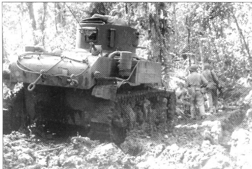
An M3A1 of B Company, 3d Tank Battalion, on the jungle trails of Bougainville, November 1943. Notice the pistol port open on the turret rear, for ventilation. Towing cables are ready for hookup to other tanks as bogging was frequent in such terrain. The anti-aircraft machine gun is dismounted and could rarely be used in such close conditions. (US Army Signal Corps (SC) photo)
