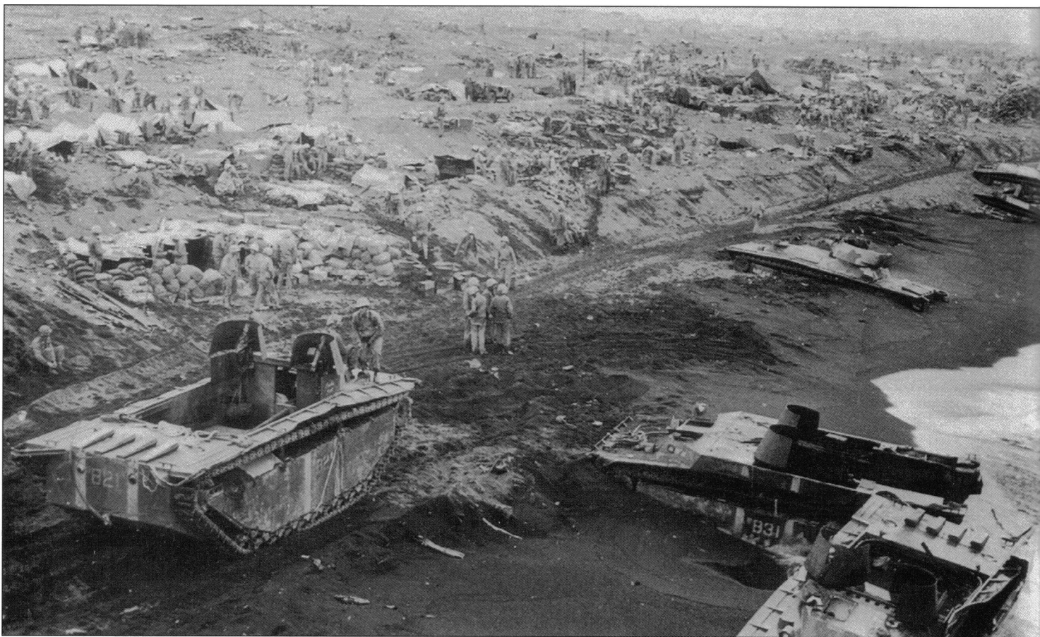
The congested Yellow Beach 2 area on Iwo Jima. The hot black volcanic sand has already started to envelope some of the amtracs and amtanks disabled near the shoreline. This view shows a couple of LVT(A)-2 amtracs including "B-21" to the left, a LVT-4 (B-31) and a LVT(A)-4 amtank. (USMC)
