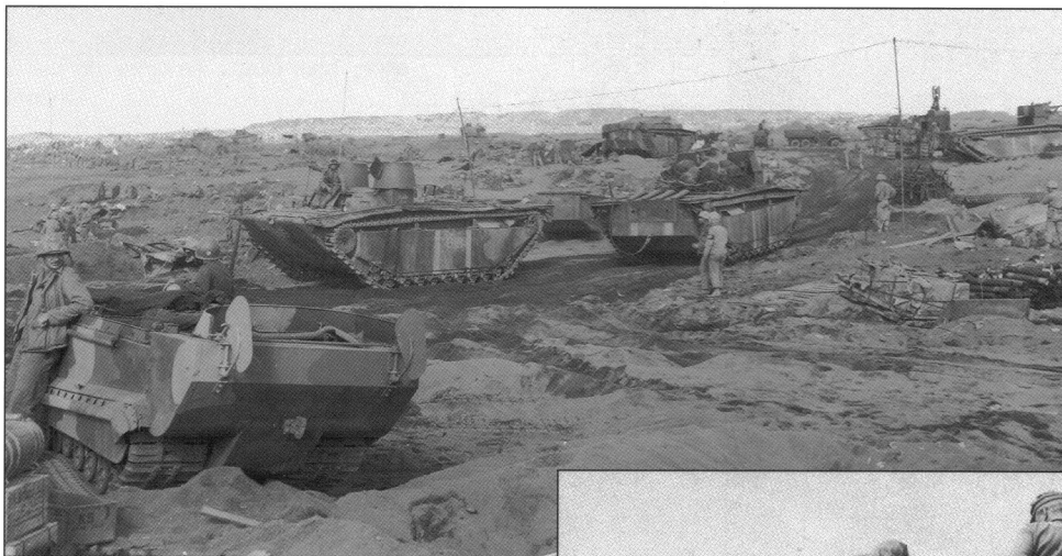
The congested Yellow Beach 2 area on Iwo Jima. The hot black volcanic sand has already started to envelope some of the amtracs and amtanks disabled near the shoreline. This view shows a couple of LVT(A)-2 amtracs including "B-21" to the left, a LVT-4 (B-31) and a LVT(A)-4 amtank. (USMC)
