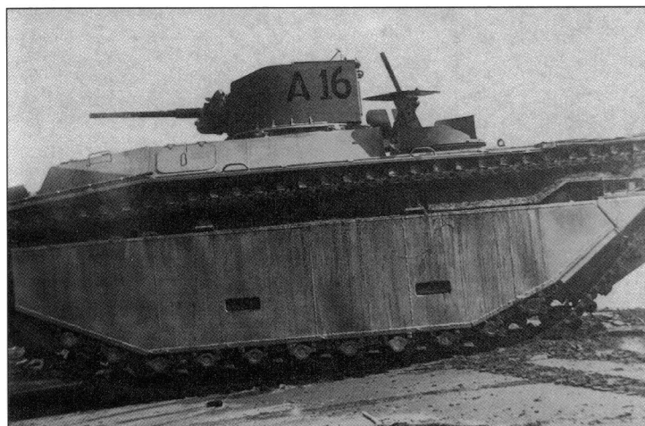
A good side view of a standard production LVT(A)-1, in 1943. This is the standard production version, with an armored collar around the rear machine gun stations, and an armored shield. (US Navy)
