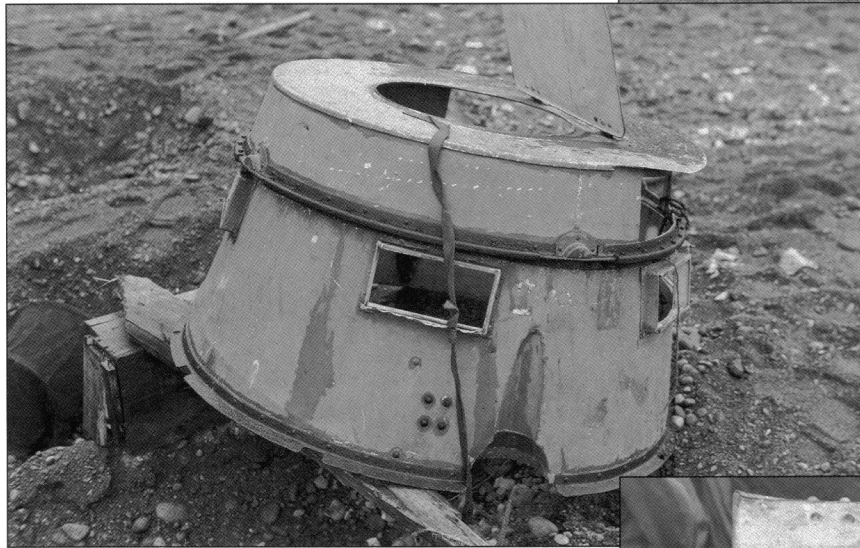
The Type 2 Ka-mi turret hatch was covered by this turret cover which also allowed the tank commander to get a better view of the beach area during the approach.
