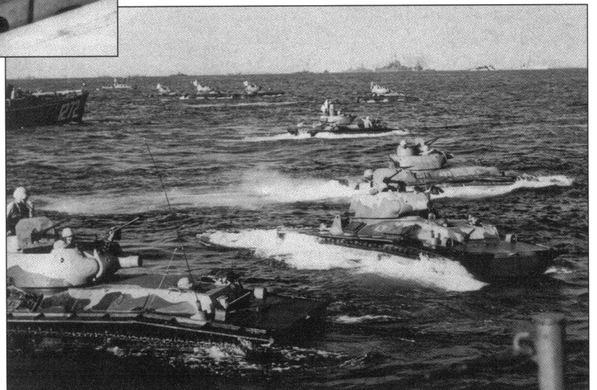
A wave of LVT(A)-4 amtanks move to shore. These are fitted with the circular armored parapet, with large expedient armored shields for their .50 cal machine gun.
