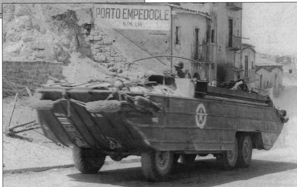
A US Army DUKW passes through Porto Empedocle on 25 July 1943. It carries the circled star, which was the standard US Army identification marking for the Sicily operation. Less visible on the lower bow is the colored bar code, a system of coded markings used to identify units during amphibious operations. (MHI)
