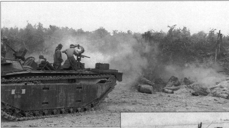
The Army's 2nd Engineer Special Brigade Support Battery modified a number of LVT(A)-2 amtracs to provide fire support. On the stern is a 37mm automatic cannon taken from a P-39 fighter aircraft and mounted on an improvised pintle. In the cargo bay are the rails for a barrage rocket launcher. This vehicle is being used to attack Japanese dug-outs on Schouten Island in the Dutch East Indies in 1944. The cartoon on the hull side shows a snorting bull. (US Army)
