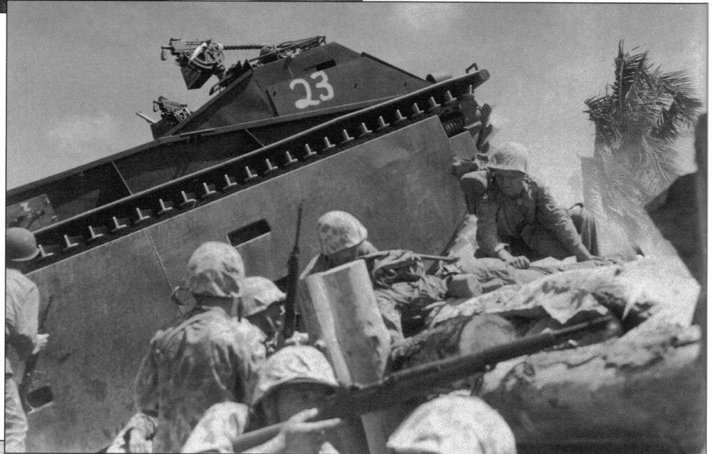
A view along the hotly contested sea wall at Red Beach 3 at Betio on 20 November 1943 with a LVT-1 knocked out in the background. Notice that armor plate has been added around the driver's compartment. In spite of the armor, losses of the amtracs near the sea wall was very heavy. (USMC)
