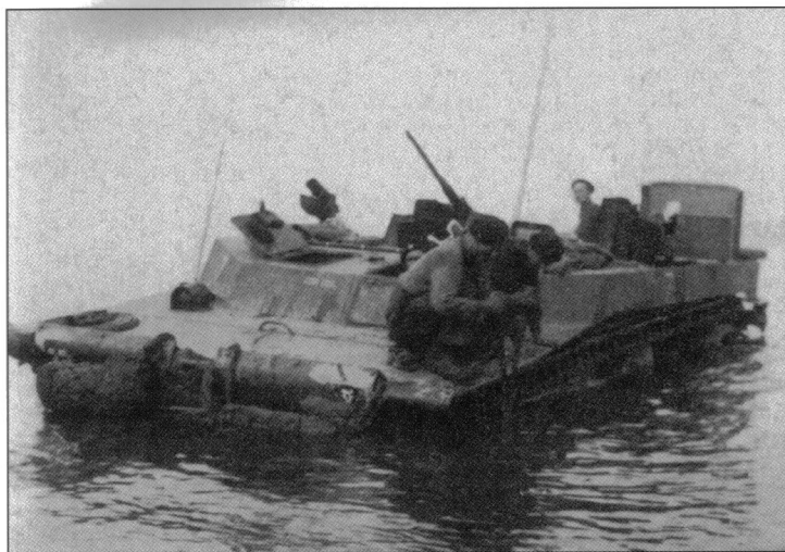
A Buffalo IV (LVT-4) of the 5th Assault Regiment RE in the waters along the Dutch coast during the autumn 1944 operations. The armored cover over the side machine gun station is evident in this view. (USNA)
