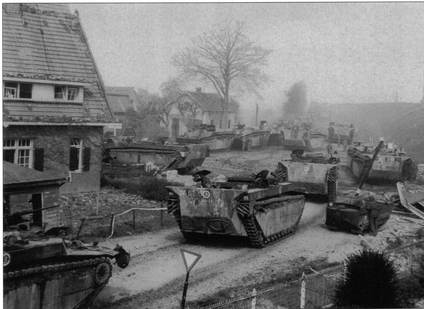
Buffalo IVs of the 1st Lothians, 79th Armoured Division, prepare for operations in a small Dutch town. This unit also made limited use of M29C Weasel amphibious utility vehicles, one of which can be seen to the right. There is considerable variation in the machine gun mountings on the vehicles, some using simple shields, other using enclosed shields. (USNA)
