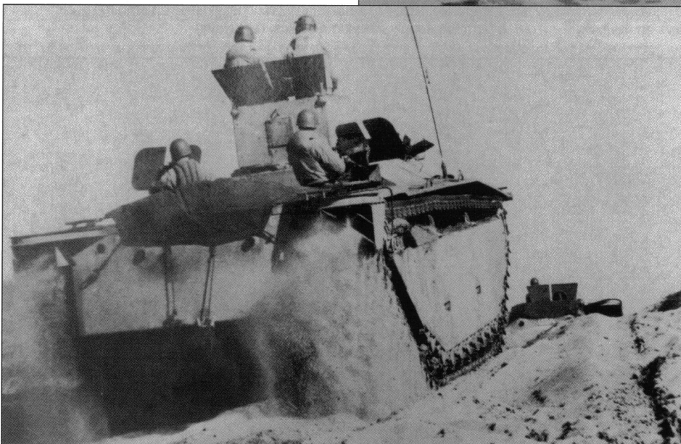
A pair of LVT(A)-1 amtanks during training exercises on the California coast in 1943. This provides another view of the canvas cover over the engine deck, and the two rear machine gun stations. (US Navy)
