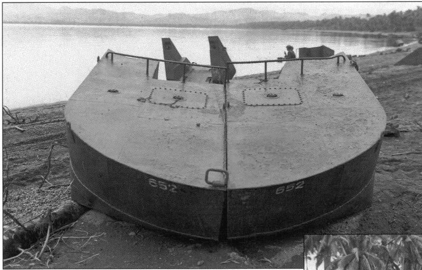
This is a set of bow pontoons from one of the Ka-mi amphibious tanks that landed at Ormoc bay. The vehicle number can be seen painted on the bow. (US Army)
