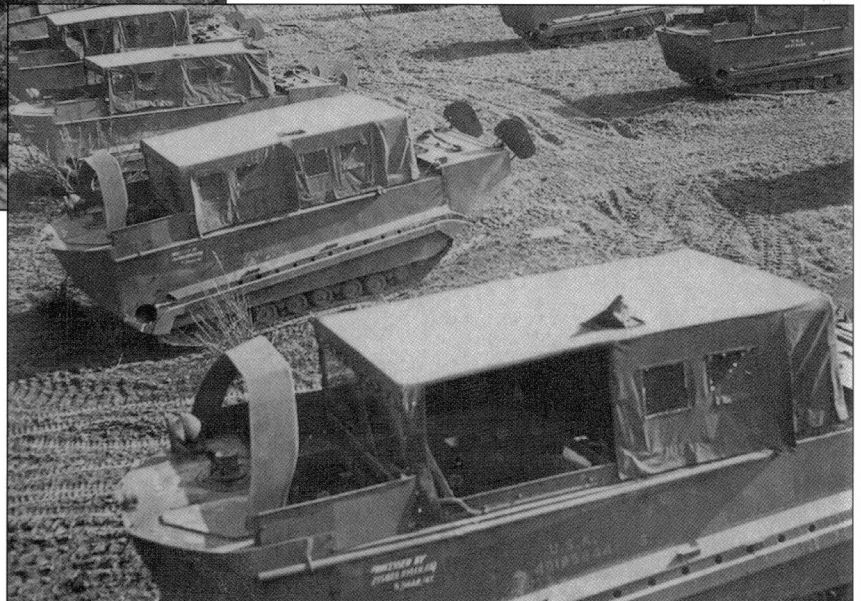
This motor pool in Germany at the end of the war shows a number of M29C Weasels with the full canvas tarp erected. The bow splash plates, designed to prevent water from flowing over the box into the cabin, have been folded upward. (MHI)
