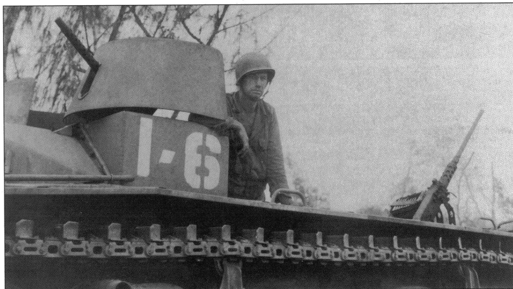
A close-up of the modifications undertaken on many Army and Marine amtracs before Saipan. An armored extension was added behind the normal driver's compartment, and a pintle mounted .30 cal machine gun with an improvised shield was added for more firepower. (USMC)
