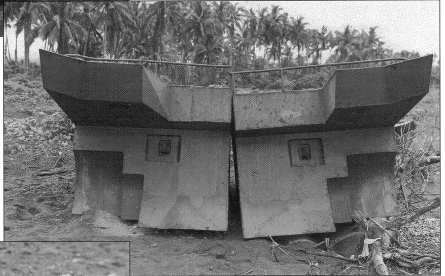
A rear view of the bow pontoons shows that it was in fact made up of two parts. The small square indentations in the lower portion of the pontoon are the attachment points which were gripped by the crab-claws on the tank hull. (US Army)
