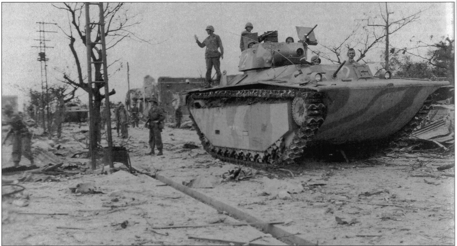
A Marine LVT(A)-4 of the 2nd Armored Amphibian Battalion on Tinian in August 1944. The two turret machine guns have had improvised armored shields added. In addition, the vehicle has pattern painted camouflage. (USMC)
