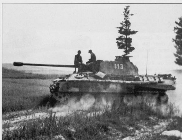
This 'Panther' Ausf.A with tactical number '113' carries several additional track links supported by the long unditching log on the side of the hull. The gun cleaning rod tube normally fixed here has been moved to the rear of the engine deck. There is an unusual, black number '8' painted on the front side skirt. The notch in the front of the skirt plate identifies it as originally coming from farther along the side of this, or possibly another, vehicle. A three color camouflage paint scheme has been applied.
