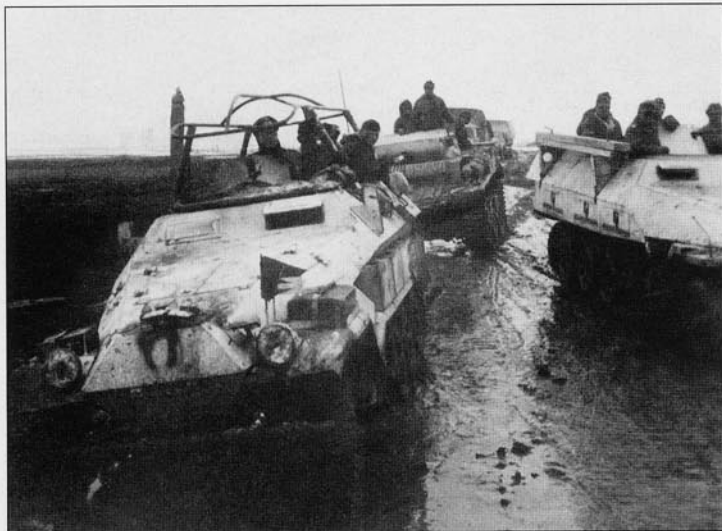
The familiar Sd.Kfz.251/6 Ausf.B command half-track of Gen.Lt. von Saucken on the left and an Sd.Kfz.251/7 Ausf.D Pioneerpanzerwagen on the right followed by one of the Division's early Pz.Kpfw.II Ausf.L 'Luchs' and two transport trucks. The assault bridges normally carried by the Pioneer half-track are missing and a couple of wooden planks are in their place. It didn't take long for wet, muddy conditions to compromise the winter camouflage of these vehicles.
