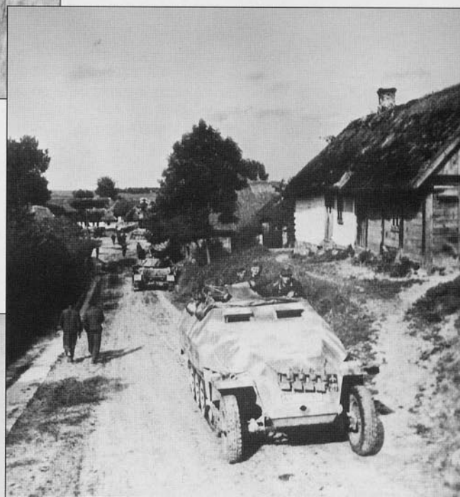
An Sd.Kfz.251/1 Ausf.D makes its way through a small village. The tactical marking to the right of the spare tracks links indicates this vehicle is from 7.Kp. of either Pz.Gren.Rgt.59 or 112 of 20.Panzer-Division. The Division suffered heavy losses and the remainder was incorporated into 4.Panzer-Division in the middle of July, 1944. The camouflage pattern is composed of large areas of green and brown on the dark sand base.
