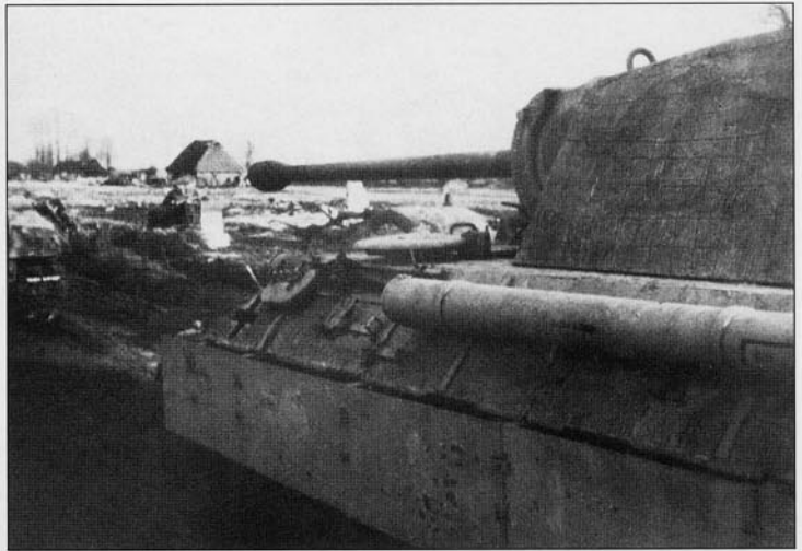
Another view along the same road. This 'Panther' Ausf.A does not have a tactical number painted on the side of the turret but has, what appears to be, a shipping stencil on the gun cleaning rod tube and a national cross on the front hull side. The Zimmerit coating is quite clear in this photo.
