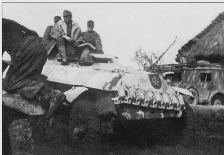
An Sd.Kfz.251/1 Ausf.C, prominently displaying the new Divisional emblem on its front plate and carrying a row of replacement track links, passes through a Russian village. It has a coat of white winter camouflage paint over the dark sand base. Visible in the background is a Horch Kfz.17 heavy wireless car with the telescoping antenna extended. It appears to have a camouflage pattern of dark sand lines over its dark gray base.
