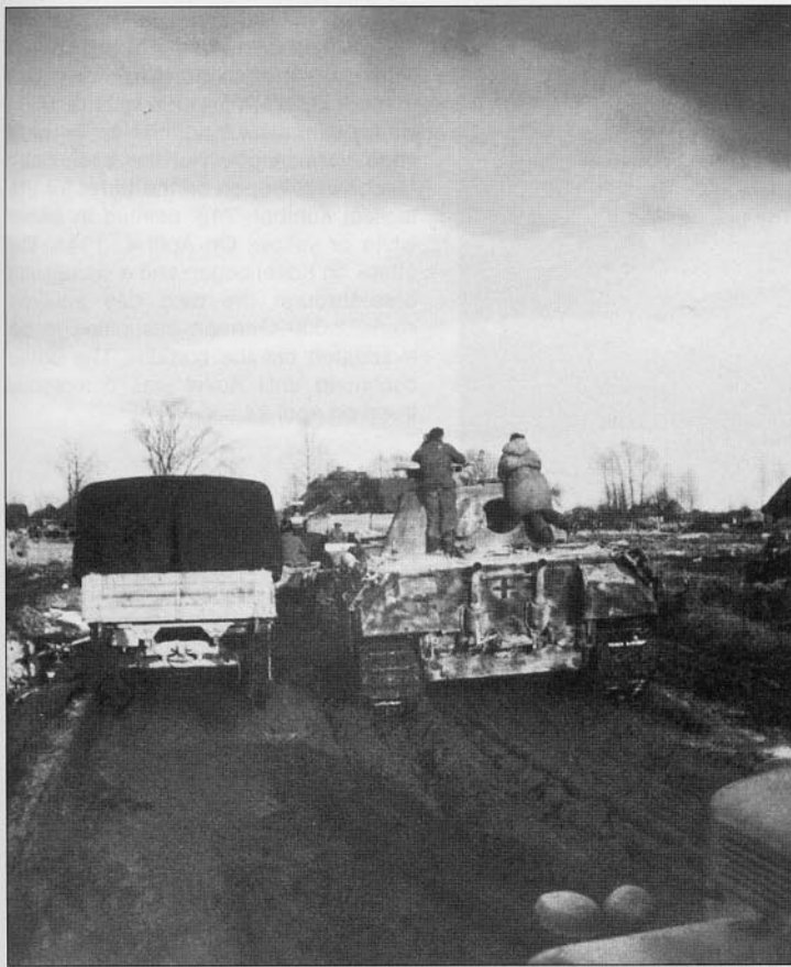
Another view along the same road. This 'Panther' Ausf.A does not have a tactical number painted on the side of the turret but has, what appears to be, a shipping stencil on the gun cleaning rod tube and a national cross on the front hull side. The Zimmerit coating is quite clear in this photo.
