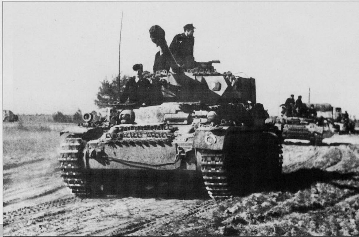
A Panzerbefehlswagen III based on the Pz.Kpfw.III Ausf.J with the 5cm KwK L/42 gun. The hull machine gun was eliminated to make room for an additional radio set. There were 81 manufactured in 1942 with a further 103 converted during 1943. The star antenna can be faintly seen behind the commander.
