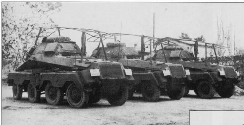
Three new early production Sd.Kfz.263 radio vehicles parked near a rail siding in the spring of 1941 as 4.Panzer-Division was preparing for the invasion of the Soviet Union. The Sd.Kfz.263 was equipped with a long range radio set and was usually used by Nachrichten (signals) units and in Korps and Armee headquarters. They are protected with canvas covers around the crew compartment and on the telescoping mast antenna. The boxes hanging on the sides are metal containers for stick hand grenades. The nearest vehicle carries the license number WH-76694. Just above it can be seen the divisional emblem while on the opposite side of the radiator grille can be seen the tactical sign for a signals unit.
