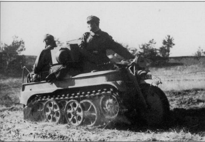
A heavily laden NSU Kettenrad (Sd.Kfz.2) appears to be towing another vehicle just outside the picture to the left. The driver is wearing the waterproof motorcyclist's coat.
