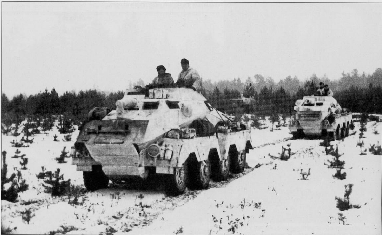
The Sd.Kfz.233 was as rare a vehicle as the "Luchs" with only some 119 produced. Armed with the obsolete 7.5cm StuK37 L/24, they were issued to the Aufklärung Abteilungen of the Panzer Divisions on all fronts. It would appear that both vehicles have had some additional armor protection added to the front.
