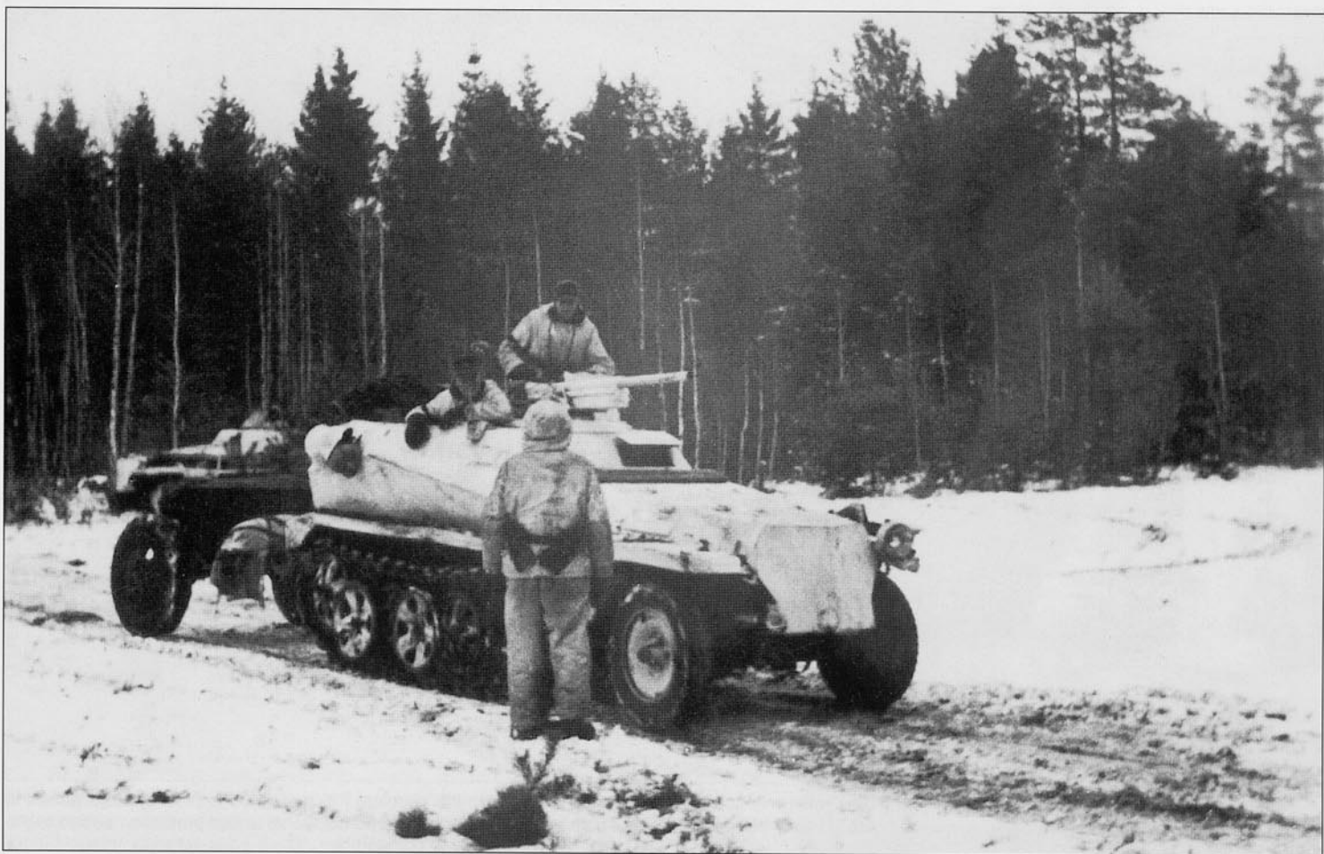
A group of Sd.Kfz.250 half-tracks in white winter camouflage. Two of the vehicles are Sd.Kfz.250/10 armed with the obsolete 3.7cm PaK36 and were usually assigned to platoon leaders. The object draped over the mudguard of the closest vehicle is a wild boar.
