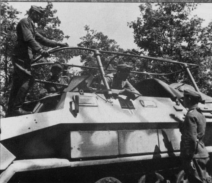
An Sd.Kfz.251/6 Ausf.A, July 1943, which has been retrofitted with the MG shield. It has been camouflaged with sand spots over the dark gray base color.
