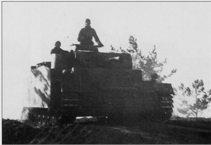
A Panzerbefehlswagen III based on the Pz.Kpfw.III Ausf.J with the 5cm KwK L/42 gun. The hull machine gun was eliminated to make room for an additional radio set. There were 81 manufactured in 1942 with a further 103 converted during 1943. The star antenna can be faintly seen behind the commander.
