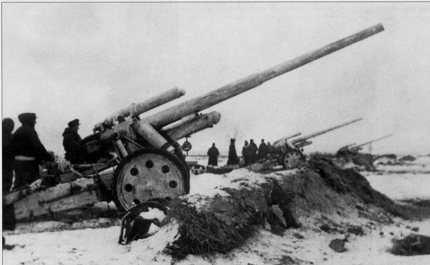
A battery of white camouflaged schwere 10cm K 18 guns lined up to fire on enemy positions. Except for the barrel, this gun was identical to the 15cm sFH18.
