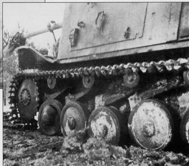
This Marder II has run over a mine, damaging its track and destroying the first roadwheel. Also note the additional armor plate that has been added to the side.
