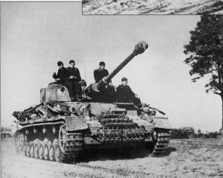
A Pz.Kpfw.IV Ausf.G with a horseshoe fixed to its left mudguard for luck. Note the additional 30mm armor plates welded to the front of the hull and superstructure. This vehicle is also equipped with the smoke candle racks on the turret sides.
