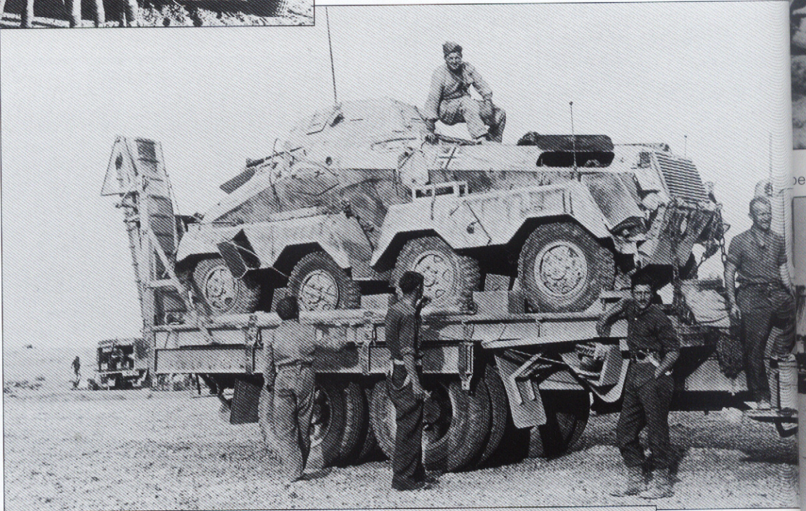
A schwere Panzerspähwagen Sd.Kfz.231 loaded onto a British transport truck for removal. The vehicle is possibly for further evaluation. The yellow camouflage paint is well worn, showing the dark base underneath. Markings are limited to the vehicle registration number plate and the original white outline national cross.
