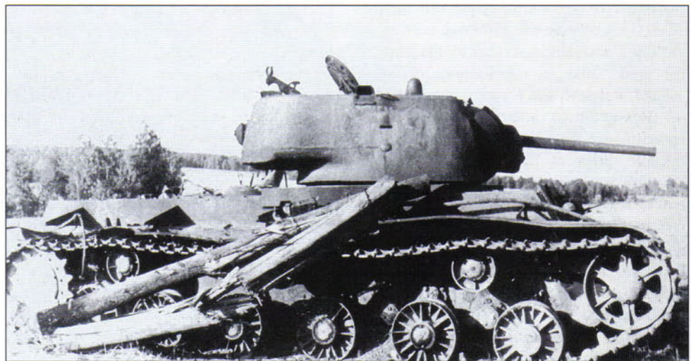
A knocked out KV-1 Model 1942 with the uparmored cast turret. The KV-1 was used with diminishing success in the summer of 1942 during the disastrous tank battles in Ukraine near Voronezh. The new tank corps were badly mauled by the more experienced German panzer divisions. The KV-1 was singled out for criticism as the continual addition of armor to its design without engine improvements led to a tank that was much less mobile than the T-34, and too heavy to cross many rural bridges.
