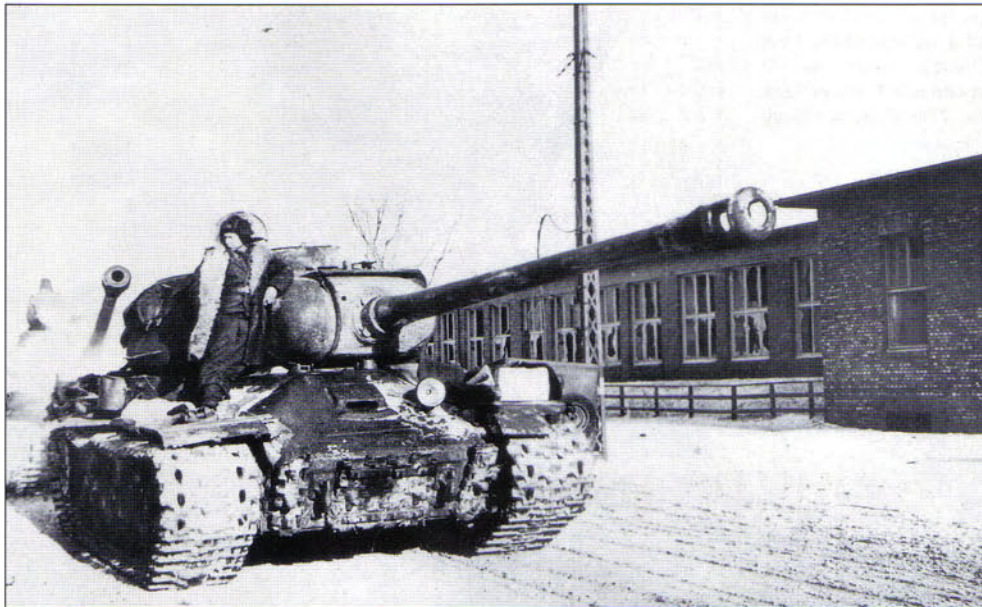
An IS-2m of the 34th Guards Heavy Tank Regiment, commanded by Lt. Col. Mikhail A. Oglobin enters the outskirts of Poznan in western Poland in late February 1945. This unit was supporting the 8th Guards Army during this operation. This is clearly the later IS-2m as it has the new bow casting. (M. Baryatinskiy)
