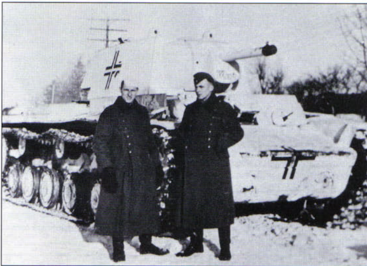
The Wehrmacht captured a number of KV-1 tanks and put them into service in small numbers in the winter of 1941-42. They were always prominently marked with German crosses to prevent misidentification. This KV-1 Model 1941 with the uparmored welded turret has the name "Marta" written in script under the gun barrel on the recuperator housing. (Lee Archer)
