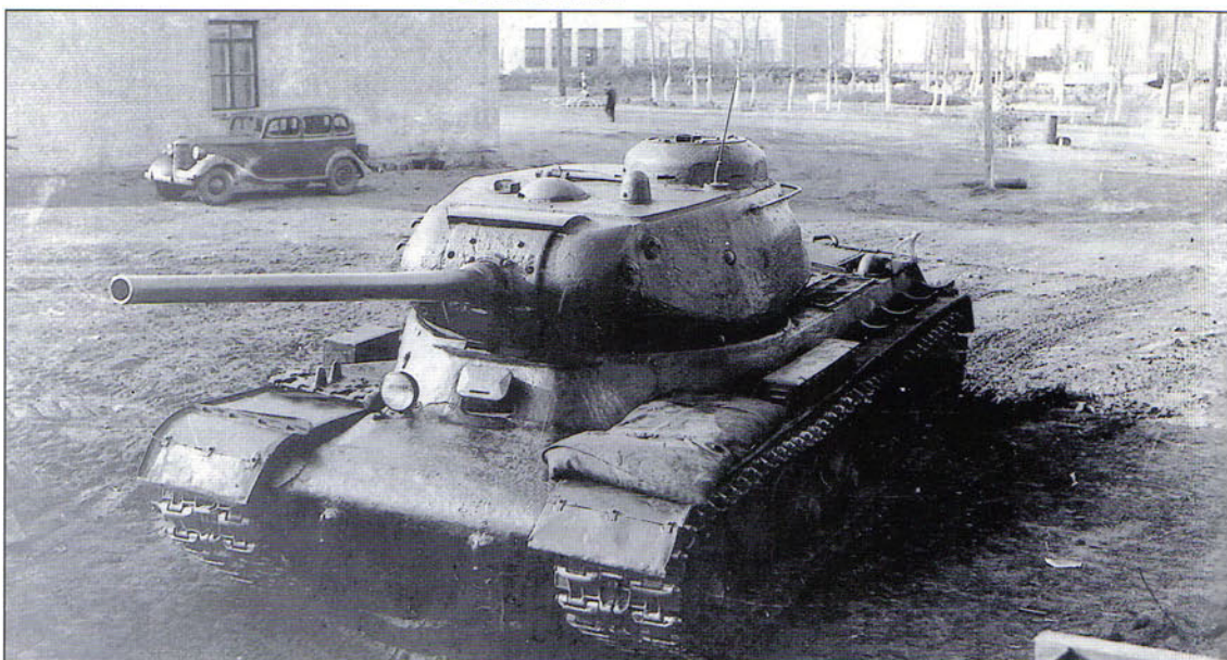
Some KV-85 heavy tanks retained the hull machine gun position as seen here. The KV-85 was used to equip a number of Guards heavy tank regiments in October-November 1943 including the 7th, 11th, 15th and 29th Guards Heavy Tank Regiments. Each regiment normally had a strength of 21 KV-85 tanks.
