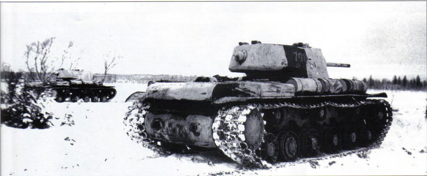
KV-1 Model 1941 tanks go into action on the Kalinin Front in January 1943. The closer tank carries the tactical number 708 and is camouflaged in a pattern of whitewash over patches of the usual dark green. The suspension has at least one of the older style roadwheels due to repair work.
