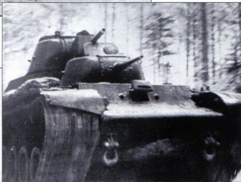
A competitive design for a successor to the T-35 was undertaken in the late 1930s, one of the contenders being the T-100 "Sotka" heavy tank developed by the Barykov design bureau at the Bolshevik plant in Leningrad. The prototype, along with the prototype of the competitive SMK heavy tank design were dispatched for operational trials to Finland in late 1939 with the 20th Armored Brigade. Neither multi-turreted design proved successful, so the Red Army opted for the single turret KV design instead.
