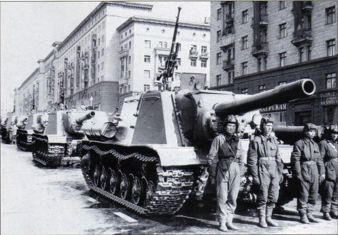
The crew of an ISU-152 await orders to move forward on the streets of Moscow during the 1947 May Victory parade. This is one of the 1945 production vehicles which has the 12.7mm DShK heavy machine gun on the hull roof.
