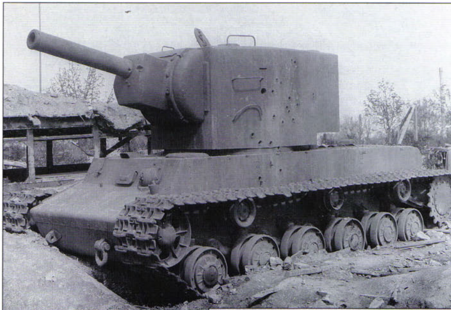
The last combat action of the KV-2 was in German hands when this captured vehicle was used by German troops in April 1945 to set up defenses near the Krupp plant. It has suffered repeated hits on the turret side possibly by 75mm tank gun fire. (US Army)
