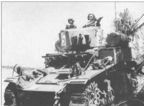
"The Pay-Off", a Marine M3A1 light tank, poses for the camera after landing on Bougainville in the Solomons on 14 November 1943. The two large drums on the rear carry additional fuel. These would usually be dropped before going into combat due to the fire hazard they posed.
