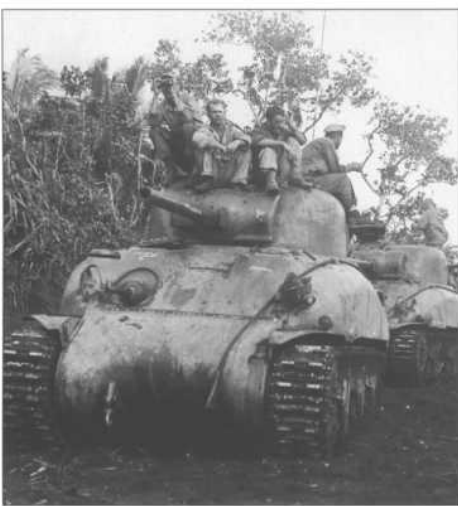
One of the 4th Tank Battalion tanks, "Hunter", was knocked out by Japanese fire during the fighting on Namur in February 1944. A close inspection of the track will reveal grousers attached, a common practice in the sandy soil of the Pacific atolls where the grousers could help improve traction.
