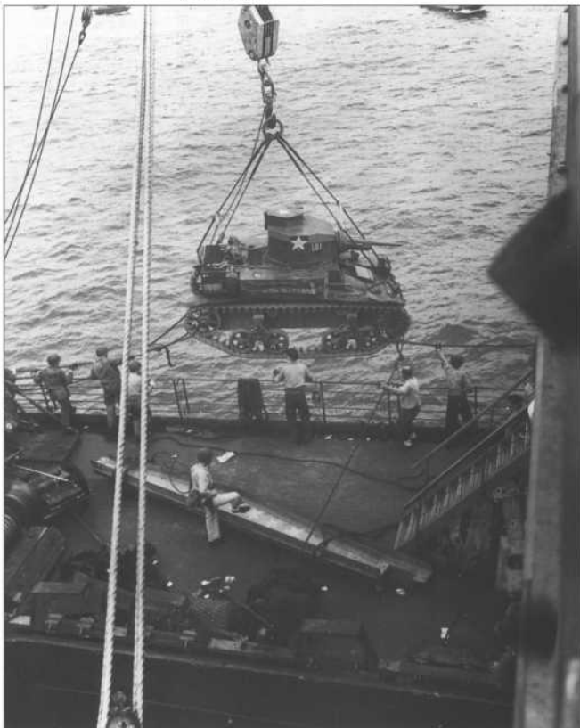
A M3 light tank of the US Marine Corps 1st Tank Battalion during training prior to the Solomons campaign in November 1942 in New Zealand. This M3 light tank is from the later production batches with the round turret and the added rear stowage bins. Notice also that the tank commander wears the early pattern US tanker's helmet with the thick leather band around the rim.
