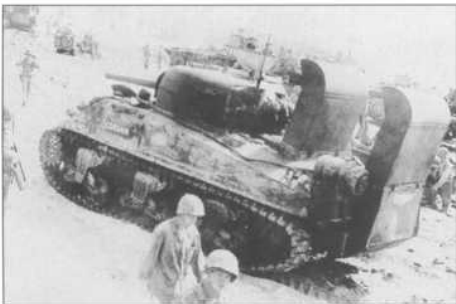
"Corsair", a M4A2 (W) of Co. C, 2nd Marine Tank Battalion, comes ashore at Tinian on 25 July 1944. Tinian was the third of the major islands in the Marshalls attacked by the US forces in July 1944. The Marshalls campaign saw the combat introduction of the late production M4A2 medium tank with the revised 47 degree hull front and wet ammunition stowage. By this stage, the deep fording trunks are becoming more standardized than during previous landing operations. This particular tank appears to have a rough coat of camouflage applied over the hull, possibly with mud.
