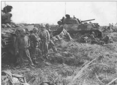
M4A2 (W) medium tanks of the 5th Marine Tank Battalion in a bivouac area on 24 February 1945 on Iwo Jima. This shows the characteristic penny-nail protection on the hatches used by this battalion, as well as the camouflage painting over the side planking. Many Marine tanks on Iwo Jima had a pattern of sand and red brown painted over the normal olive drab.
