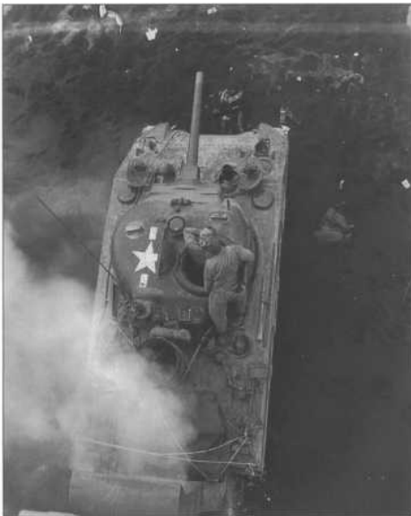
M4A2 (W) medium tanks of the 5th Marine Tank Battalion in a bivouac area on 24 February 1945 on Iwo Jima. This shows the characteristic penny-nail protection on the hatches used by this battalion, as well as the camouflage painting over the side planking. Many Marine tanks on Iwo Jima had a pattern of sand and red brown painted over the normal olive drab.
