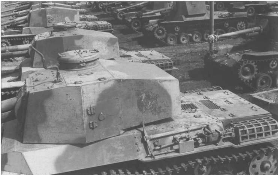
A view of a huge tank park at Hakata, Fukuoka prefecture on Kyushu shortly after the end of the war. In the foreground are some Type 3 Chi-nu medium tanks. Some of the vehicles in the background are the new Type 3 Gun Tank No-ni III, an improved version of the Ho-ni tank destroyer on the Type 97 medium tank chassis, but with a fully armored gun compartment.
