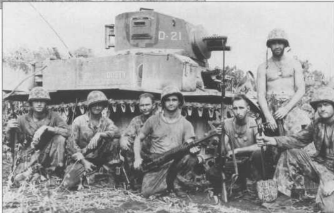
"Dusty", a M3A1 flamethrower tank of Co. D, 2nd Marine Tank Battalion during the Saipan fighting in June 1944. Company D had 12 Satan flamethrowers, which replaced the usual 37mm gun. The general consensus was that the Satan flamethrowers didn't have enough range, and their capacity of 2-minutes of fuel was also deemed inadequate. Two of the Marines display war trophies including a Japanese machine gun and a rifle.
