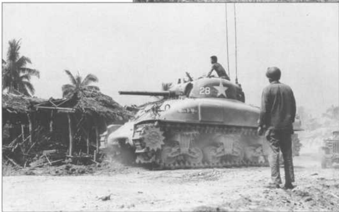
A M4A1 medium tank named "Man O'War" moves through the town of Jualita on 24 October 1944. Notice that the tank has grousers fitted to the track, in an attempt to aid the traction of the smooth rubber block tracks in the frequently encountered mud of Leyte.
