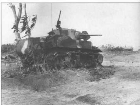
One of the 4th Tank Battalion tanks, "Hunter", was knocked out by Japanese fire during the fighting on Namur in February 1944. A close inspection of the track will reveal grousers attached, a common practice in the sandy soil of the Pacific atolls where the grousers could help improve traction.
