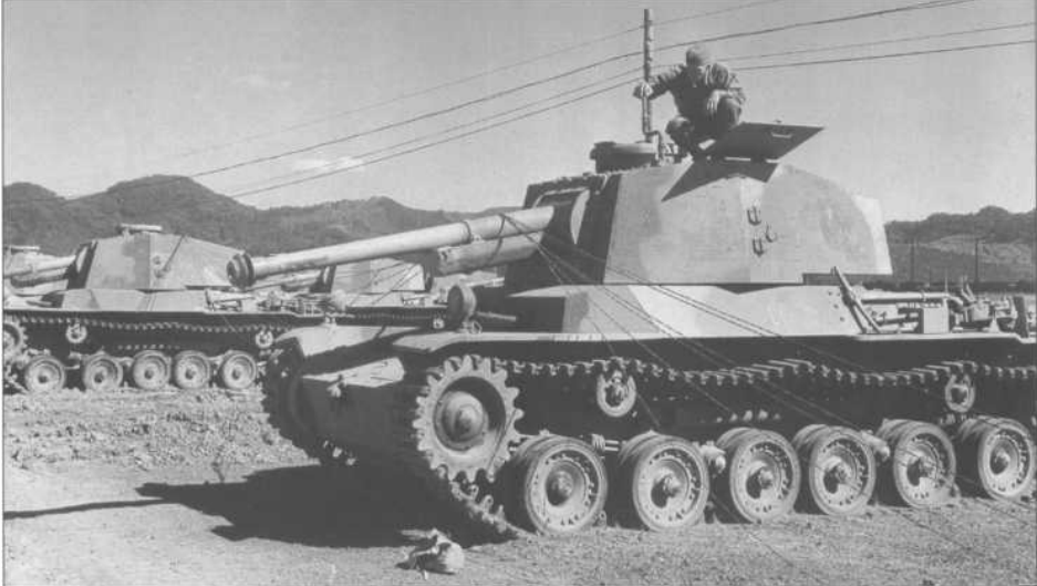
Although the Japanese tanks encountered through most of the Pacific fighting were inferior to the M4 Sherman medium tank, by the end of the war, the Japanese had developed a new and powerful medium tank, the Type 3 Chi-nu armed with a 75mm gun. These were saved for the final defense of the Japanese Home Islands, but ultimately never fired their guns in anger.
