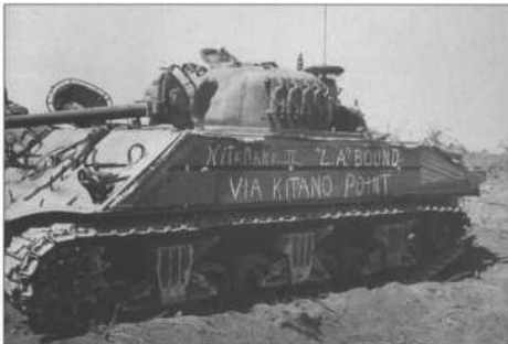
A M4A2 (W) medium tank "Nightmare II", a replacement tank sent to the 5th Tank Battalion on 23 March 1945 shortly before the end of the fighting. On this tank, the protection over the hull hatches is different than the usual 5th Tank Battalion penny nail style.
