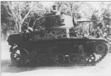
A M3 light tank of the US Marine Corps 1st Tank Battalion during training prior to the Solomons campaign in November 1942 in New Zealand. This M3 light tank is from the later production batches with the round turret and the added rear stowage bins. Notice also that the tank commander wears the early pattern US tanker's helmet with the thick leather band around the rim.
