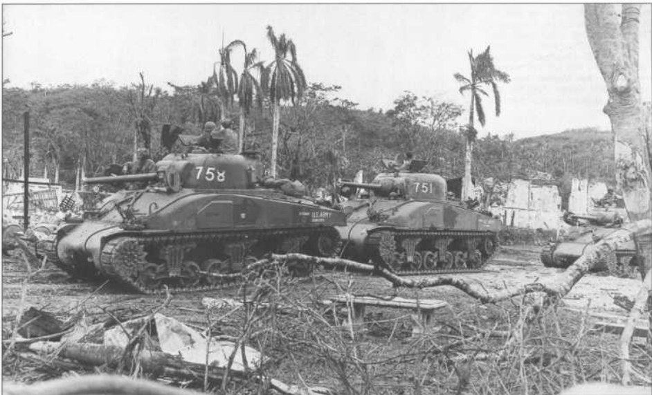
A platoon of composite hull M4 medium tanks of Co. C, 706th Tank Battalion during operations near Agaña on Guam on 2 August 1944. The Guam operation followed the Saipan landings. The composite hull M4 was similar to the basic M4 medium tank, but the hull front was a single casting rather than being constructed of the usual welded plates.
