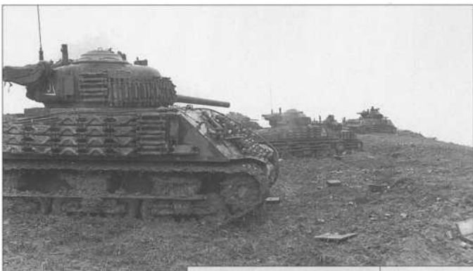
A platoon of M4A2 (W) medium tanks of the Marine 1st Tank Battalion during the fighting near Naha in May 1945. The extensive use of track blocks was intended to protect against anti-tank guns and various types of hand-emplaced anti-tank mines. The suspensions of the tanks were often covered with timber or wood planking to prevent Japanese infantry from striking the thin hull armor with lunge mines or with explosive devices.
