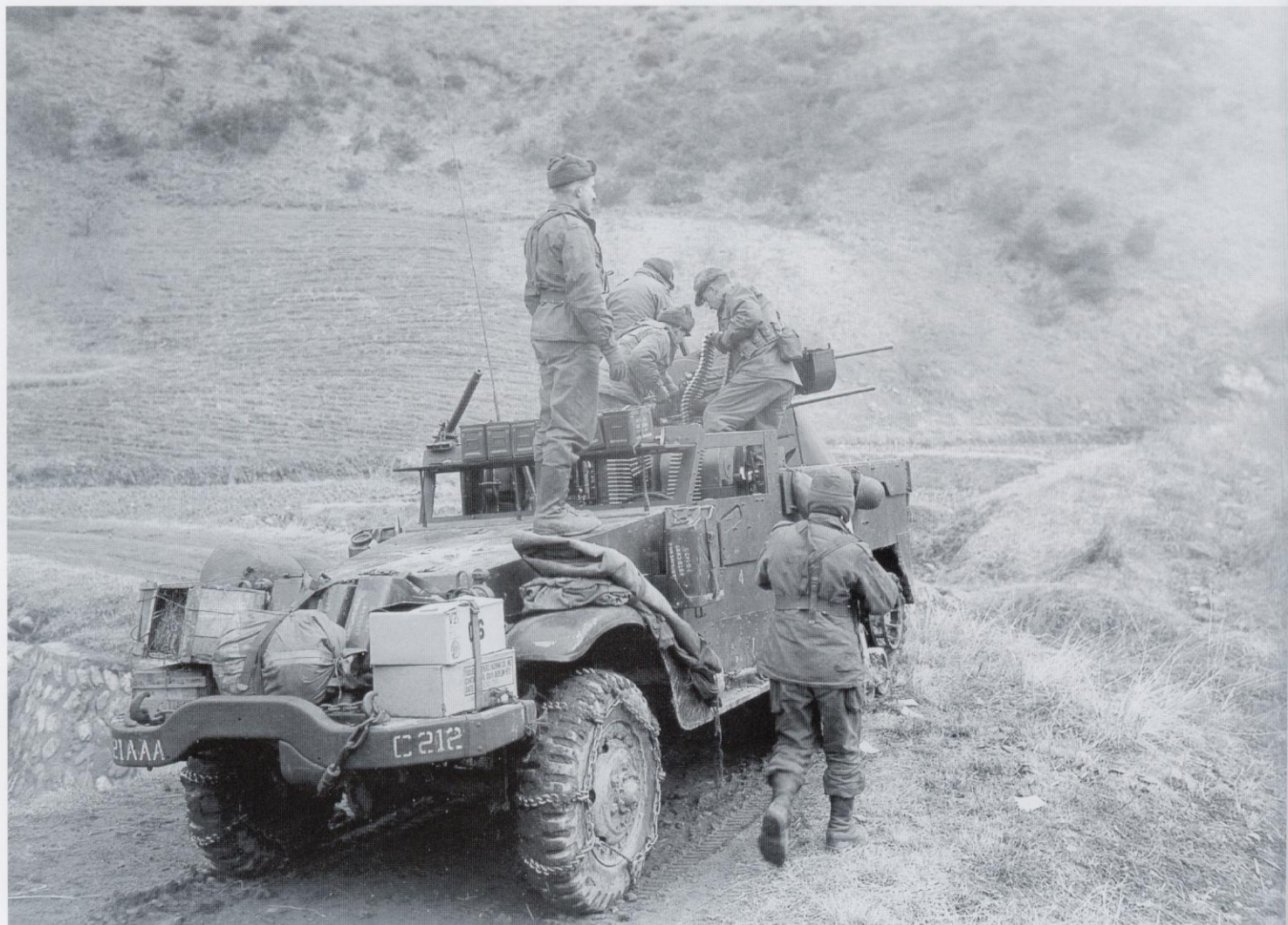
A M16 .50 cal MGMC of the 21st AAA Bn. provides fire support for the 35th Infantry, 25th Infantry Div. during fighting along the 38th Parallel on 10 March 1951. This particular vehicle has the extended winch bumper, and the crew has added a .30 cal Browning machine gun over the right side of the cab.
