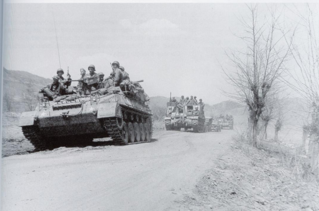
A M37 105mm howitzer motor carriage of the 58th Field Artillery Bn. supports the 3rd Infantry Div. during fighting on the Imjin river on 12 April 1951. The M37 was based on the M24 light tank chassis, and was intended to replace the old M7 105mm HMC on the M4 medium tank chassis.
