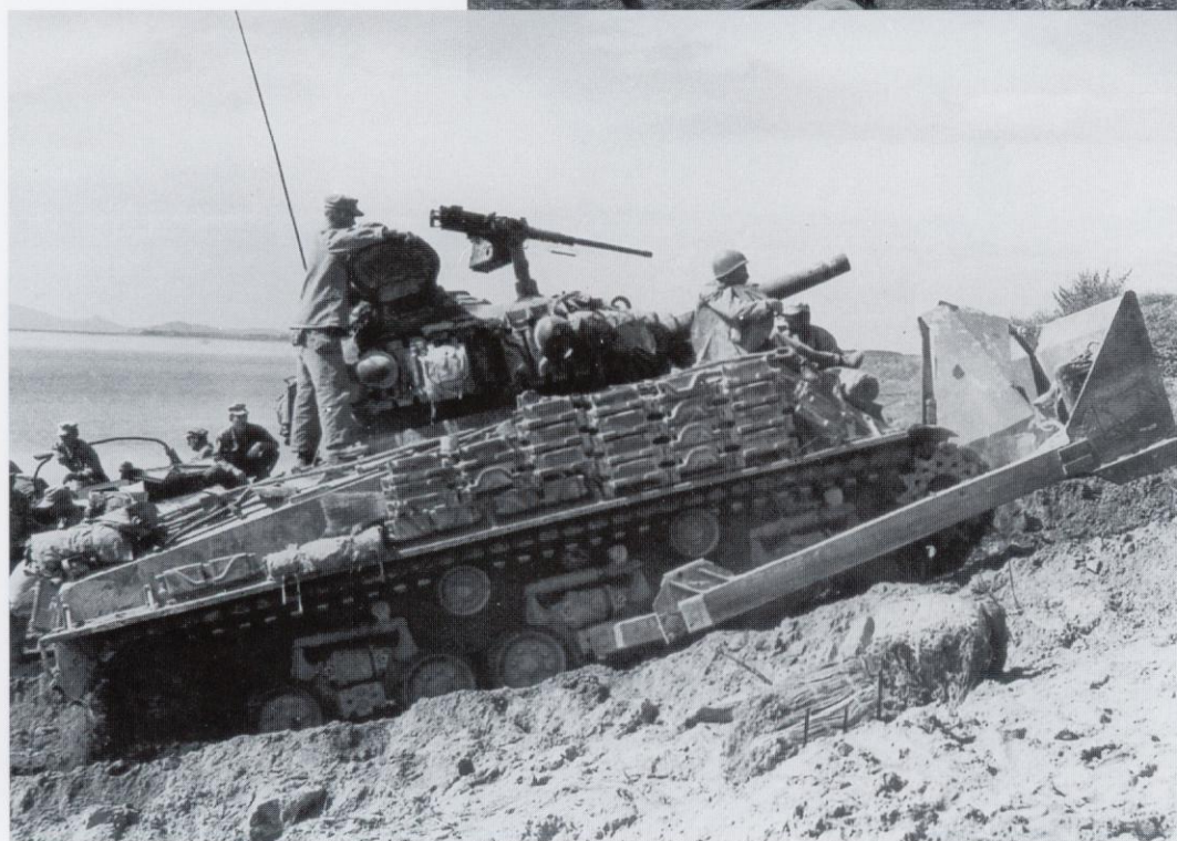
A M4A3 (105) howitzer/dozer is used to prepare approaches for the amtracs on the Kimpo side of the Han river on 20 September. Tanks were ferried over to the Seoul side of the river using bridge sections. The extensive spare track fittings on the side were intended to provide extra armor for the crew.
