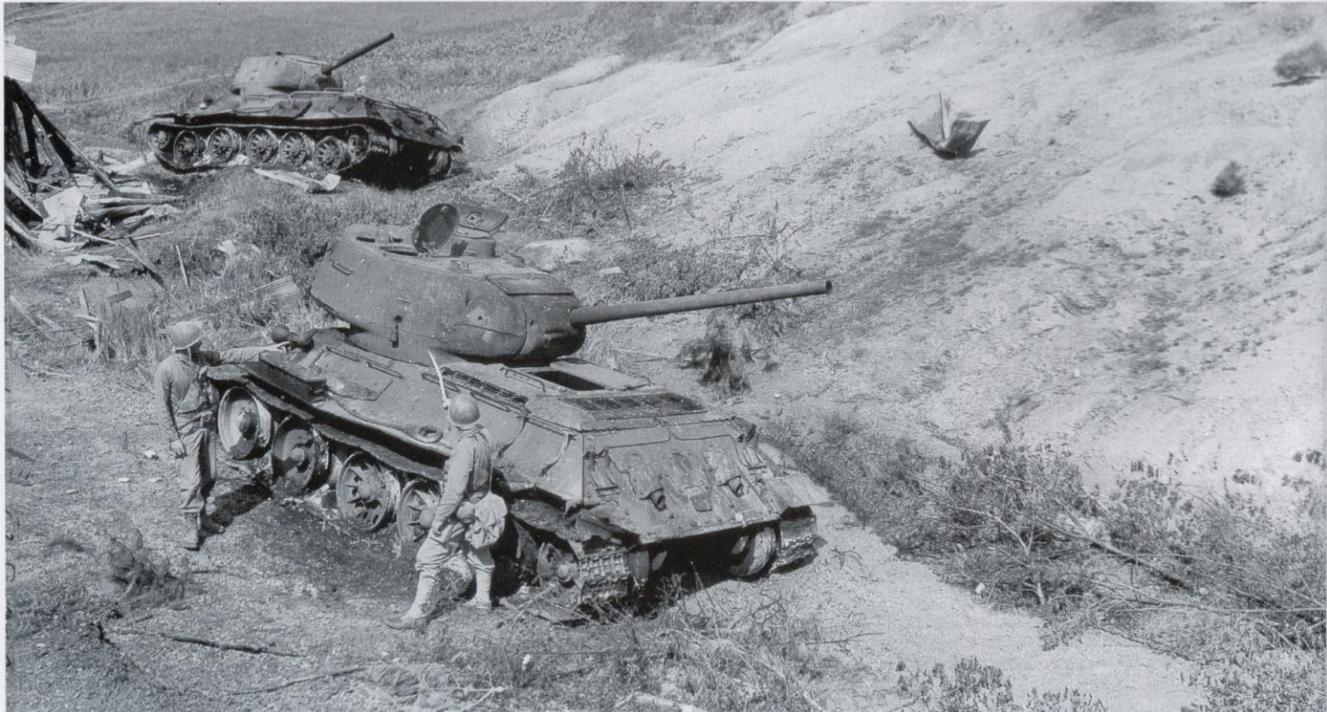
Two T-34-85 tanks of the NKPA 16th Armored Brigade, knocked out by Marine M26 Pershings during fighting near Yongsan on 3-4 September are inspected by Marines of Co. B, 1/5th Marines. The nearest tank has taken a hit on the front side of the turret which evidently led to a vehicle fire which burned the tank out. Notice that the intense heat of the fire has burned the rubber rims off the road-wheels.
