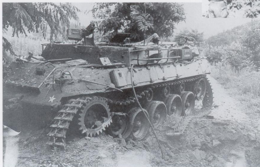
A M39 armored utility vehicle shows the devastating effect an anti-tank mine has on such a light armored vehicle. The drive sprocket and lead road wheel have been shattered by the force of the blast, and the driver was probably seriously injured. This vehicle belonged to Co. A, 89th Tank Bn. and the incident occurred near Chonyon-ni on 8 August 1951.
