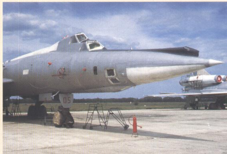
The Tu-22U Blinder-D is a training version with a raised cockpit for the instructor aft of the standard flight deck, and a step-up canopy. (Anatoli Andreyev)
