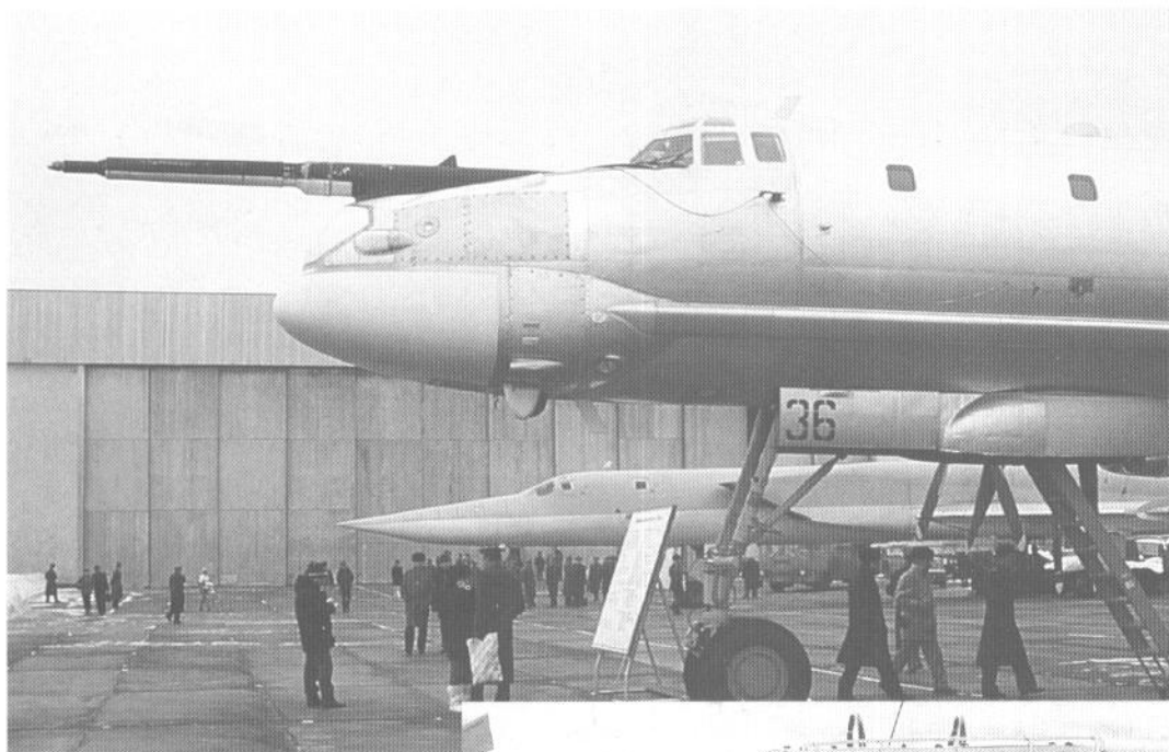
The nose of the Tu-95MS Bear-H aircraft with Short Horn navigation and bombing radar antenna. The in-flight refuelling probe is seen above. (Piotr Butowski)
