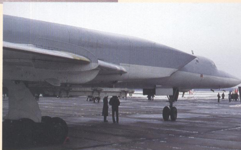
Tu-22M3 Backfire-C is equipped with new Kuznetsov NK-25 engines with increased thrust, therefore the air intakes are bigger, their form being similar as in MiG-25 Foxbat interceptor. (Piotr Butowski)
