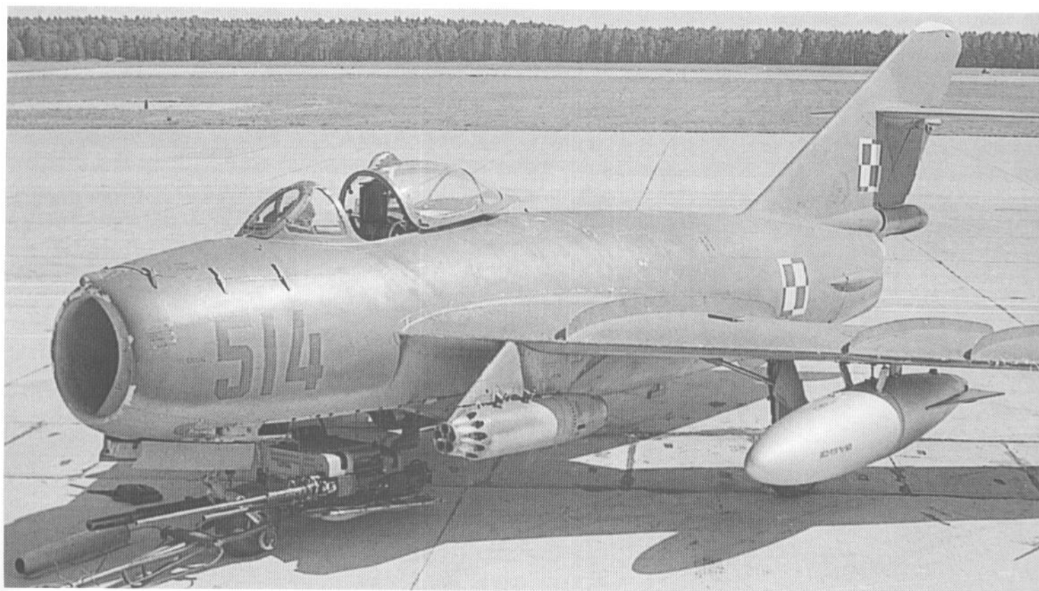
The light attack aircraft Lim-6bis was finally withdrawn from the active service in Polish Air Force in March 1992. Lim-6bis is a Polish-made version of MiG-17 Fresco, used as a light ground attack aircraft. The photo shows the pods under the inboard section of wings (absent in original MiG-17) mounted with UB-16 57mm rocket launchers. (Piotr Butowski)
