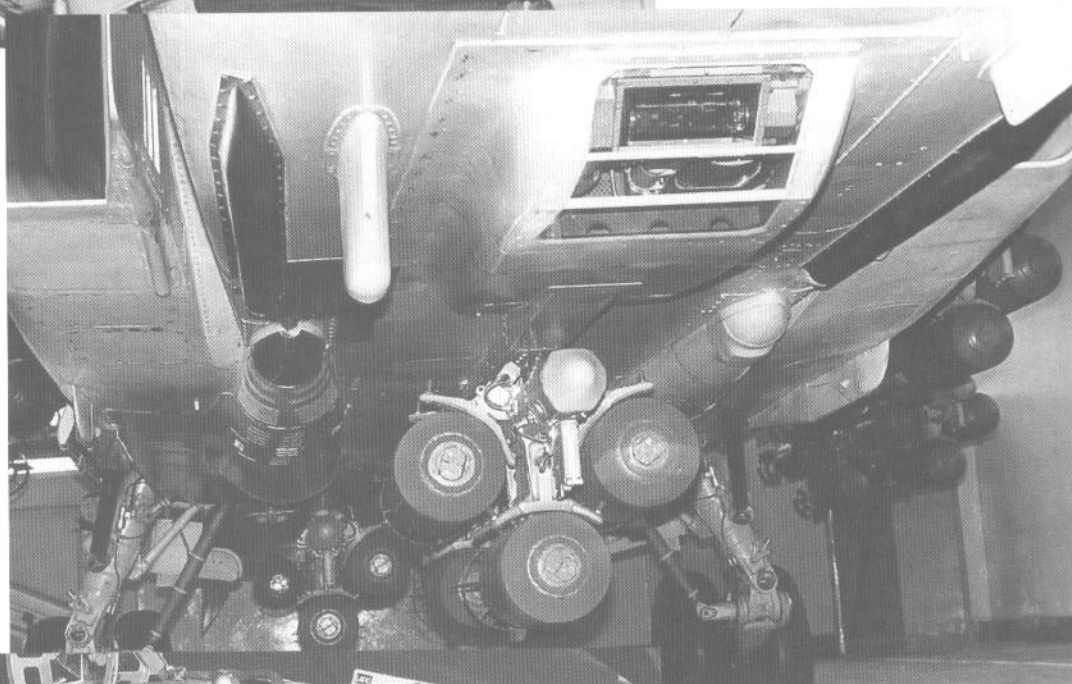
A view of the underside of a Su-24M Fencer-D. The big window of the Kaira-24 LLTV device is seen in the middle section with the bomb-carrying beams behind. There are two identical oblong fairings on both sides. The port-side fairing, with the black mark in the photo, contains a six-barrel Gsh-6-23 cannon. The barrel shutters are opened before firing. The contents of the starboard-side fairing is unknown. (Piotr Butowski)
