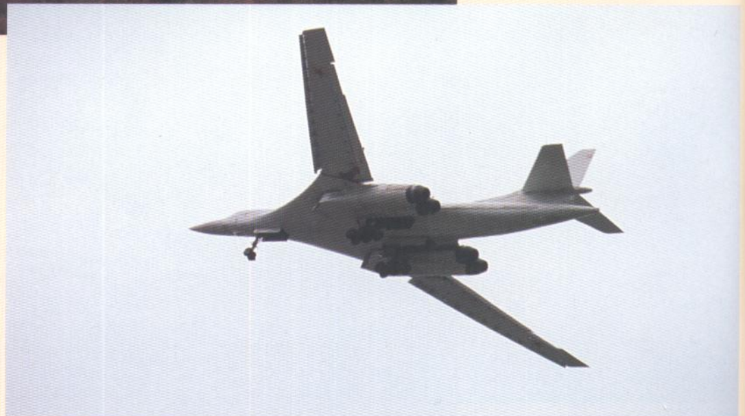
A Tu-160 prior to landing: wing sweep angle set at 20^\circ , and landing gear, flaps and slots lowered. (Piotr Butowski)
