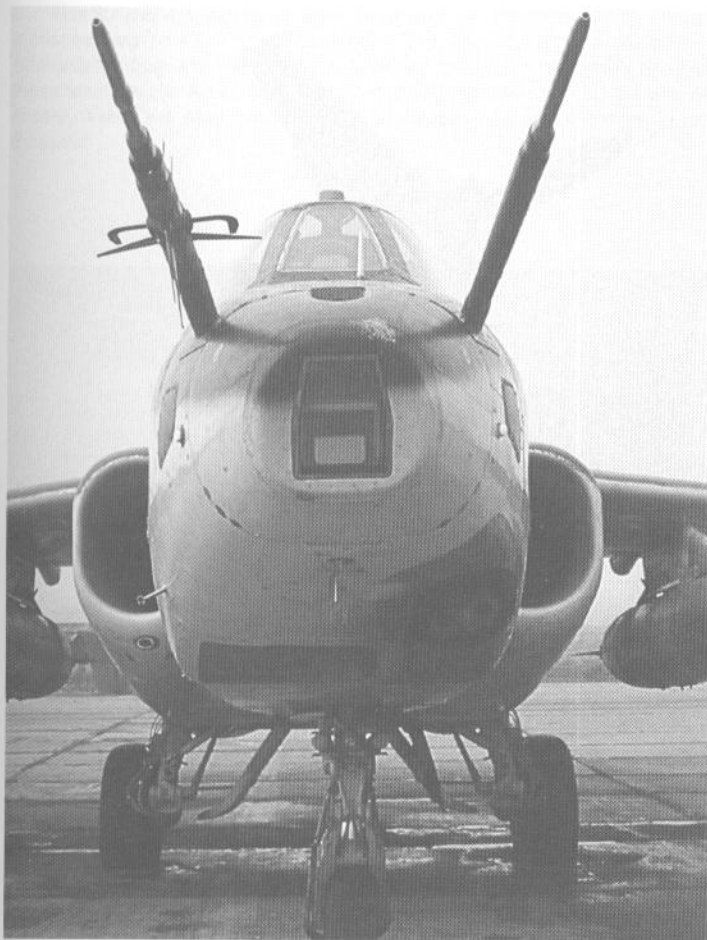
The Klon laser rangefinder and target designator's window in the nose of the Su-25 Frogfoot A. Note the twin-barrel 30mm cannon on the bottom of the front fuselage, on the port side. (Piotr Butowski)
