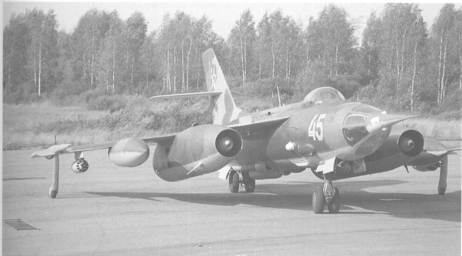
Yak-28PP Brewer-E electronic warfare aircraft. A distinguishing feature of this version is the presence of many aerals on the fuselage. (Piotr Butowski)
