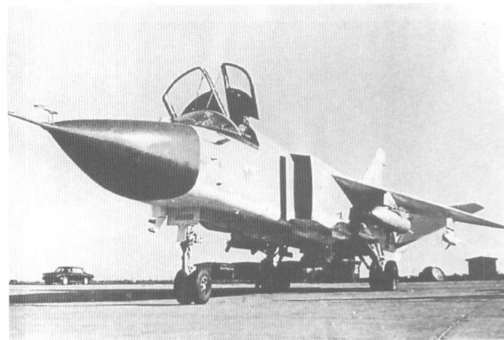
One of the first Su-24 aircraft produced. The air intakes are much larger than in the later aircraft. Also the tip of nose is different. The most interesting, although not very well visible detail is the SPPU-6 gun container suspended from the underwing pylon, which holds a six-barrel GSh-6-23 23mm movable cannon. The computer-controlled cannon can be lowered by about 30°. The photo shows the barrels in the lowered position. (Sukhoi Design Bureau)
