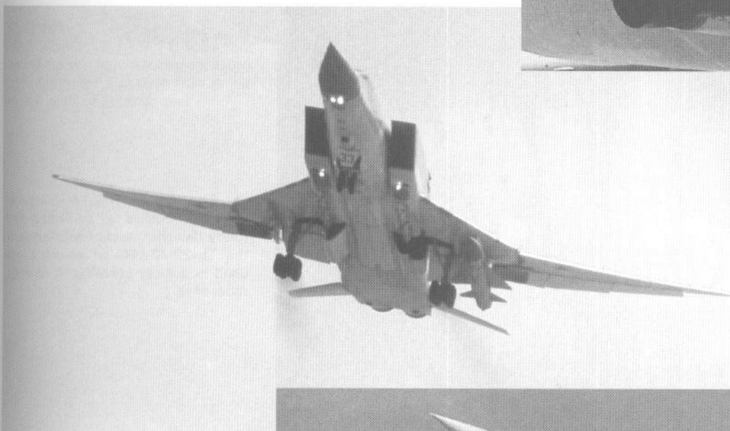
The Tu-22M3 Backfire-C during take-off. Note the Kh-22 (AS-4 Kitchen) missile carried under the port side wing, as well as the multiple weapon racks beneath the intake trunking.
