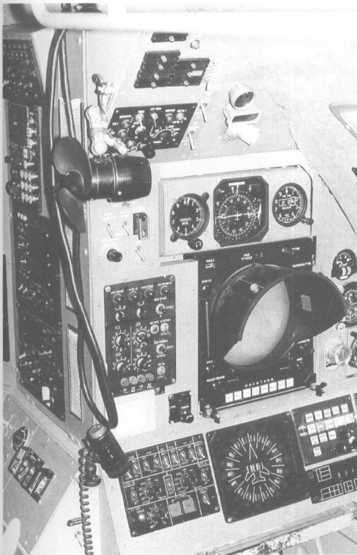
The station of the second navigator who is also the operator of the aircraft's defense system. On the lower console, among other items, are the switches for active electronic jamming, as well as the chaff/flare dispensers controls. (Piotr Butowski)
