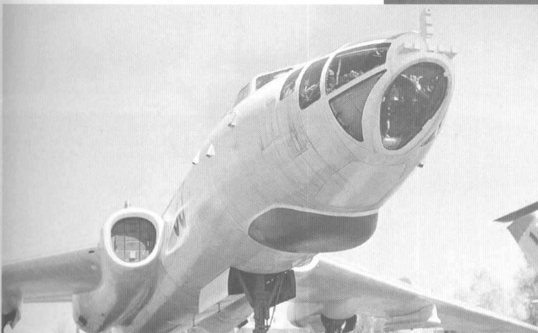
The Tu-16K-26 in a museum in Monino. The RBP-4 (Short Horn) radar antenna is located under the fuselage nose. A small device in the form of an inverted "T" at the aircraft's nose is the antenna of the Ritsa device used for homing KSR-5 missiles ( Ritsa is the name of a lake in Georgia). (Piotr Butowski)
