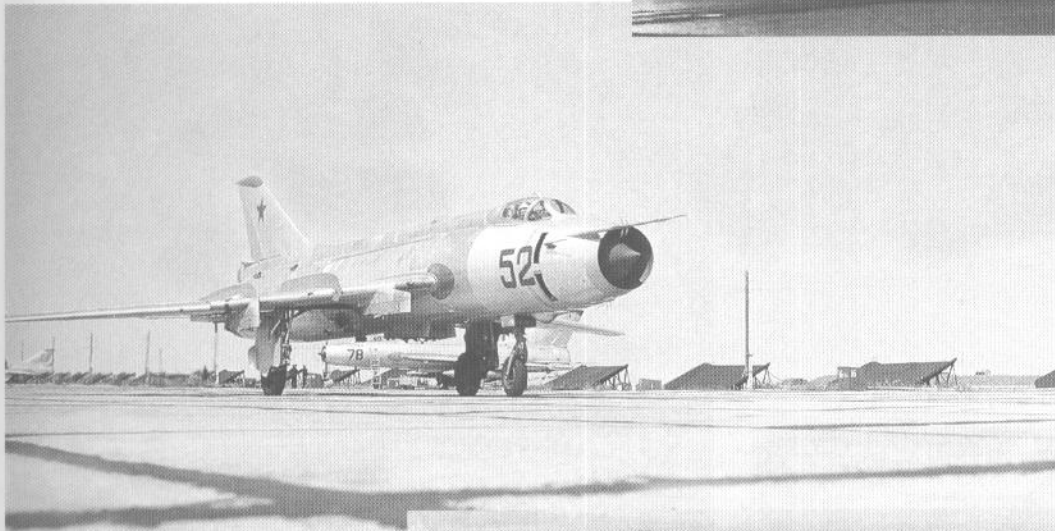
The Su-7 Fitter-A aircraft has been chosen by Sukhoi's team as the basis for the new design, the Su-17 Fitter-B. The wings have been redesigned into a variable geometry model with movable ends. The changes in external appearance include: the cockpit canopy opening upwards instead of sliding back, as in the Su-7; a fairing between the pilot cabin and the tailfin; and some minor changes in the arrangement of aeriels. Also two big armament-carrying beams have been suspended under each wing. In 1972, two Soviet VVS regiments were equipped with the Su-17 aircraft.
