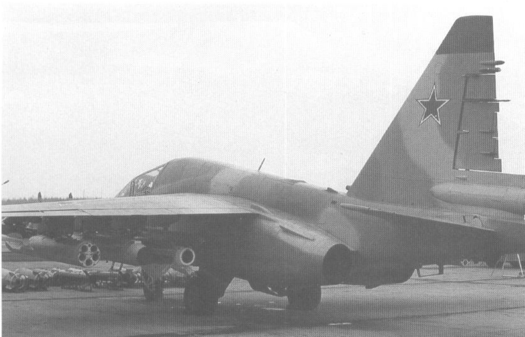
In 1992, the manufacture of the Su-25T begins. Inside the Sukhoi design bureau this version is called the Su-34; with the name Su-25TK it is offered for export. The external appearance of new Su-25T differs from the old Su-25 due to the "hump" on the fuselage behind the cockpit and the large fairing (for the 192-tube chaff/flare dispenser) on the tailfin. Inside the aircraft there is new armament: the Shkval LLTV-system ( shkval for squal) and the Mercuri FLIR pod, used for night attacks. (Dmitri Grinyuk)
