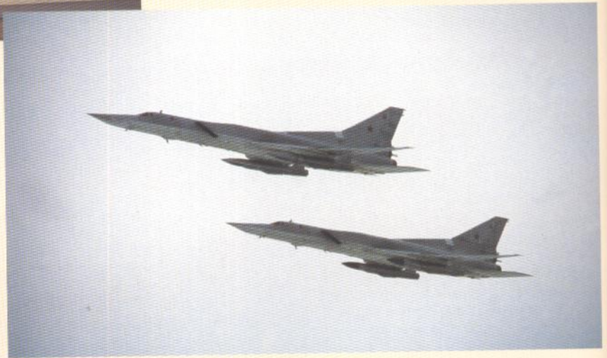
Two Tu-22M3 Backfire-C bombers. Note the different versions of Kh-22 (AS-4 Kitchen) stand-off missiles carried by both aircraft. The first one carries the anti-radar version, while the second one is equipped with missiles with programmable trajectory and an integral navigation system. (Piotr Butowski)
