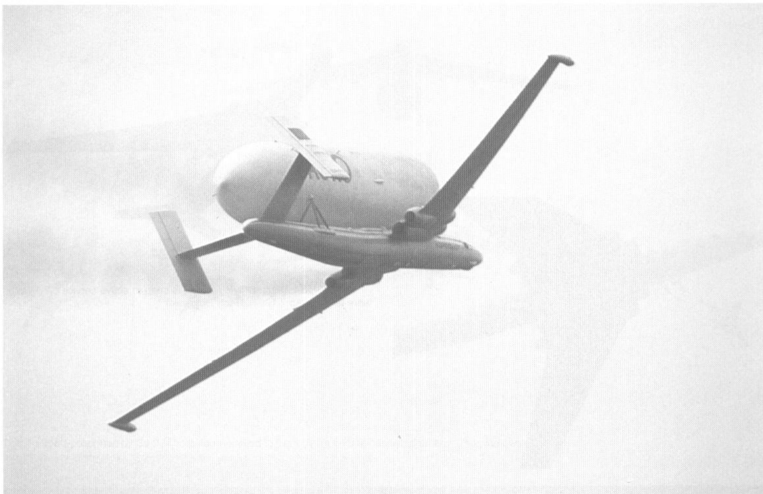
The special modified version of the 3M Bison, the VM-T Atlant, was designed for carrying big and heavy loads. Because of turbulence generated by the load carried on the Atlant fuselage, the classic tail section has been replaced by an H-shaped, double tailfin appendage. (Piotr Butowski)
