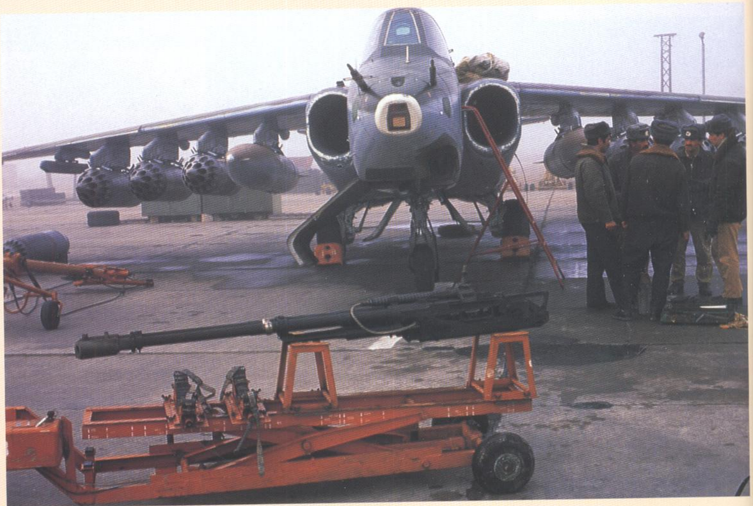
A twin-barrel 30mm cannon dismounted from the fuselage of a Su-25. (Piotr Butowski)
