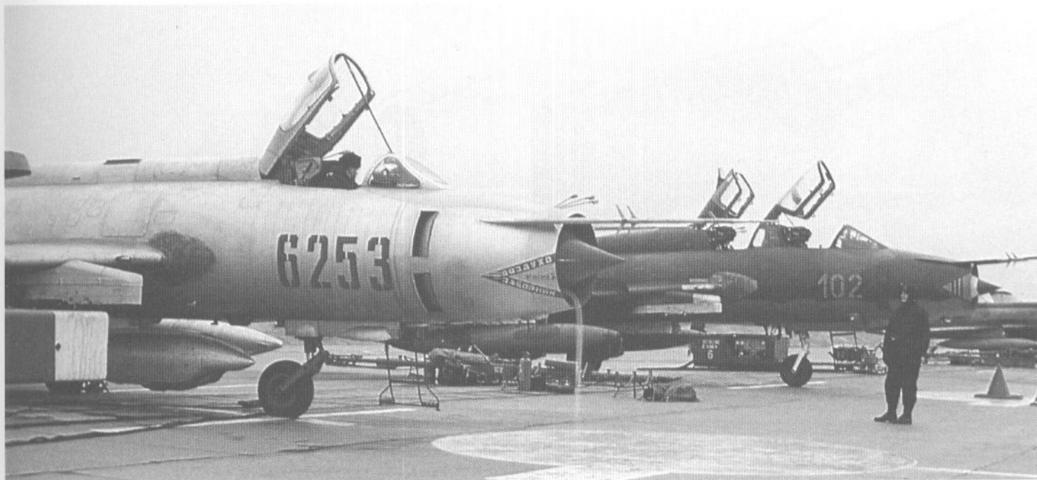
A Su-20R Fitter-C during the engine test prior to take-off on a reconnaissance flight. The thin line entering the air intake is a puddle, left after recent rain, being sucked out. (Piotr Butowski)
