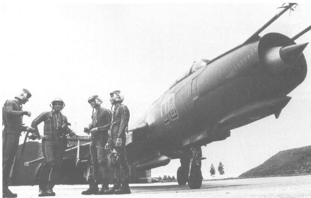
A Su-20R Fitter-C during the engine test prior to take-off on a reconnaissance flight. The thin line entering the air intake is a puddle, left after recent rain, being sucked out. (Piotr Butowski)
