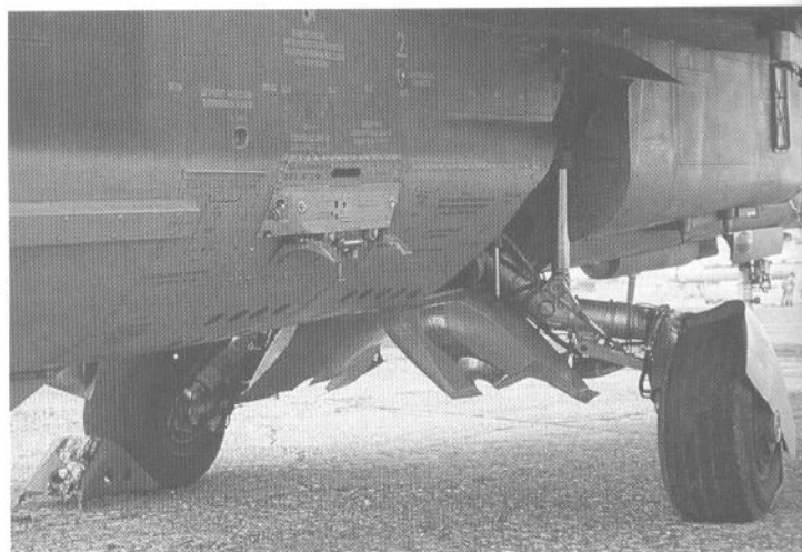
The wide, low-pressure tires of the MiG-27 main wheels allow the aircraft to be operated from unpaved airfields. A catch for the 100kg bomb is visible near the landing gear. (Piotr Butowski)
