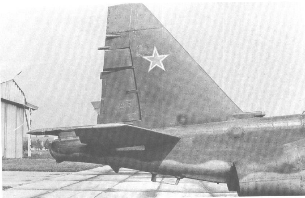
The split rudder of the Su-25 Frogfoot. The small upper rudder section is operated through sensor vanes and transducers on the nose probe, and the automatic electro-mechanical yaw-dumping system. A small air intake for cooling the electronic equipment and cockpit ventilation is seen in the lowest part of the tailfin's leading edge. (Piotr Butowski)
