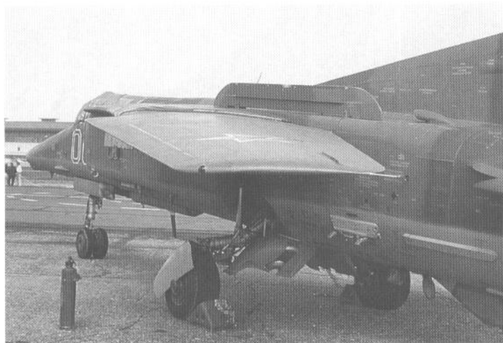
ASO-2 chaff/flare dispensers installed on the back of the MiG-27 fuselage. (Piotr Butowski)
