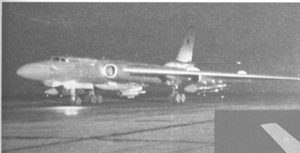
The Tu-16K-11-16 Badger-G, with two KSR-2 (AS-5 Kelt) stand-off missiles beneath the wings, came into service in 1968. The Tu-16K-11-16 is used in naval aviation mainly for attacks against large warships.
