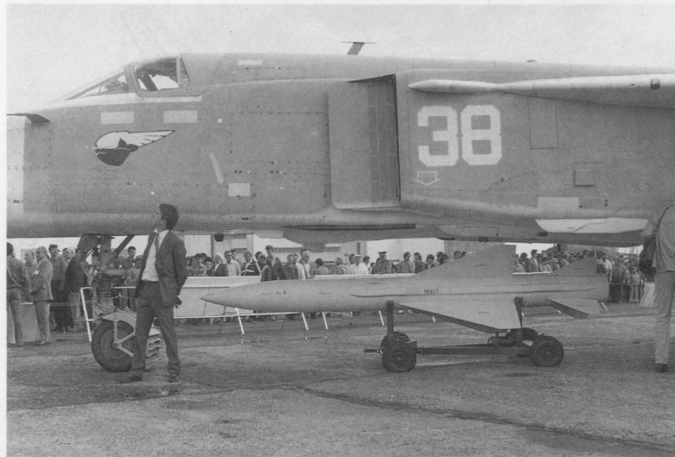
This close-up of the nose shows the AS-11 Kilter missile which arms the Su-24M on anti-radiation missile strikes. It is comparable to the American HARM missile, though significantly larger. Note the Sukhoi production insignia under the cockpit. (Nick Cook)
