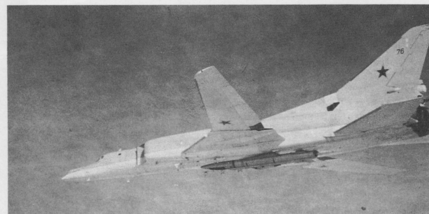
The typical armament of the naval Tu-22M2 is the AS-4 Kitchen (Soviet designation: K-26) anti-ship missile. It can carry one in a recessed bomb bay as seen here, or two on outer wing pylons. Land attack versions of the missile are also employed.
