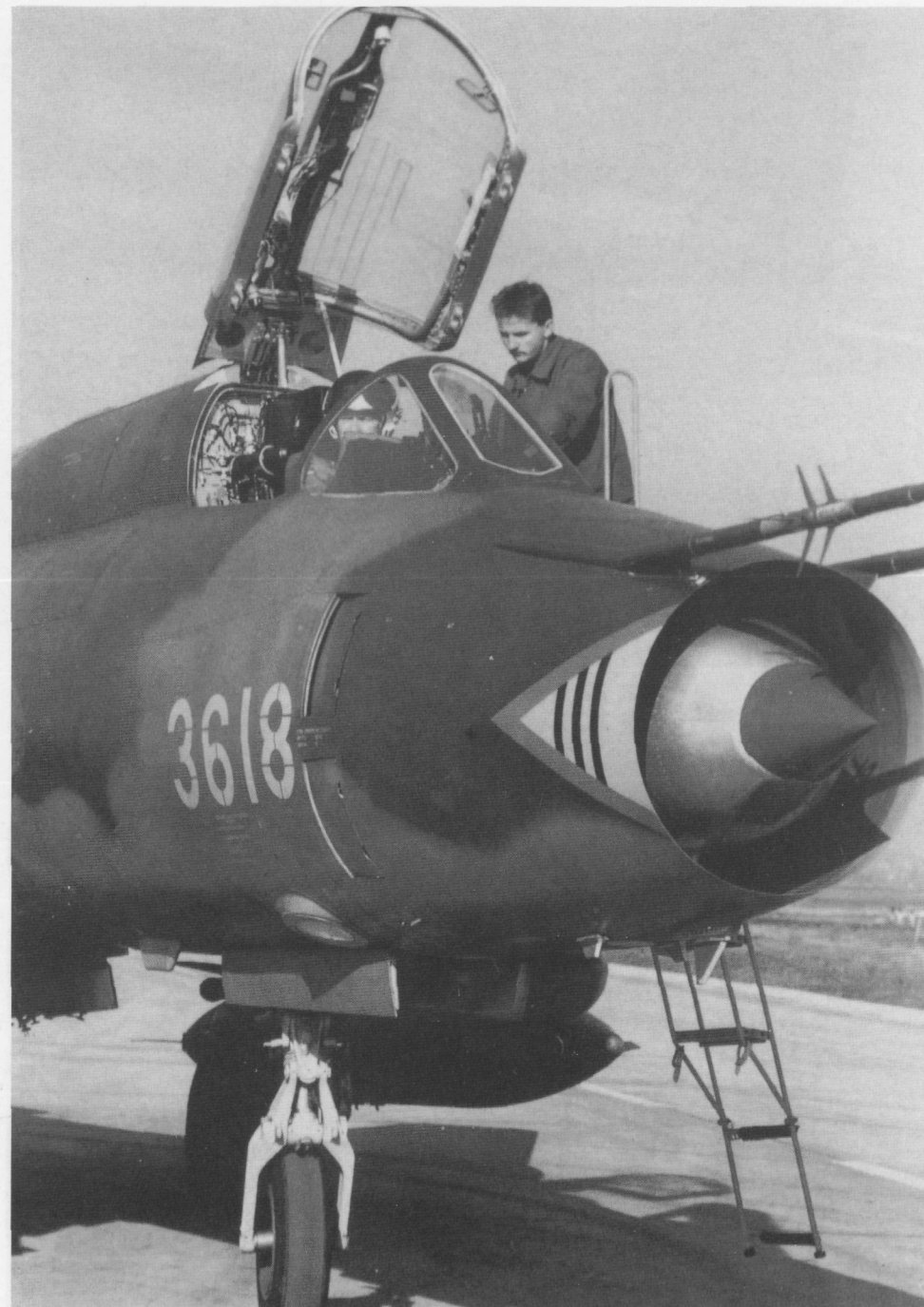
A close-up of the nose of Czechoslovak Su-22M4. These aircraft carry a distinctive yellow-red-black warning area around the air intake.
