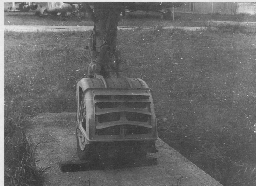
Another detail view of the anti-FOD device on the T-6 prototype at Monino, and similar to that on the current production aircraft.
