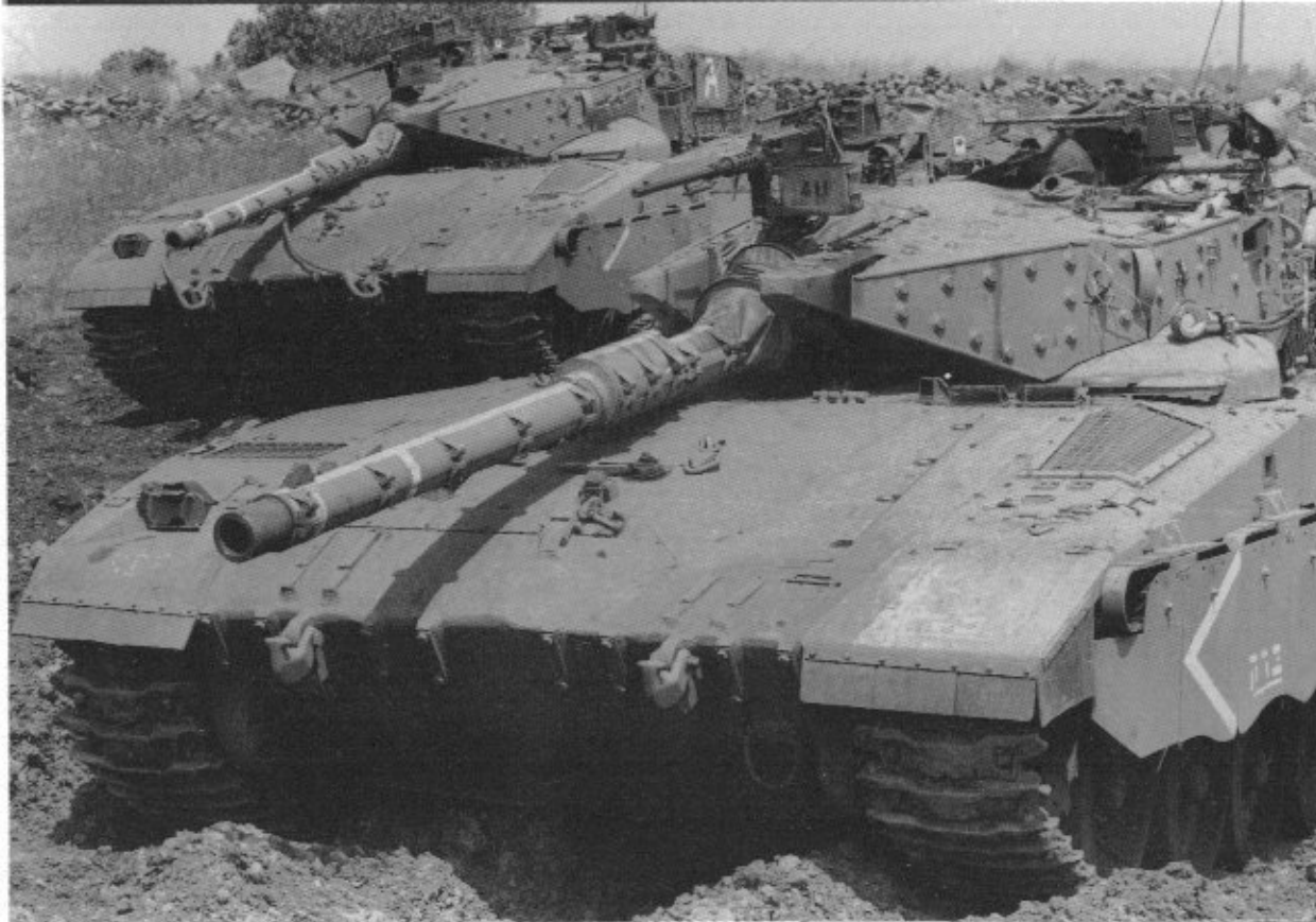
This close-up view of the MERKAVA Mk. II offers an excellent view of the additional armor plating welded to the turret. Note Type 602 ballistic helmet and its FN MAG stock resting place. (IDF Spokesman)
