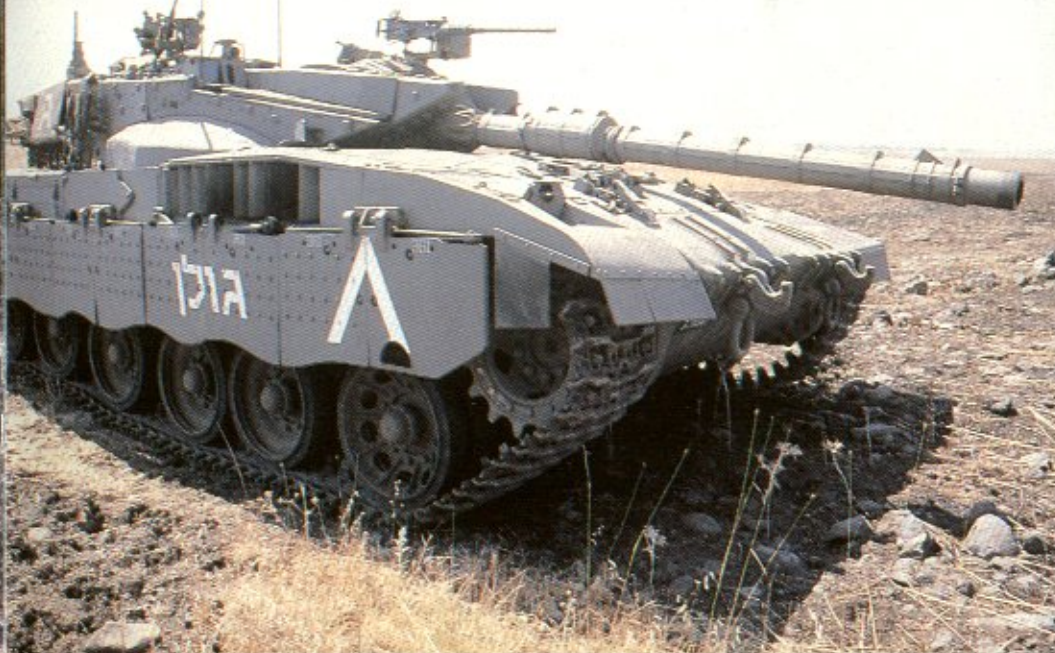
A MERKAVA Mk. II MBT named "Golan" offers an interesting side view of the famed "chariot tank", including heavily armored side skirts, seen here with reinforced welded plates. (IDF Spokesman)
