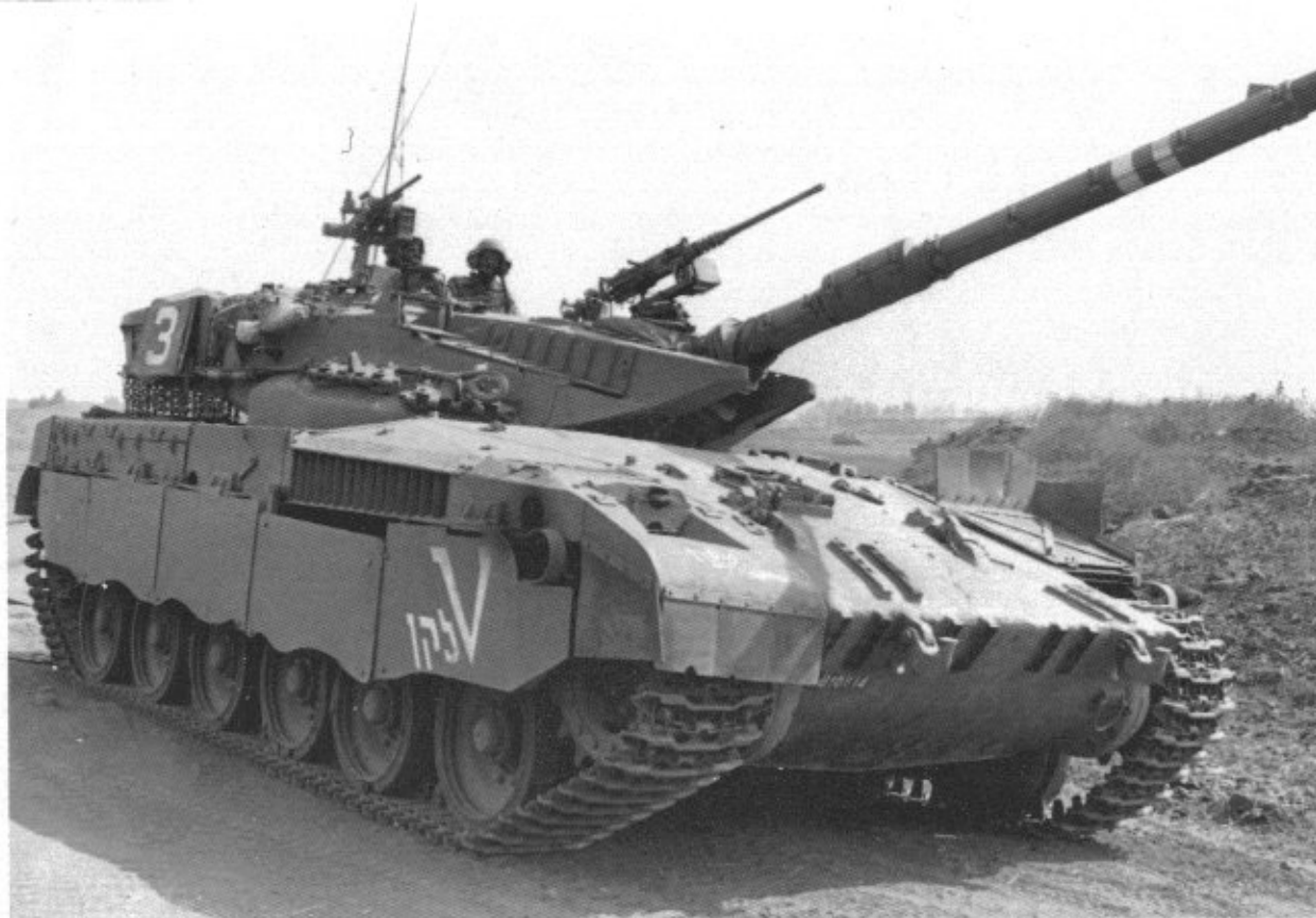
The elevated 105mm gun of this MERKAVA on the Golan Heights allows the turret gun base attachment for the .50 caliber machine gun to be seen to advantage. (Yoni Reif/IDF Spokesman)
