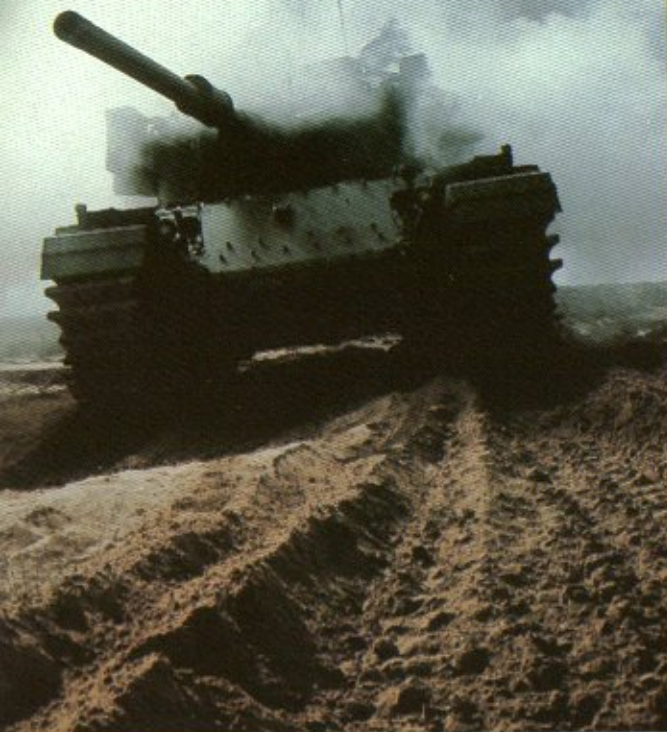
Enveloped in a cloud of smoke and dust, a Centurion continues its advance during live firing training exercises. Note add-on plate of armor attached to glacis plate. (Ofer Karni/IDF Spokesman)
