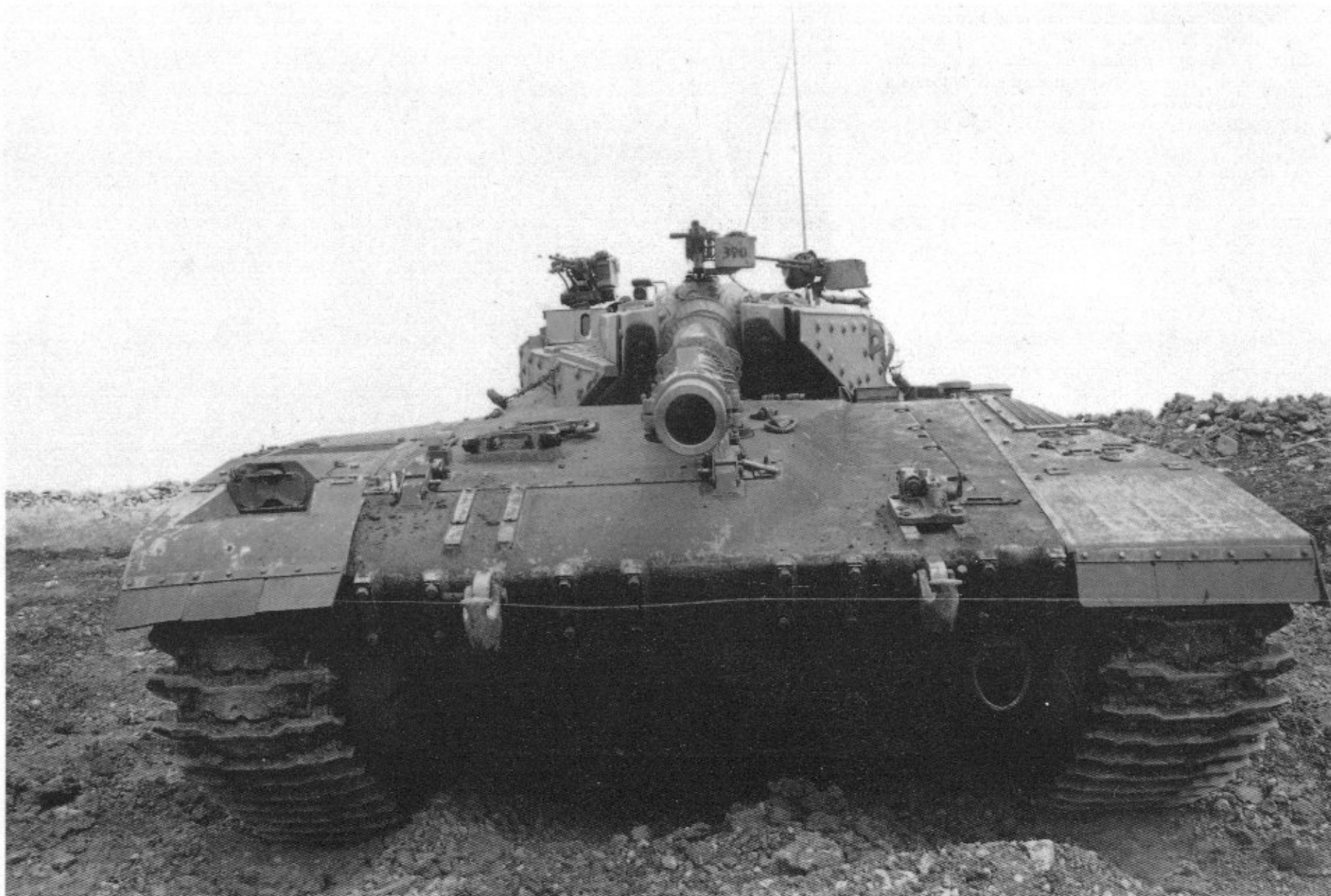
"Go ahead...make my day"! The business end of the MERKAVA 's 105mm gun and low sloped, vertical glacis plates; shown here to advantage. (IDF Spokesman)
