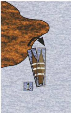
Diagram 11: A grounded ship clearing its bow of the headland.
