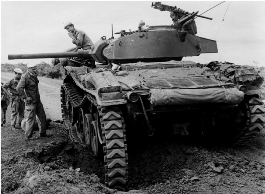
This Chaffee of the Groupe d'Escadrons de Reconnaissance Divisionnaire (GERD) – a formation retained under strategic control in Tonkin – came to grief during an operation north of the Bamboo Canal in the Red River Delta in January 1954. During 1952–54, 398 French AFVs were destroyed, 84 per cent of them by mines and improvised explosive devices. Generally, M24 hulls were rarely ruptured; crew casualties were therefore limited, and maintenance personnel were able to repair the damage relatively quickly – although they were severely hampered by a logistical system that suffered supply delays of six months to a year. In contrast to the M24, other AFVs were often damaged beyond repair or completely destroyed. Once the Viet Minh overcame their psychological fear of tanks they often attacked them with satchel charges at close quarters, irrespective of casualties. (Author's collection)
