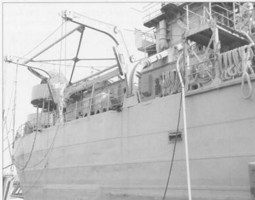
Aft starboard side of LST-325 shows the Welin-type davits in the lowered position. The aft 40mm tubs can be seen behind the davits and the end of the signal bridge in the "V" of the forward davit. The port on the hull is the main engine exhaust vent.
