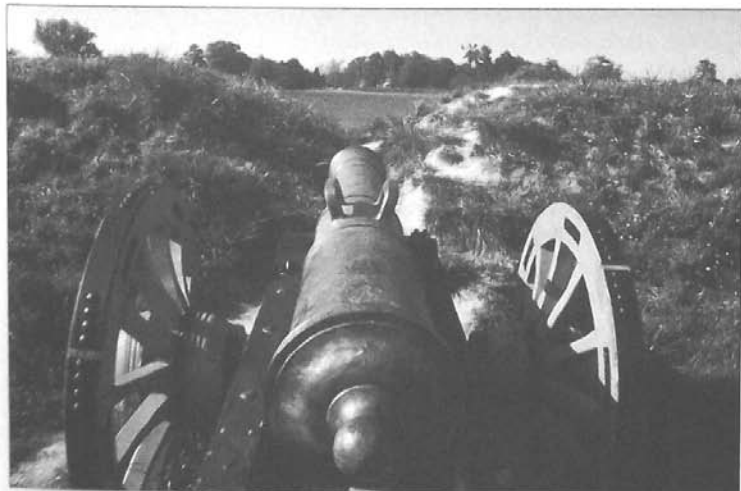
Gribeauval siege 24-pdr from the 1770s. Viewed from the rear. Note that squared 'handles' were also seen on top of the Gribeauval system heavy guns, just as on the field artillery pieces, although the original design plates showed the more Baroque-looking 'dolphins' on top of the brass guns. This replica is located at Yorktown, Virginia. (Photo RC)
