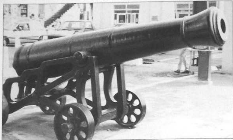
Naval 18-pdr iron model 1778 gun. Note the muzzle casting. This gun, and others like it, were preserved at Plymouth, Montserrat, West Indies. They suffered during the volcanic eruptions of the 1990s when Plymouth was partly covered with ash. (Photo RC)
