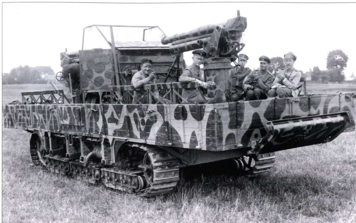
Three chassis were set aside to construct prototypes of the A7V-Flakpanzer, part of a broader effort to develop motorized anti-aircraft batteries. The weapons appear to be captured Russian 76.2mm Model 1902 guns, which have had a new trunnion and elevation assembly added for high-elevation fire. (Thomas Anderson)
