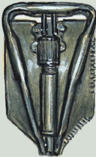
(9) The M1967 collapsible intrenching tool or "tri-fold e-tool." Lighter than earlier models, it was therefore less effective for digging in hard soil, and hacking with the blade locked at 90 degrees was less comfortable.
