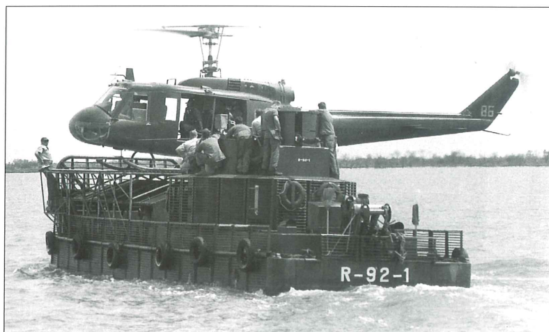
July 1967: this Army UH-1H "slick" from 9th Avn Bn, 9th InfDiv lands on the 16ft square platform added above the troop compartment of a Navy "Tango boat" – Armored Troop Carrier – of River Assault Flotilla One, operating in the Mekong Delta. Initial limited experiments with the "world's smallest aircraft carrier" were followed by a general modification of these boats to ATC (Helicopter) standard. (US Navy, courtesy Simon Dunstan)
