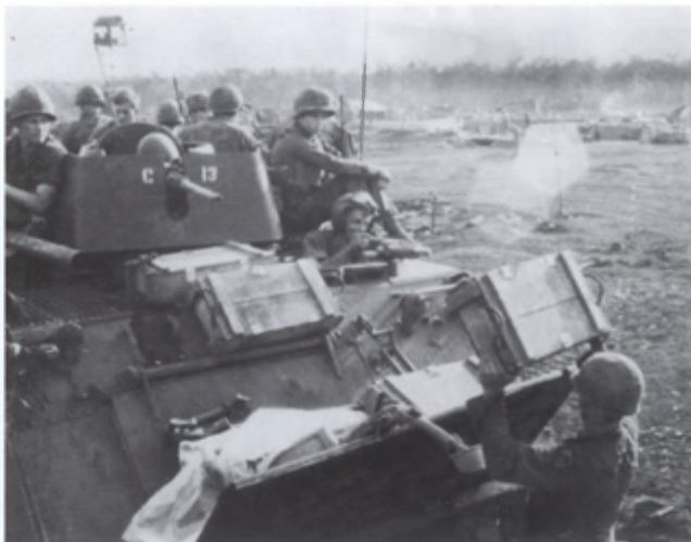
An M113A1 ACAV being prepared for an operation. The infantry ride on top – seemingly in an exposed position, but far safer from mines and RPGs than they would be inside the vehicle. Mechanized units could carry heavier weapons – note the 90mm M67 recoilless rifle visible to the left of the .50cal MG shield. Ammunition crates are being loaded behind the extended bow plane, normally used when “swimming” the vehicle.
