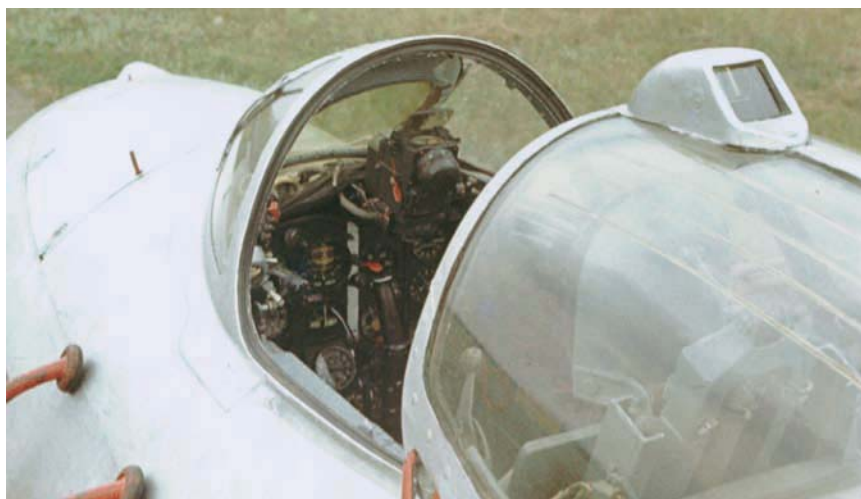
The cluttered MiG-17F cockpit, with its thick windshield frame and ASP-4NM gunsight (linked to an SRD-1 Radal gun-ranging radar) impeding the forward view, rear-view mirror above the canopy and de-icing heating elements embedded in the transparency. (Dr István Toperczer)
