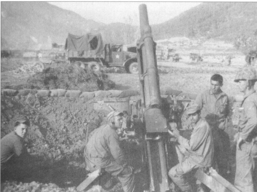
The 11th Marines' 105mm M2A1 howitzer prepares for a fire mission. Three battalions in both marine and Army divisions were armed with this excellent weapon. (USMC)
