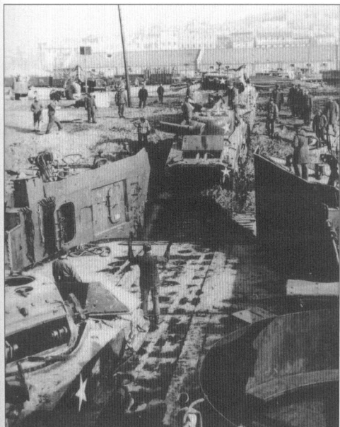
An army M4A3 Sherman tank pushes damaged marine tanks into an LSU for evacuation to Japan and repair. The obsolete Sherman served on in the flamethrower and tank-dozer roles. (USN)
