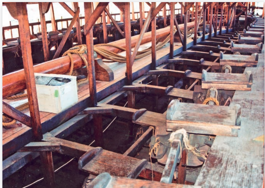
Thranites and zygias 'rowing benches' on Olympias . Note the 'stretchers' for the thranites ' feet and the mast stowed in the central companionway, demonstrating the desirability of having it on shore and out of the way in battle. (Author's collection)
