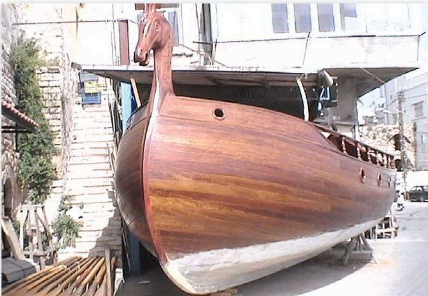
Reconstructed Phoenician merchant ship with cedar planking and rounded prow. (Sanford Holst Phoenicians: Lebanon's Epic Heritage , Cambridge and Boston Press)
