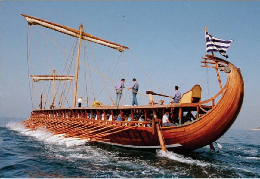
Olympias from one of the best angles for attack, presenting least risk of breaking one's own oars, losing one's ram or becoming locked together on contact. This line of attack called for a sharp burst of speed and for smart manoeuvring and excellent judgement of his collision course on the part of the helmsman. Both thranites and zygios oarsmen and the tightness of the seating arrangements can be clearly seen. (Hellenic Navy)
