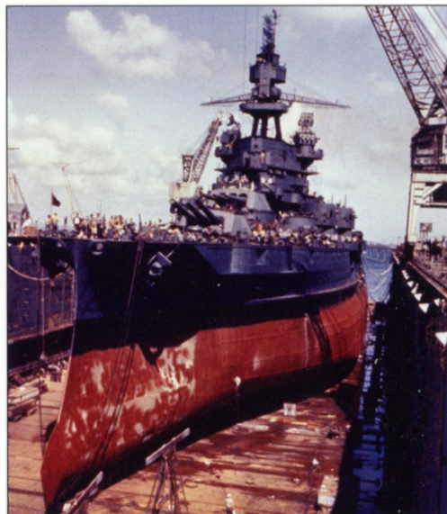
USS Pennsylvania in an Advanced Base Sectional Dock (ABSD) which allowed US naval assets to be re-refitted or repaired in the battle theatre. (NARA)
