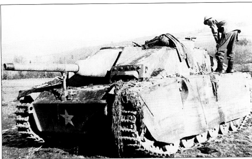
Besides the five Panther tanks converted to resemble M10 tank destroyers, Panzer Brigade 150 also had five Sturmgeschütz III assault guns, painted in American markings, with an ineffective disguise. This one from Kampfgruppe Y was abandoned between Baugnez and Geromont. (NARA)
