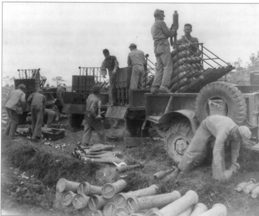
LEFT Each Marine division had a detachment of 12 1-ton truck-mounted 4.5-in. rocket launchers organized into two six-truck sections. The crewmen were called "Buck Rogers Men" after a contemporary science fiction hero. Each truck, nicknamed a "Sandy Andy" after a popular toy, mounted three Mk 7 launcher racks with each holding 12 rockets. They could fire 36 high explosive and white phosphorus rockets in four seconds to a range of 1,100 yds (1,006 m). (USMC)
