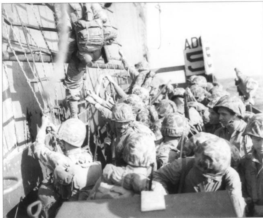
Troops of the 1st Mar. Div. board a landing craft, vehicle and personnel (LCVP) alongside an assault transport on the morning of L-Day. Rather than the rope cargo nets used earlier, these men have the benefit of more stable chain and wooden rung ladders. An LCVP, the most used landing craft, could carry 36 troops or a 6,000-lb (2,722-kg) vehicle or 8,100 lb (3,674 kg) of cargo. The 35-ft 9-in. (11-m) craft were armed with two .30cal. M1919A4 machine guns. (USMC)
