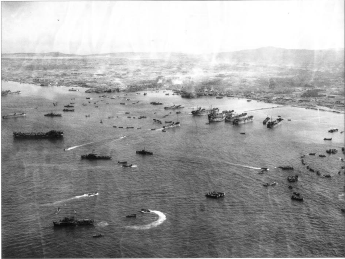
This aerial view of the beachhead on L4 gives some idea of the logistical effort required to sustain a landing force ashore. Six Landing Ships, Tank (LST) are off-loading at center right of the picture. The reef prevents them from grounding closer to shore. The small bay above and to the left of the LSTs is the mouth of the Bishi Gawa (Stream). (USMC)
