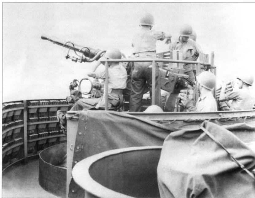
A twin 40-mm anti-aircraft gun mounted on an unidentified type of landing ship. The 40-mm Bofors was mounted on virtually all ships in either single, twin, or quad mountings (the latter two being liquid-cooled) for anti-aircraft defense, which was essential at Okinawa because of the unrelenting Kamikaze attacks. Landing ships operating close inshore used anti-aircraft guns to place suppressive fire on shore targets. Scores of four-round clips line the gun tub. (USMC)
