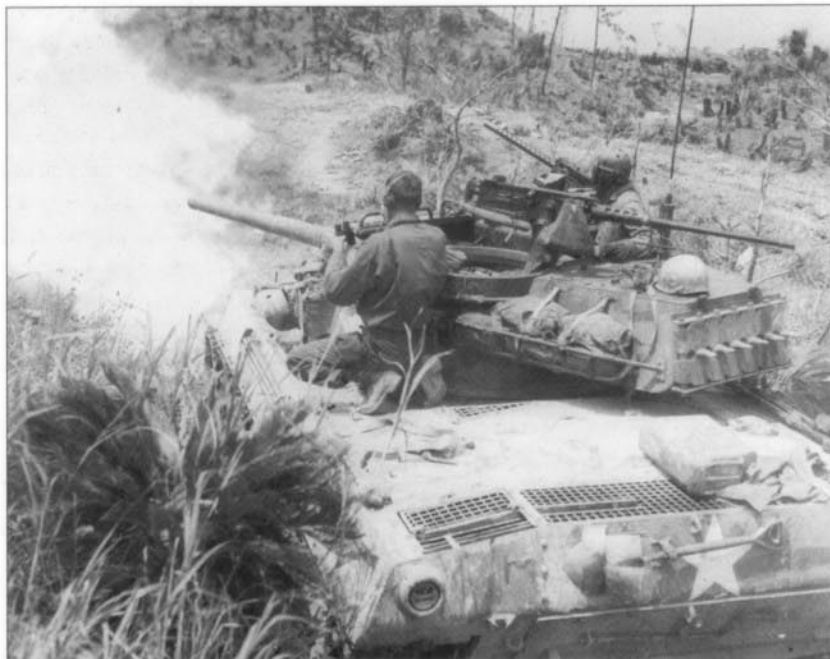
A 76-mm gun-armed M18 "Hellcat" tank destroyer of the Antitank Company, 306th Infantry, 77th Inf. Div. fires on the Shuri Line, 11 May. Atop the turret are .50cal. HB-M2 and .30cal. M1919A4 machine guns. Note the crew's haversacks in the turret bustle rack and the spare treads on the turret rear. (US Army)
