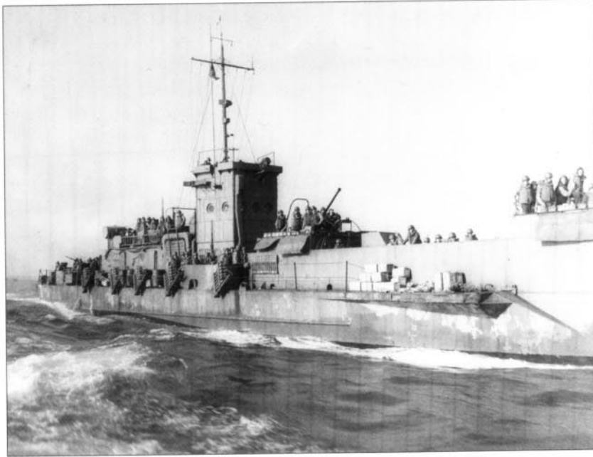
A landing craft, infantry (gun) (LCI[G]) type D. It mounts five 4.5-in. Mk 7 rocket launchers on either side along with three 40-mm and four 20-mm guns. Each Mk 7 launcher rack holds 12 high explosive rockets with a range of 1,100 yds (1,006 m). These craft preceded the assault waves toward shore firing suppressive barrages. Three of the same Mk 7 launcher racks were mounted on Marine 1-ton trucks. (USMC)
