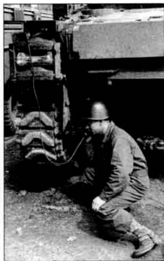
One of the lessons from the bocage fighting was the need for better tank-infantry cooperation. A simple but effective innovation introduced before Cobra was the installation of a telephone mounted in a .30cal ammunition box on the rear of the tank, wired to the tank's internal intercom system. This allowed accompanying infantry to talk to the tank crew and help coordinate their actions.
