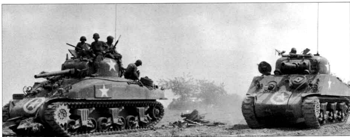
The 7th Armored Division surged past the cathedral city of Chartres on 16 August. The M4A1 from the 31st Tank Battalion on the left is fitted with a Rhino, while the M4 (105mm) assault gun to the right is not.
