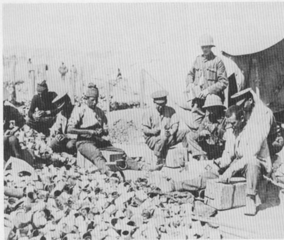
◀ Manufacturing hand-grenades: empty tin cans are converted to 'jam tin bombs'. The man at extreme right is using an anvil upon which to cut up lengths of barbed wire to pack into the tins to act as shrapnel.
