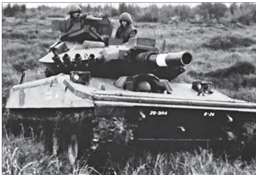
Armored cavalry units began replacing their Patton tanks with the M551 Sheridan armored reconnaissance airborne assault vehicle in late 1967. It was armed with a 152mm gun.
