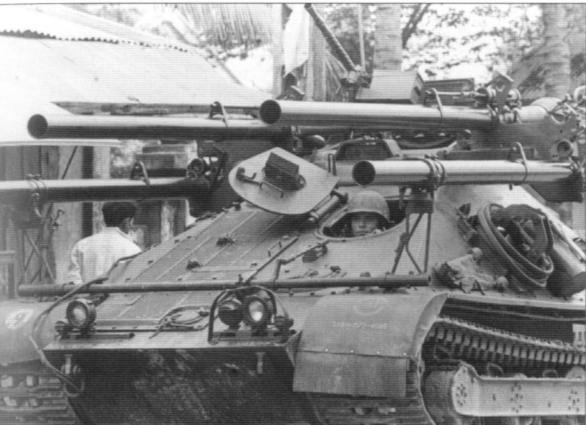
The light M50 Ontos tank destroyer packed considerable firepower in its six 106mm recoilless guns (only four are fitted to this one), but its thin armor made it vulnerable even to small-arms fire at close ranges. (NARA)
