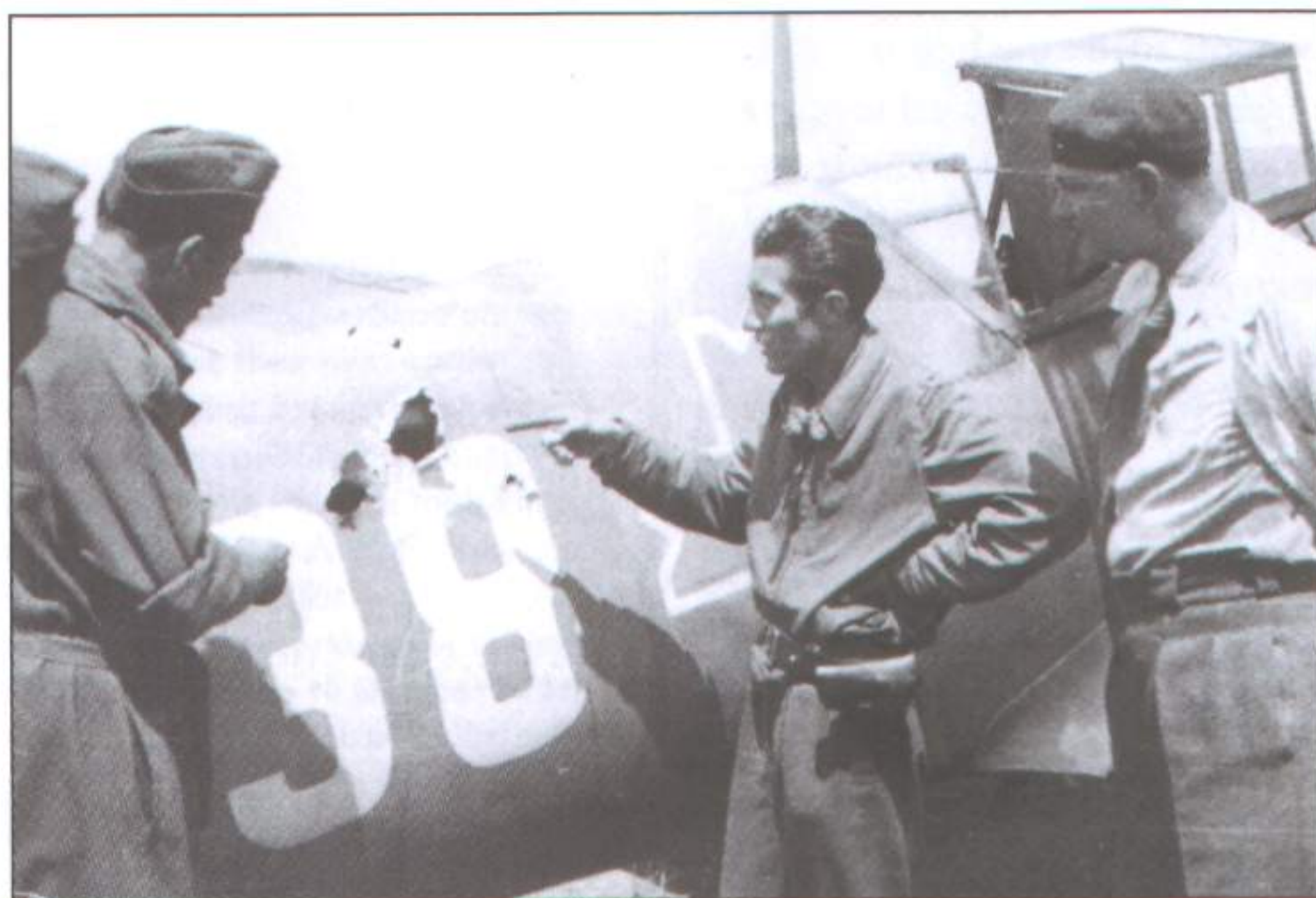
Slt rez av Ioan Di Cesare of Grupul 7 vânătoare shows engineer Lt mec Serban Diaconu the damage to his Messerschmitt ('White 38' Wk-Nr. 13845) after a dogfight with Soviet fighters which were obviously armed with both machine guns and cannon. 'White 38' later suffered 30 per cent damage from Soviet flak while being flown by Adj av Constantin Ursache on 21 July 1943, the fighter in turn being handed back to the Germans for repairs to be effected
