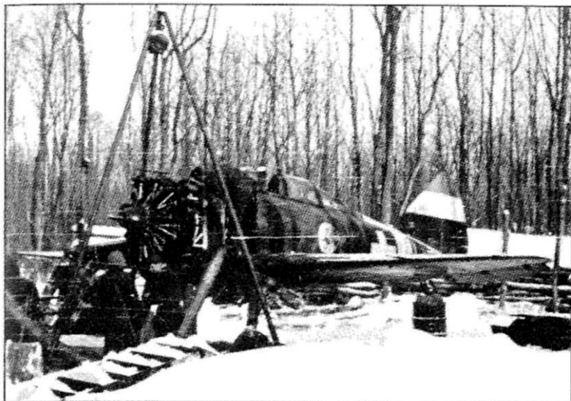
Graphically illustrating the primitive conditions confronting groundcrews during the winter of 1942-43, an Re.2000 has its Piaggio P.XI engine changed at Ilovskoje. The Reggiane's radial powerplant proved to be a mechanical nightmare 'in-the-field' (Terry via Punka)
