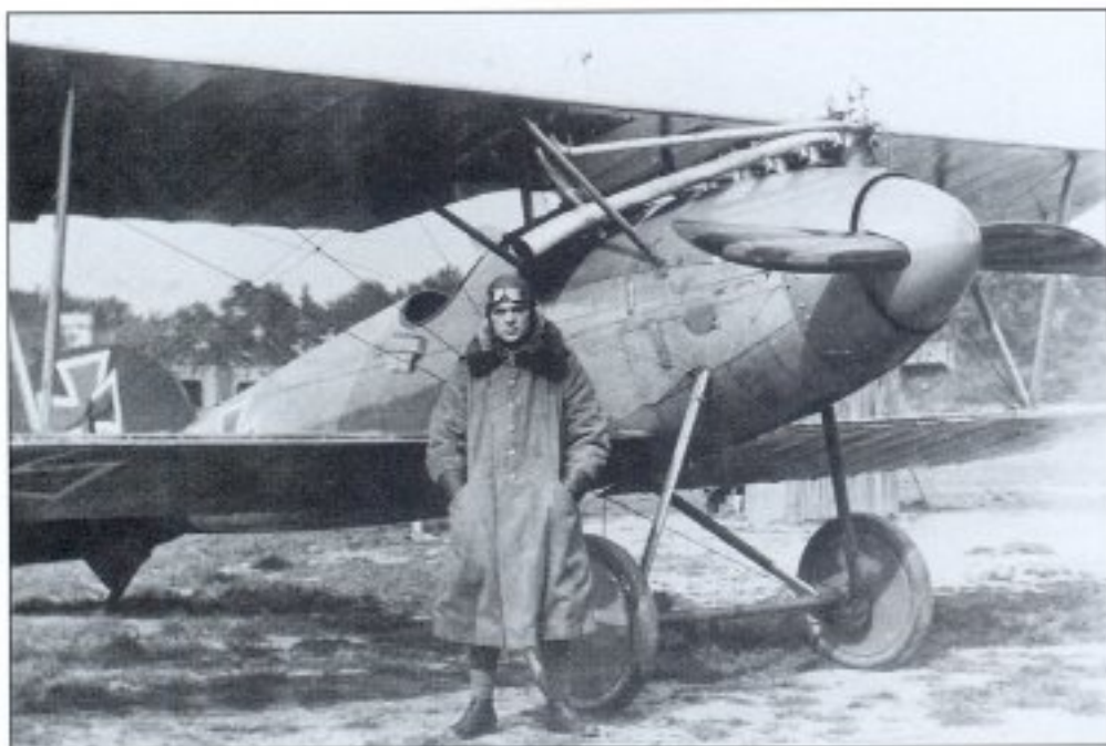
Jasta 17's leading ace, Julius Buckler, wears a full-length greatcoat with fur collar in this view taken at Wasquehal airfield in the autumn of 1917. The dark-painted tail (black?) was the unit marking at this time. Buckler's usual Mops insignia is not to be seen – the wings were covered in five-colour 'lozenge' fabric. Note the rack of signal cartridges mounted below the cockpit (HAC/UTD)
