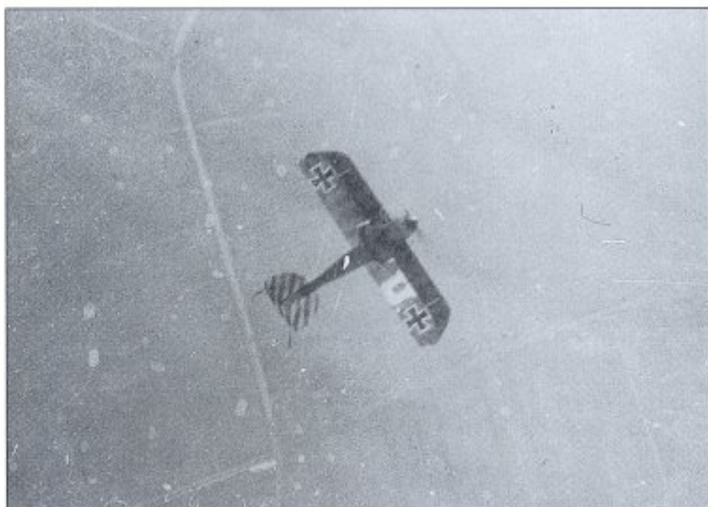
This remarkable photograph, taken from above Ernst Udet as he looped his black Albatros D Va, reveals the underside markings of his fighter. Udet used his 'U' initial in place of the numbers which the other Jasta 37 aircraft displayed on their lower wings. Such markings on the wing undersides were meant to facilitate aircraft identification and confirmation of victory claims by ground observers (A Imrie)
