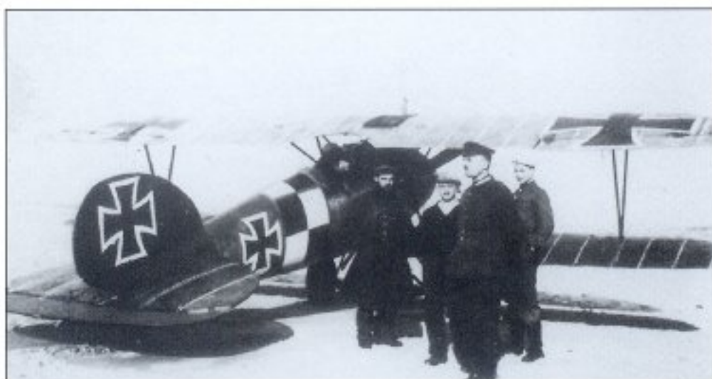
A useful rear view of Sachsenberg's Albatros D Va at MFJ I. This perspective illustrates the five-colour printed camouflage fabric on the wings and tailplane (J Rhyeuß)
