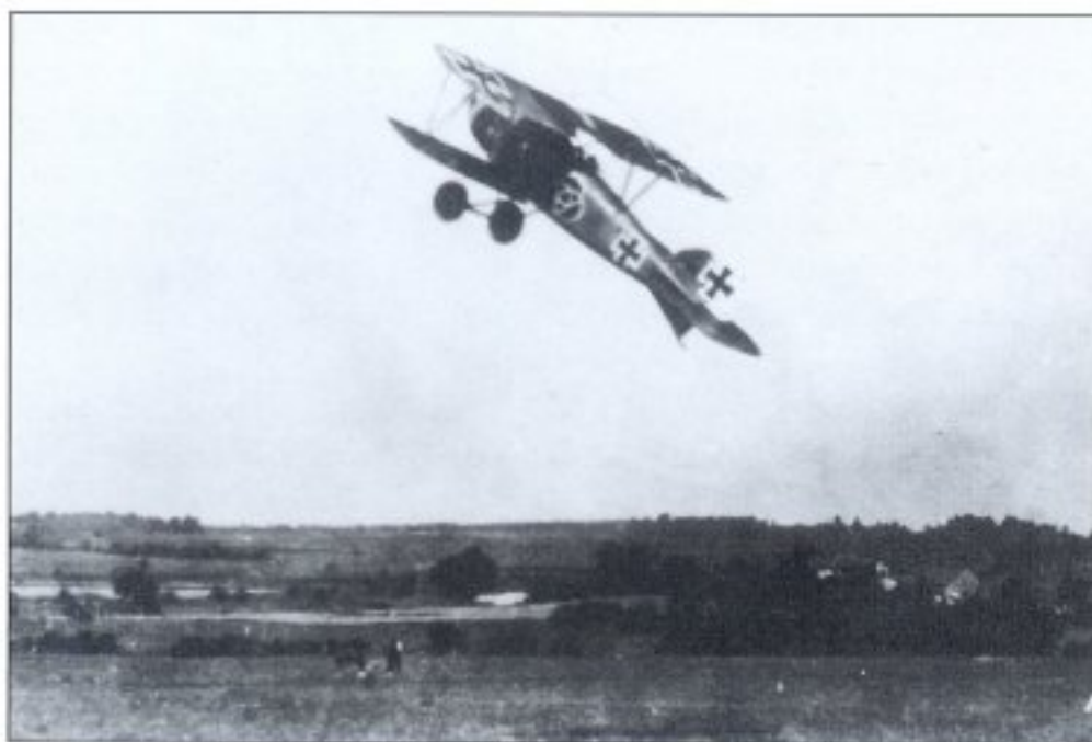
Altemeier's D III reaches for altitude on take-off. This aircraft was fitted with small lower wing braces attached to the bottom of the vee-struts to prevent the wing from twisting (HAC/UTD)
