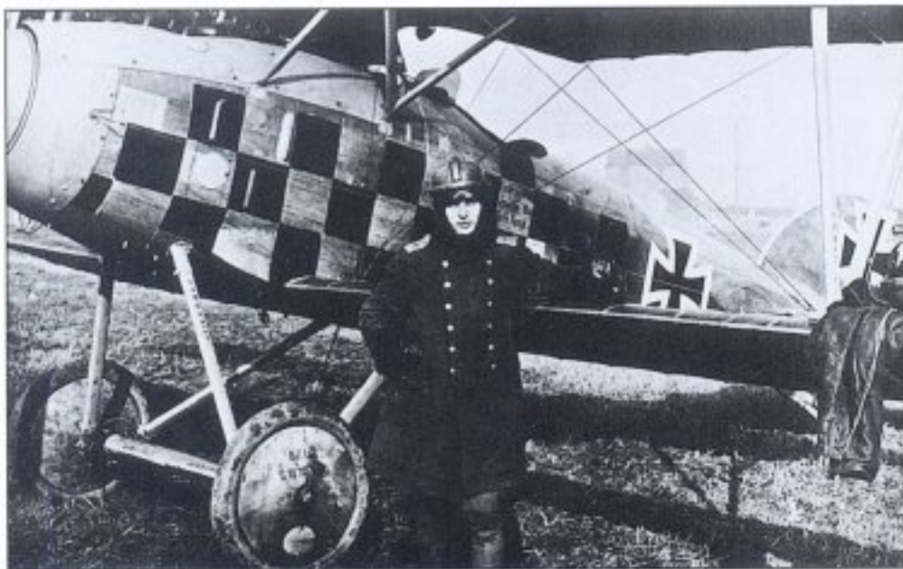
Jasta 49 pilot Ltnd R Hermann Habich poses with his Albatros D III (OAW) 5127/17. This unit was equipped with several OAW-built D IIIs, and Habich's was marked with a black chequerboard pattern painted on the varnished plywood nose. The struts display the legend OAW D 3 5127, but the port wheel cover must have been a replacement item from another aircraft, as it is marked as 5129 (P M Grosz)
