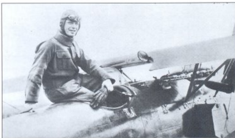
Ltn d R Herman Pfeifer sits on the decking of his Albatros D II in this postcard photograph – one of a series of publicity shots taken of successful Jasta 9 pilots. The bulky Windhoff radiator is quite evident on the fuselage side, and a mounting for a flare pistol can be seen on the right side of the cockpit
