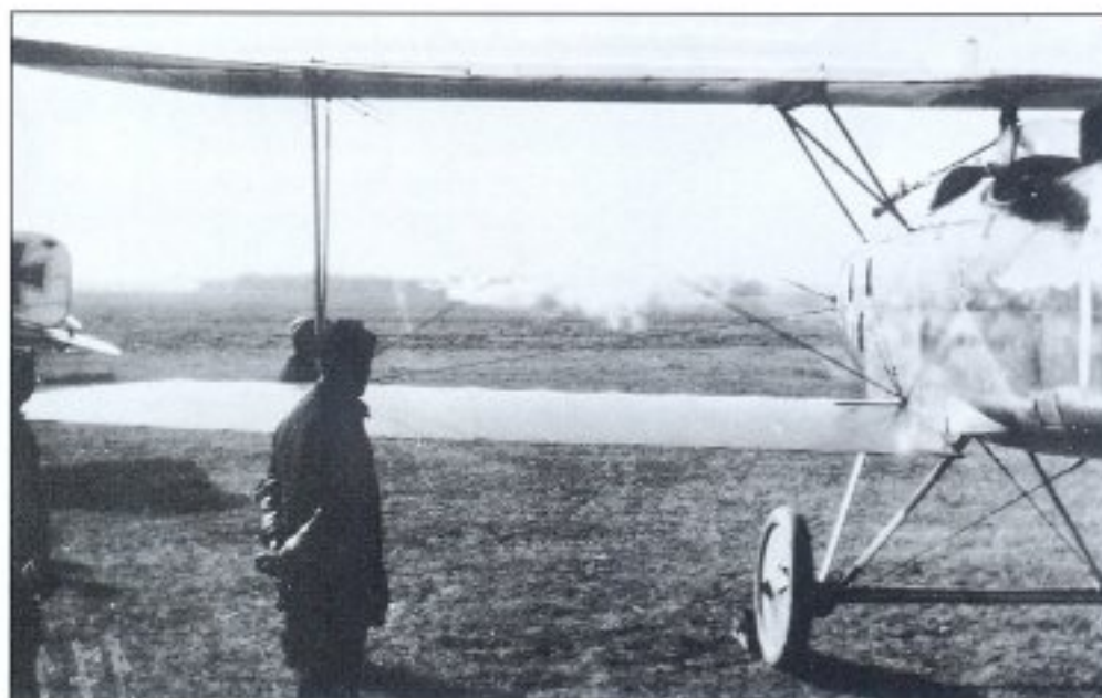
Berthold's D III of Jasta 14 is set up on the shooting stand as its guns are 'sighted in'. Again, the familiar winged sword emblem of the Staffelführer can just be discerned (HAC/UTD)
