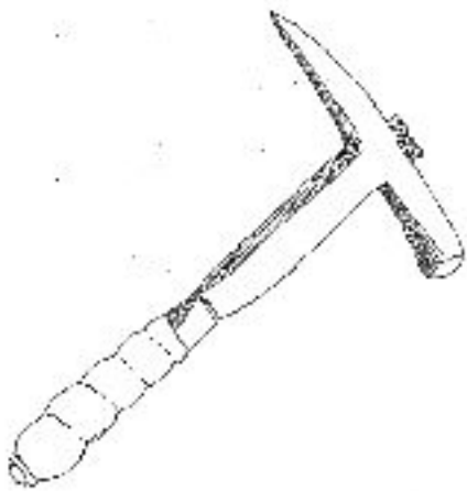
An Zax is one of many roofing tools. The point is used to punch through slate tiles.
