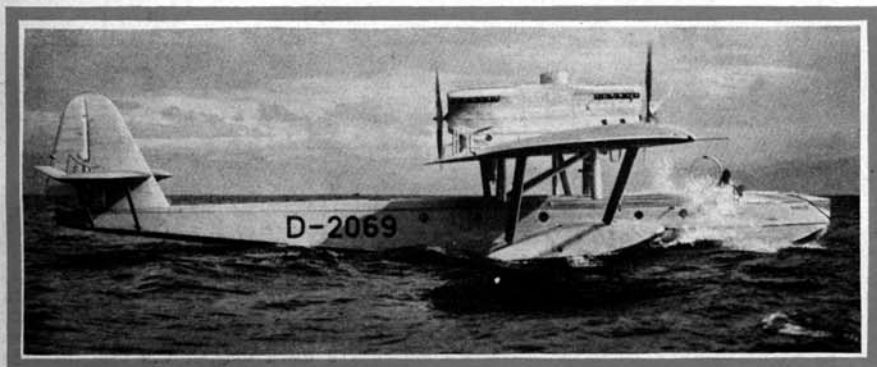
Great seaplanes of this type, will be used when the first regular flying service over the Atlantic is inaugurated. Note loop aerial on nose of craft for the radio compass that guides flyers
